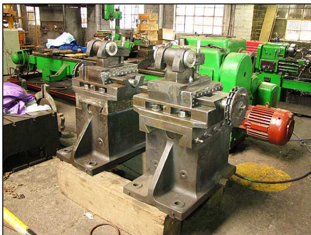
P13 - By the 2 nd of March the second tool tower (left) had been reassembled and the new grease nipples finished. The last fabrication work will be a pair of spoked wheels to be slipped over the square shanks of the traverser shafts.
