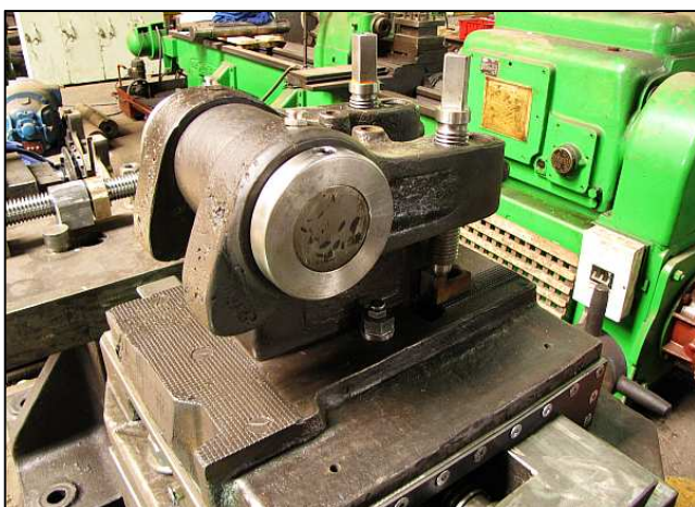
P09 - James has also been drilling, tapping and fitting new grease nipples in strategic locations. Although the tool stands were blatantly neglected, they weren't designed with easy lubrication in mind in the first place.
