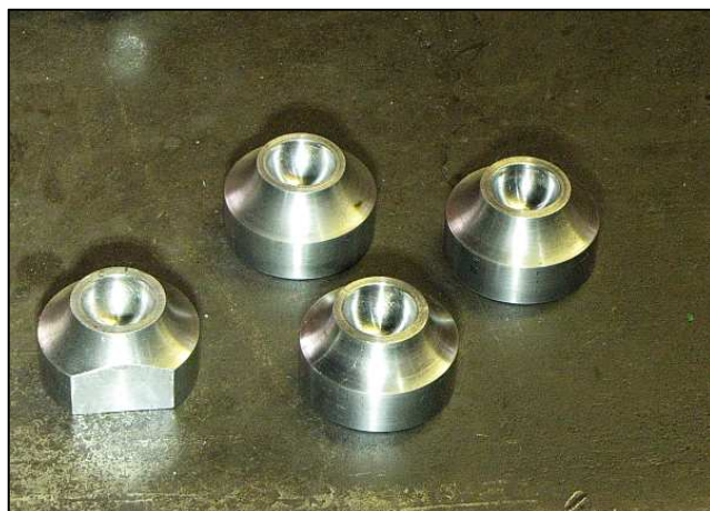
P18 - The leftmost pad has already had a 'flat' machined out as the diameter is too wide for installation. It was quite a sight to see that asymmetric shape whirling sideways in the lathe's chuck – but our James knows EXACTLY what he is doing!
