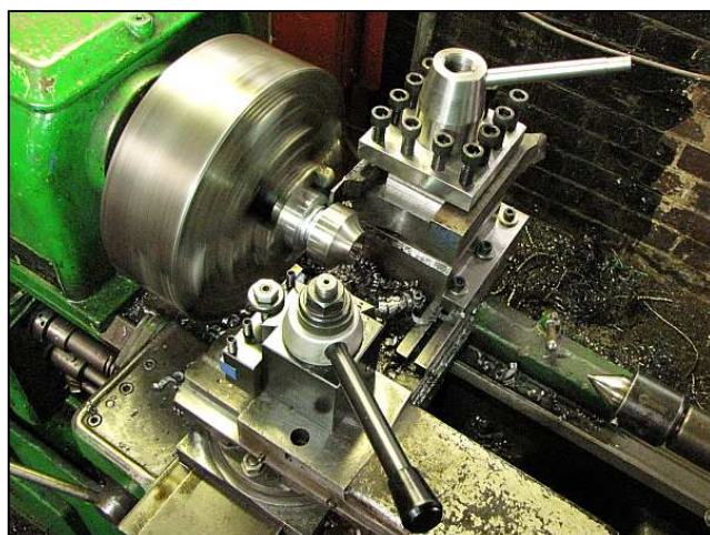
P16 - The jacking pads for the tangent bolts were originally machined double headed on circular stock. Here the two ends are being parted with a deep cut. The cut was too deep for the tool and had to be finished with a hack saw.
