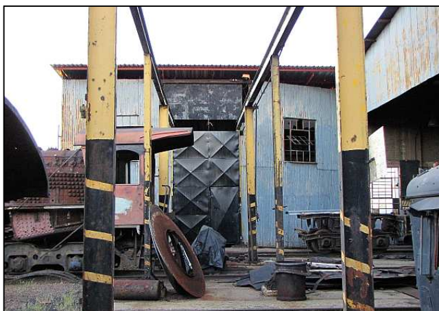
P21 - This view of the closed doors emphasises the original intended purpose of the gantry crane – to transfer locomotive axles to the wheel lathe for profile correction.
