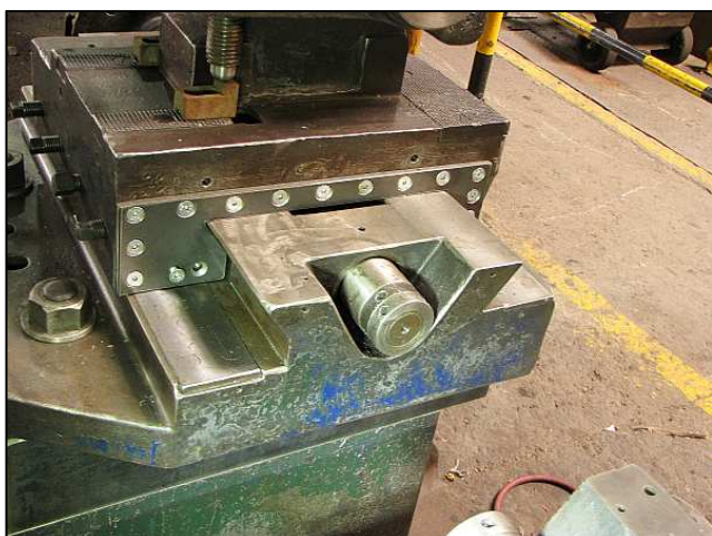
P15 - One of the new hard steel scraper plates in the process by being fitted – using countersunk allen key machine screws. Incidentally, you can also see that the tool carriers were once painted blue over a green base.
