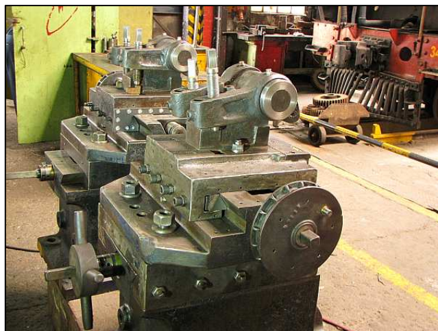
P14 - This view shows the adjustable tapered key that is used to adjust the clearances. The slides had to be machined. You will notice an extra spacer added behind the wedge. The spoked wheel is the last one surviving.
