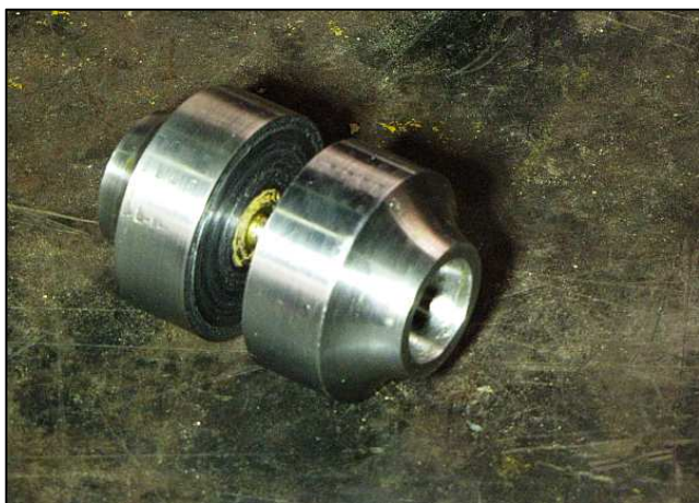
P17 - Looking like a weight lifting dumbbell, the assembly awaits final sawing to separate the two heads and then the bases to be re-machined flat again. You can see the hemispherical socket into which the tangent bolt will engage – almost like a pushrod into a tappet on an old car engine.
