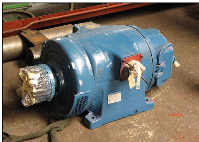
P22 - The rebuilt electric motor has since been relocated and is ready for installation.
