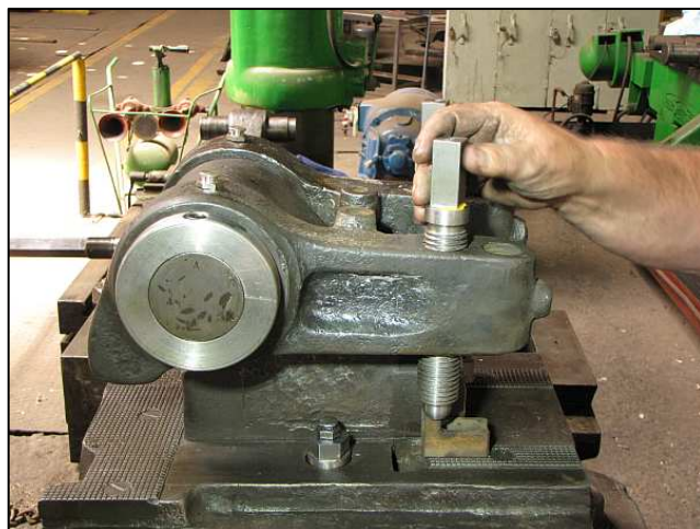
P08 - The pivoting tool heads have been refitted with brand new tangent bolts, which are used to tilt the actual cutting tools.
