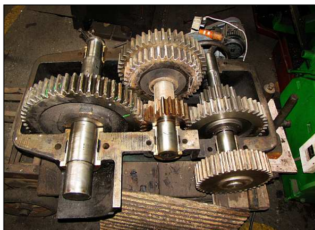
P10 - Both of the lathe's overhauled gearboxes have been test assembled and proven to be free-running in their new bearings. This, the tertiary gearbox, has had the existing worn bronze half-shell bearings all relined with Vesconite.
