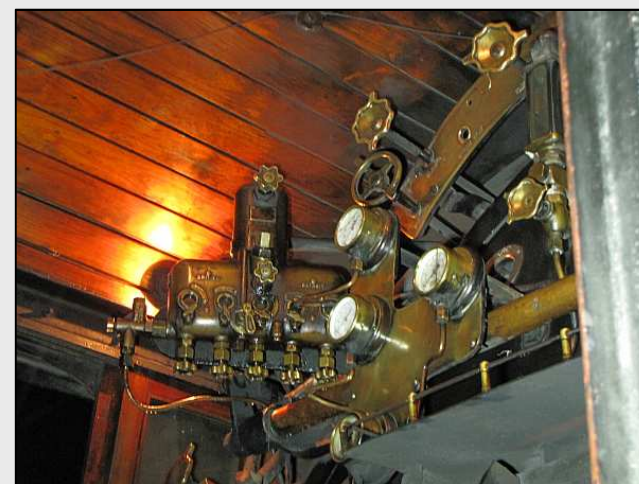
P14 – At least this one was fairly dry! This is the 'five-lung' Detroit lubricator for the 15F. It had already been serviced and the feed set to get the slippery stuff running through the oil lines prior to running. (We'd be taking off after a relatively quick shunt of picking up the two-part train.)
