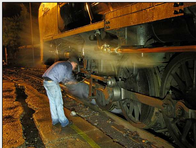
P10 – Seen greasing the eccentric pin on the Expansion Link, Shaun Ackerman was given the second slot, also in recognition of a substantial financial contribution and the work he put into the tour coaches. Shaun and Philipp constitute SAR Steam Tours Management and Organisers.
