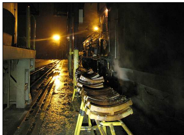
P08 – A diesel brake shoe rack. We are considering modifying or recasting some locomotive brake shoes to use replaceable composite friction liners, as we are running out of spare stock to use. The 15F chows her brake shoes.
