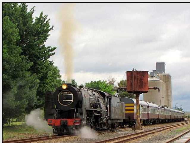
P22 – After some cell-phone interlocking with the pilot on the 12AR, Ackersmudge pulls the 15F away from the stationary sleeper train. The intent was to clear the front end to attach the goods for departure. Just look at that thin jet of sulphury yellow smoke – a tell-tale flag of poor coal.
