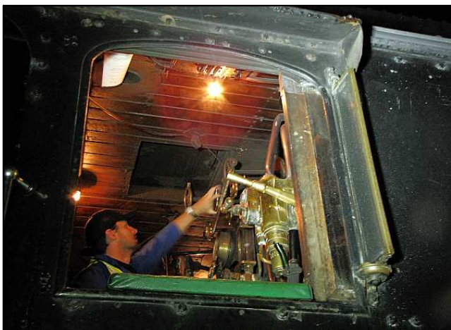
P05 – That is a Dawie opening the blower after laying some coal on a half-opened and partially-shaken fire. (Ash chute closed over the pits.) I didn't shake-up overnight for fear of waking the passengers. Apart from a jammed valve on the turret, needing spanner treatment, the 12AR woke up OK.
