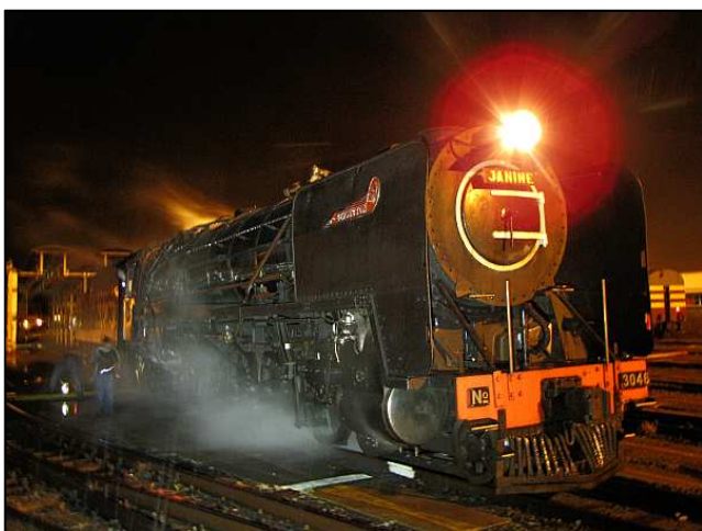
P13 – The thousands of lubrication points on a typical SAR locomotive are a right penance in the rain. The water also gets into the axle boxes, especially on the 12-Bucket. I was shielding my camera from the rain with my trademark sheep drover's hat, one of the reasons why I wear it!
