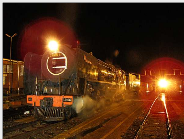
P02 – The Class 15F locomotive had the better fire in the morning, so she was moved out first. Although there was less clearance for ash drops, we didn't want to drop ash down into a wet diesel inspection pit. Fire cleaning was a only a cursory affair this morning though – more of a raking.
