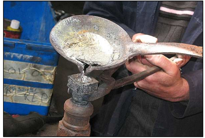
P122 - Before a locomotive is steam tested, the various fusible plugs in the firebox all need to be removed, stripped, cleaned and then their heads re-cast into a hemispherical mould with the correct grade of molten lead. This has to be done by a certified person and the individual plugs need to be date stamped and recorded in the locomotive's log book.
