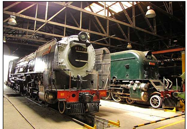
P118 - Challenge – Wheel Lathe. Both of these large locomotives, a Class 25NC and a GMA/M Garratt, are in operable condition. But they are not allowed on the main line due to wheel profile/flange wear. Between them, they have 44 wheels – with 12 driving axle sets that need to be removed to machine the wheels.
