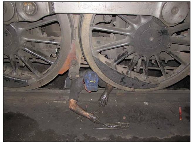
P112 - Work sometimes has to be performed between the frames and the wheels, which is usually a greasy job for the stout of heart and slim of build. Every bay on the 15M workshop has a work pit.
