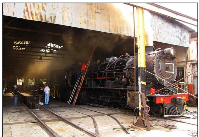
P102 - Although the Top Shed is usually used for locos in steam, the live steam boiler tests are usually performed in the 15M shed area. This is the 12AR undergoing boiler testing in March 2013 – she was still building up pressure at this point prior to setting the safety valves.
