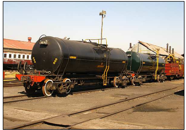
P094 - We have a small fleet of water tankers are our disposal, all of which need servicing. One of them has been especially lined as a drinking water tanker and one of them has a fitted fire-fighting pump. These tanks are required to extend the range of our thirsty steam locomotives on a railway that no longer has water supplies.
