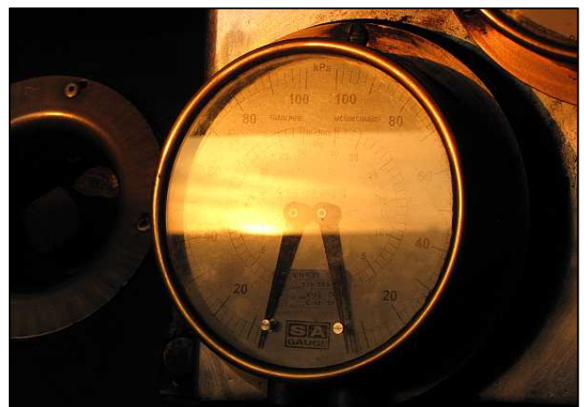
P126 - Not all locomotive work is brutal or dirty. The various relatively delicate pressure gauges, and the vacuum gauges for the brake system, have to be recalibrated and certified at regular intervals. Seen at sunrise on a tour is a classic duplex vacuum brake gauge.
