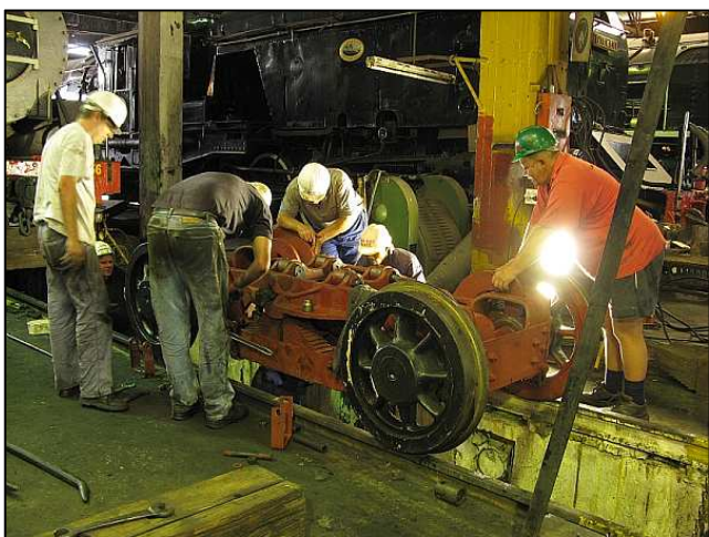
P113 - The depot gang can be seen overhauling the surprisingly complicated front bogie of a locomotive.
