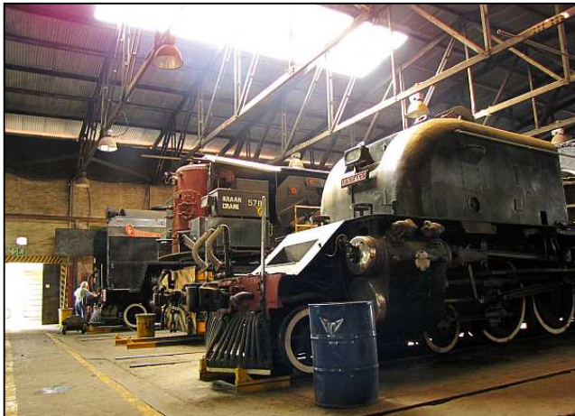
P087 - A variety of steam machines at rest, as they are waiting for other projects upon which they are dependent. The GMAM Garratt in the foreground and the Class 25NC at the rear are 100% intact but are waiting for the wheel lathe's completion to enable wheel profile correction.
