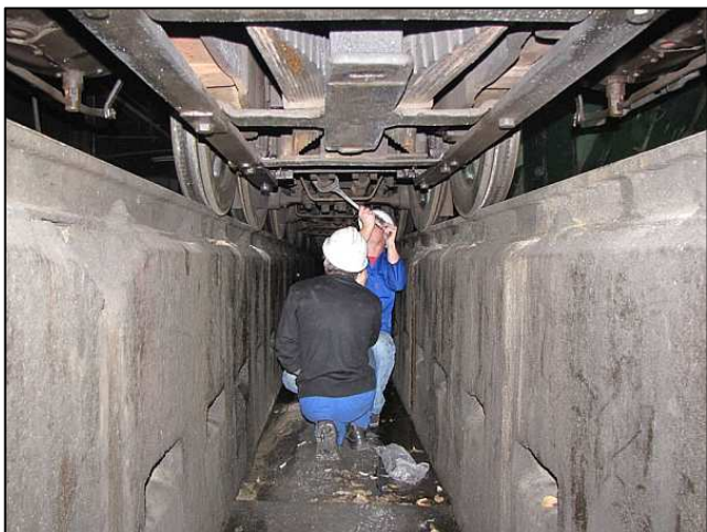
P143 - You get them underneath! Here, a locomotive's brake pull rods are being tightened up to eliminate excess clearance between the brake shoes and the wheels. This is a frequent task in preparing and road-worthying a locomotive for a day's run.
