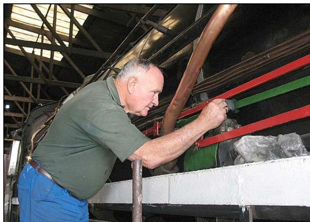
P148 - We usually have gentle work available for the old lads who are getting a bit creaky at their hinges. Oom Attie, currently South Africa's oldest certified steam driver at age 74, is seen quietly painting the green indicator rod for the powered-reversing gear and is staying out of mischief!
