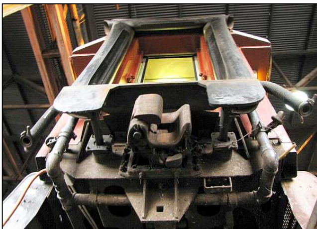
P089 - The 15M workshop's inspection pits come in useful for the servicing of the draft gear and buffer plates of the coaches, all of which need lubrication and checking at regular intervals.
