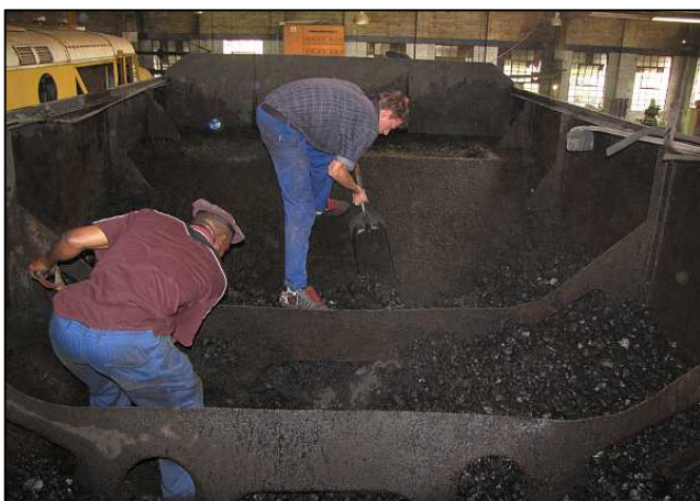
P125 - Unlike diesel which can be pumped with ease, coal has to be mechanically handled – one of the subtle reasons why steam traction is no longer used. Two members are 'trimming' unused coal forward in the Class 25NC's tender, so it can be reached from the cab to light up the fire.
