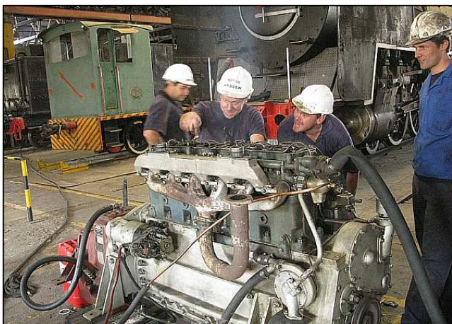
P147 - A certain grumpy Yorkshireman (Center) looks pleased for a change as the diesel shunter's engine is running as a bench-test on the second try. (The starter motor failed the first time round.) He is happily explaining the need to tighten up the valve clearances to the STEAM boys who aren't familiar with internal combustion engines.
