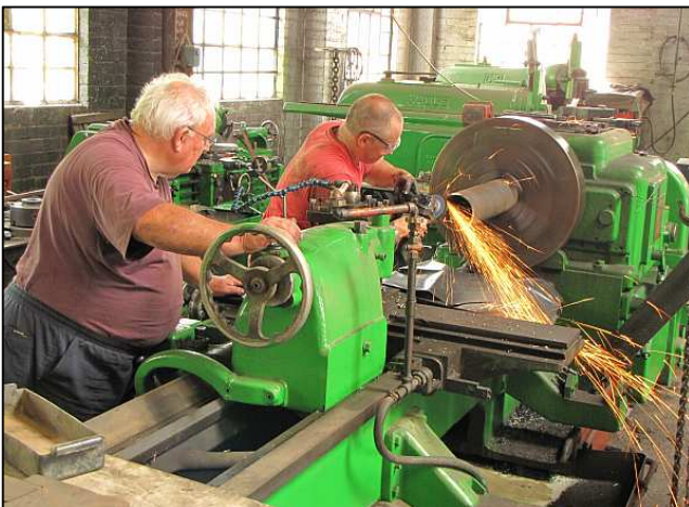
P107 - Making a plan. A genuine ex-Millsite Fitter is using a handheld angle grinder to dress the chamfers on a new steam downpipe being spun in the big Dean Smith lathe.
