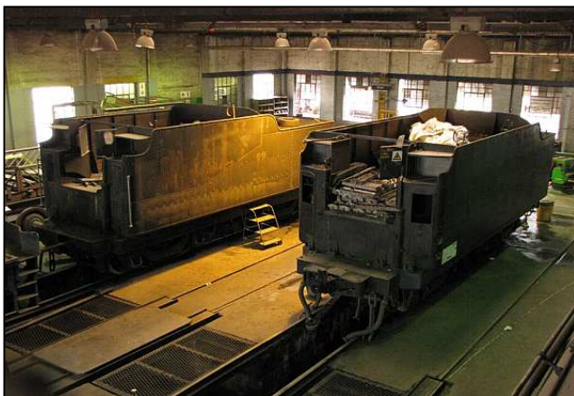
P095 - Tenders also need to be repaired. These two examples are waiting for their locomotives to be repaired first though! The tender in the foreground is for Class 15F No.2914 and it has a stack of removed fire grates sitting in the coal space. The tender is waiting for plate work and conversion of the axles to roller bearings.
