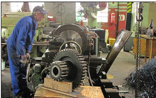
P119 - Challenge – Wheel Lathe. New gear blanks are seen in the process of being machined for the restoration of our wheel lathe, and by a genuine ex-railways machinist too! They were sent away for the cutting of the actual gear teeth. As of Feb 2014, the new gears have all been cut.
