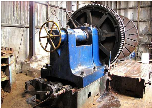
P117 - Challenge – Wheel Lathe. We are in the process of restoring this mighty machine which is able to clamp multiple ton locomotive axles and re-machine the wheel profiles. Not only would we be able to machine our own equipment, but can also take on paying work from other railway and industry-related bodies to earn revenue.
