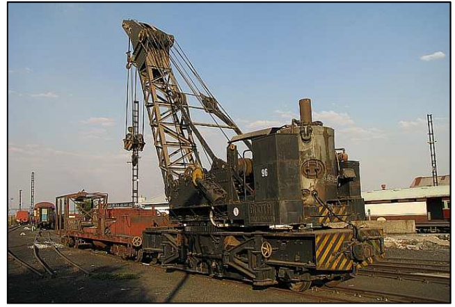
P092 - We have an intact Booth Rodley Steam Crane waiting for a replacement boiler to be fitted. No.96 'Shosholoza' was last used in 2008 to clear some scrap and move wagons from the boiler washout area– the uncertified boiler was then charging on compressed air.
