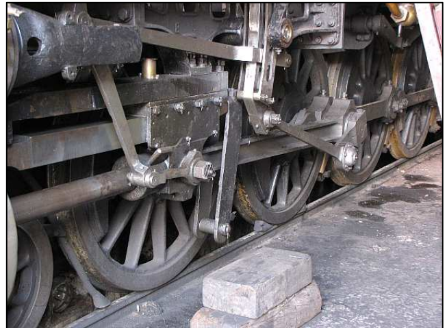
P106 - Reefsteamers is a pioneer in using Vesconite bushes in steam locomotive rodding, even when the railways said it would not work. Vesconite is a synthetic self-lubricating material that is tolerant of dry running. It has been so successful that it is now the Reefsteamers standard to replace all valve gear bushes with Vesconite when the original bronze bushes become worn.
