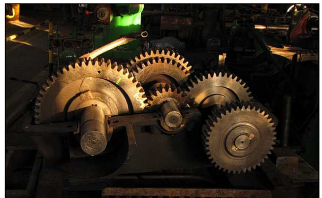
P120 - Challenge - Looking like a giant clockwork toy, the components of the wheel lathe’s tertiary gearbox are in place in their inverted housing. The gears had been newly made and the bearings relined, so the whole lot was test-assembled to check for free running. It would need to be stripped again to send the gears for case hardening.
