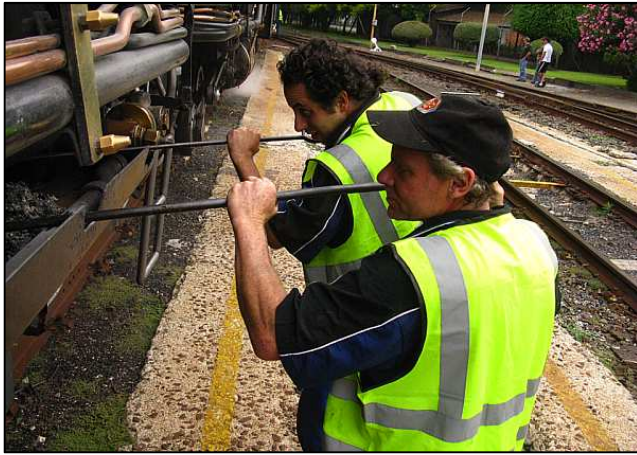
P133 - It takes teamwork to keep these often cantankerous machines going. Two of our Reefsteamers are incidentally moving in perfect synchronization as they strive to break up a HUGE chunk of clinker blocking the 25NC's ash pan.
