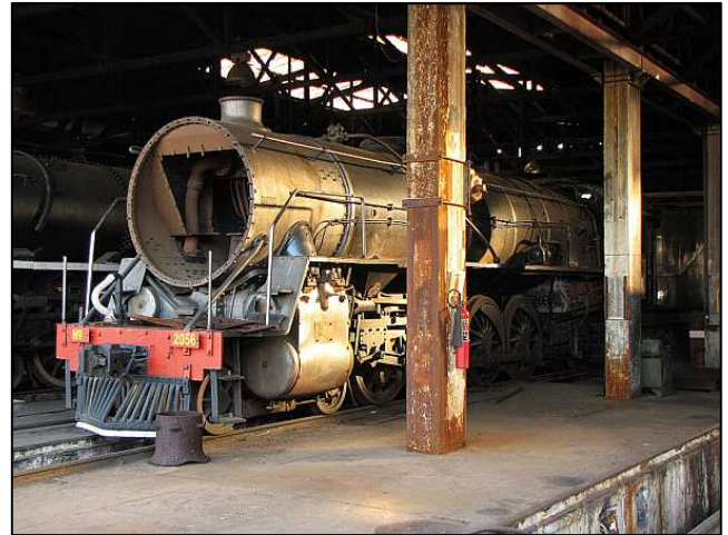
P086 - Some otherwise intact locomotives are sleeping in the 15M Workshop due to the expense of the repairs needed. This is our Class 15CA No.2056, which needs a full set of new boiler flues at approaching R450 000.
