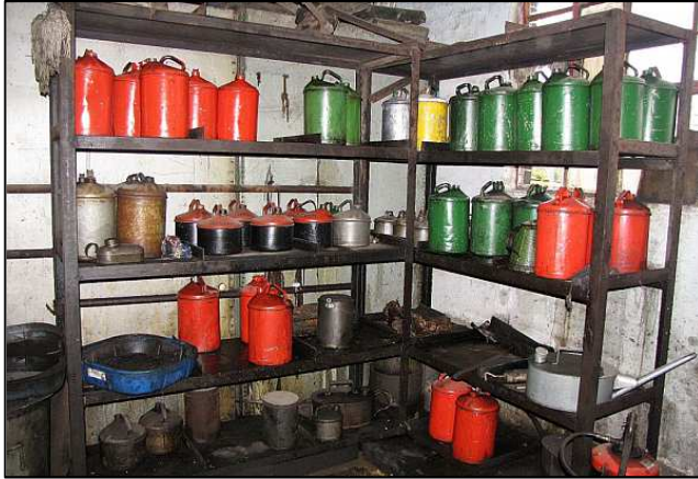
P115 - Challenge – Lubrication. Steam locomotive require quite a variety of expensive greases and oils to operate. This is a view of the oil racks with MH Oil (Red), Steam Oil (Green) and the shorter paraffin cans. The steam cylinder oil is actually tallow-based and has to be pre-ordered.
