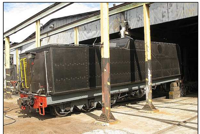
P096 - Occasionally the jacks and blocks come out – this is the rebuilt type EW tender of Dave Shepherd's Class 15F No.3052, which was treated to new decking, rebuilt bogies, rebuilt brakes and a rebuilt mechanical stoker, as well as new bracing within the coal bunker.
