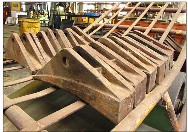
P124 - There is no such thing as popping down to your local Midas franchise to buy spare parts for your locomotive! Parts have to be scrounged, repaired, modified or re-made to fit. This is a trolley load of spare cast iron brake shoes intended for a Class 24 locomotive – some of which would be modified to fit the GMA/M Garratt.
