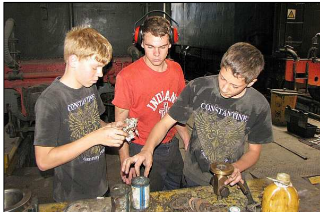
P152 - The younger people are allowed to do the less critical work on the locomotives too, obviously under supervision. The youngsters to the left and right of Jeandre are using grinding paste to lap in the brass sealing olives for water gauge cocks. Jeandre (center) is a full time staff member and is a 21 st Century Apprentice Steam Fitter.
