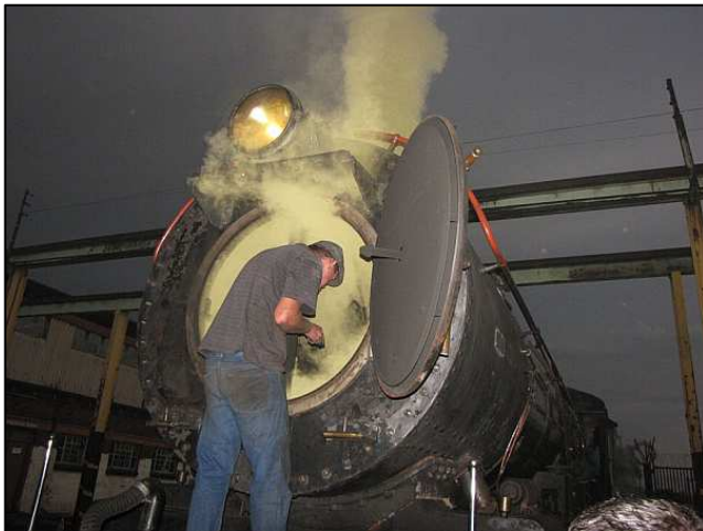
P135 - Things don't always go right! This 12AR locomotive had just undergone a steam test but the blower was not working, and thus the fire couldn't be drawn-up bright. We are treated to an unusual view of a smokebox door being opened on a live boiler while the fault is being looked for. (It was simply a flange that hadn't been bolted properly.)
