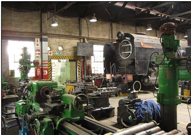
P067 - The main machine shop of the 15M shed survived from the old days, with just the loss of a large vertical boring mill before the stripping and scrapping was officially stopped there. Our locomotives can thus be repaired with some of the same machinery with which they were repaired in railways service.
