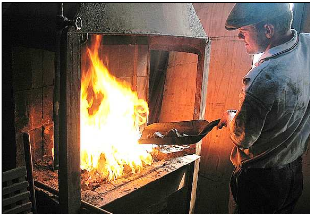
P075 - Although the original Forge Workshop was lost to scrap when the Depot first closed, there is still a working coal-burning forge in our Running Shed. More than just a 'braai', it is lined with refractory bricks and has a compressed air supply. Here, it is being stoked to heat up and soften large-bore copper piping for ease of bending.
