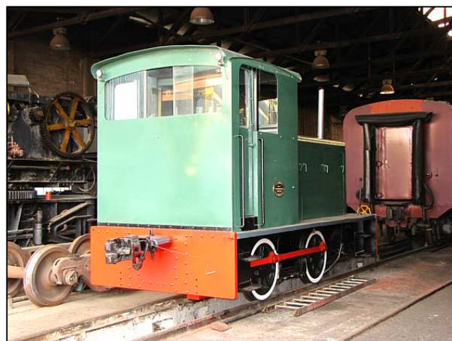
P066 - This tough little shunter has been named 'Andrew', after a certain equally-tough little Yorkshireman. He looks great in a fresh paint job after an engine and gearbox overhaul.
