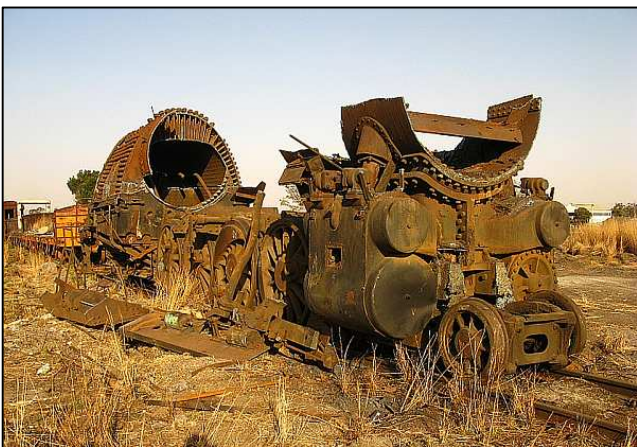
P011 - Two weeks later, the same locomotive, Class 15F No.3020, had been viciously disembowelled, having lost the boiler, cab, smokebox, buffers and the running boards. No matter how derelict the locomotive was, it is always sad to see one of these brave old machines finally go down.
