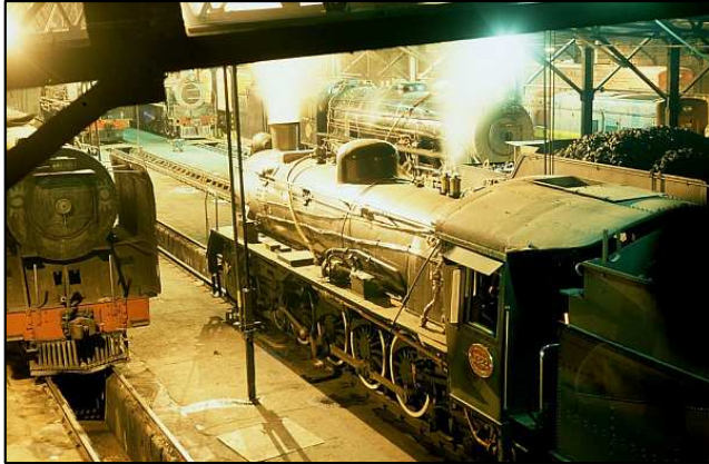
P007 - The diesels began to move into steam's territory from 1987 – you can see them on specially raised servicing tracks at the rear of this picture. The use of steam traction was terminated here in late 1992. But the mechanically and electrically more complex diesels do not thrive in a steam environment and they were soon moved out anyway.
