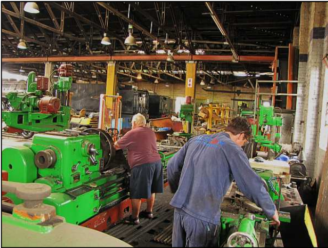
P073 - A view from the corner of the machine shop. Reefsteamers has three lathes of which two are operable. The big lathe was donated to us and is an 8-ton Dean Smith unit. We have plans to raise the check and tail stock by about 4 inches to increase the lathe's capacity.
