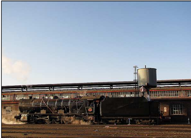
P031 - Although the old water tower is fully functional, we prefer to fill our tenders with hose pipes and keep the water stored in the tower as an emergency reserve. On special occasions or when a speedy refill is vital, we still top up our tenders from the tower in the good old fashioned way.
