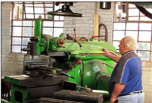
P071 - This Thule reciprocating shaper is being used to cut a perfectly straight edge onto a battered steel plate. We have two of these machines, most often used for machining items such as planar bearings and crosshead slides.
