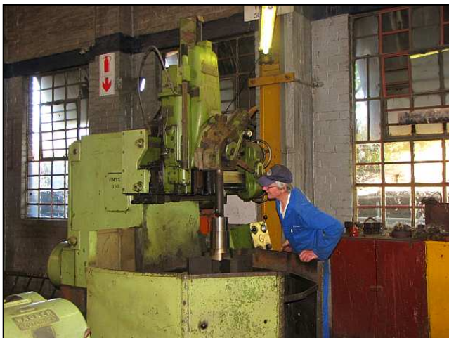
P069 - This is the surviving vertical boring mill, which is still fully functional. This is considered to be a medium sized machine and we have used it to machine brand new bronze bushes for our engines. (Amongst other items.)
