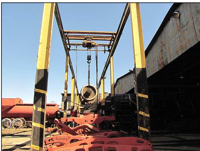
P083 - Here is an end view of the pneumatic gantry crane fulfilling a role very close to its original purpose. It is seen being used to traverse an axle for the Class 25NC's tender. The rails on the crane are recycled light-weight rails that were originally rolled in 1885 – predating the depot itself.
