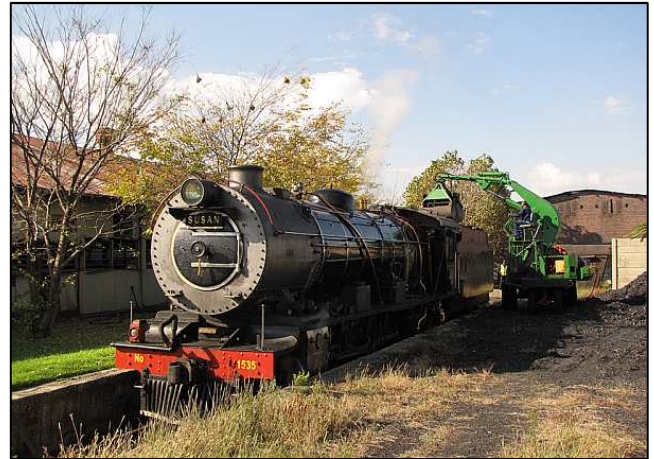
P032 - With the loss of the original elevated coal stage (Pic 008), Reefsteamers had to adapt an existing goods loading platform into a simple coaling dock. Here, the Class 12AR's tender is being filled with coal using the electric powered self-propelled 'Yumbo' grab.
