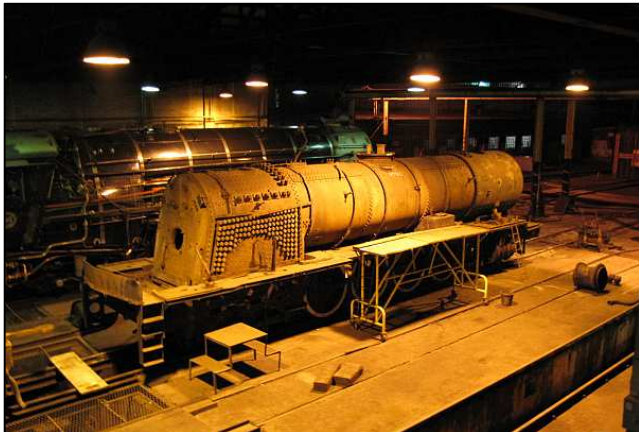
P051 - This is what Rosie looks like today. She has been completely stripped down to be made ready for a thorough sand blasting. Once cleaned, the boiler plates will be X-rayed and thickness tested for assessment for restoration. Years of being parked in the weather has caused local rust pitting in the boiler. She might never run again if the boiler turns out to be unusable – but she is safe for now.
