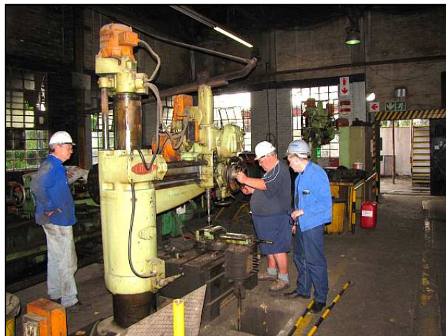
P070 - The two radial arm drills are fully functional. This one has a lower table and a recess pit placed so that long objects like shafts can protrude into the ground.
