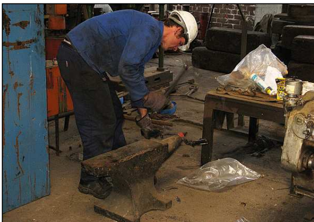
P077 - We have a couple of anvils to go with the forges. Here the reversing lever belonging to prestige Class 15F No.3052 'Avril' is being heated and straightened before having its Johnson Bar style ratchet rods fitted.
