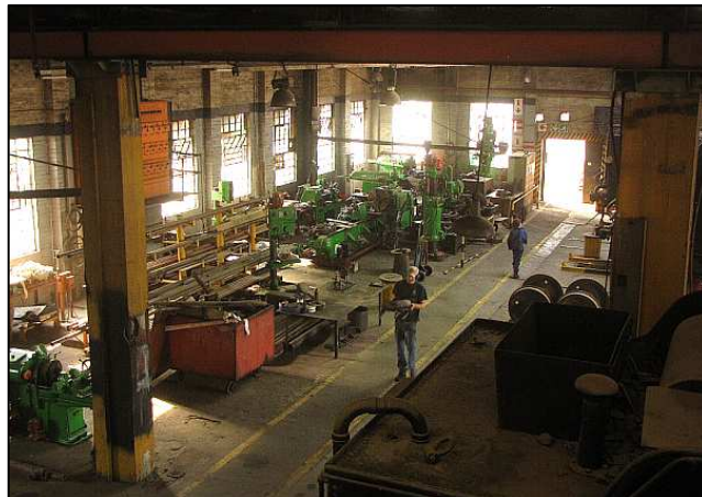
P068 - The surviving workshop is a major asset for Reefsteamers. Most of the machines that survived were in worn condition and with the electrical power disconnected. We are gradually restoring them all to operation and also bringing in surviving machines from other areas of the depot for convenience of access and wiring.
