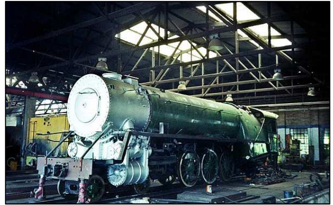
P056 - The loco from the left, Class 15F No.3046, was the first locomotive officially allocated to Reefsteamers for restoration in the now-preserved 15M workshops. It was quite a major project for such a new group to take on!
