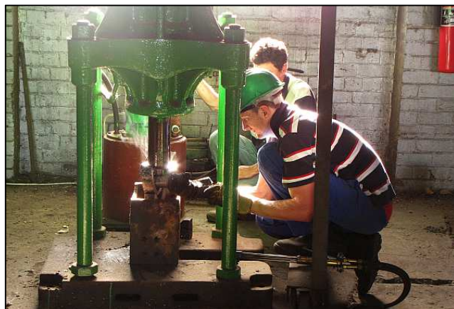
P072 - One of two hydraulic presses is being used to press a steel bar 3/4 inch thick to form a drilling jig. This is the 'small' package press intended for drive wheel coupling rod work. The bigger one can exert a pressure of 50 tons.
