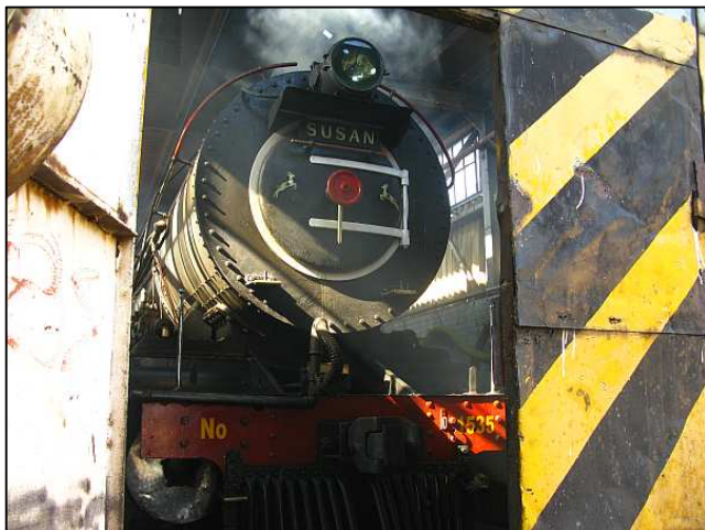
P01 - A bit closer to the ground now that the bogie has been re-installed, the 12AR No.1535 steams up behind the still-closed gates. As we had two blowers on the compressor, the draft was a bit diluted and the steam-up took a while.
