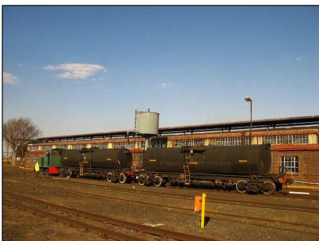
P19 - This unusual move was to fill up a tanker for each the two locomotives that we planned to run the following day. They were parked in fire hose reach opposite a water bowser, rather than being shunted for the water tower.
