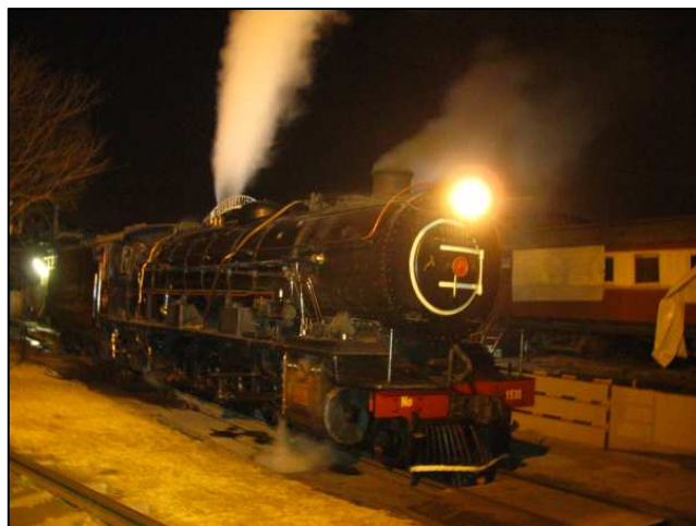
P36 - In spite of Simon deliberately 'capping' the hot boiler by running the left injector to spray down the cab and backhead BEFORE cleaning the fire, she still popped-off. Obviously excited to be in steam once more.
