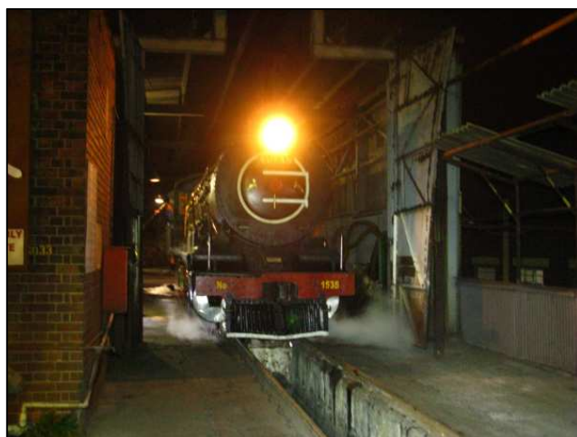
P32 - The 12-bucket finally moved out at about 6:30 after an extended time of standing and blowing through the open cocks to warm up the winter-chilled cylinders.
