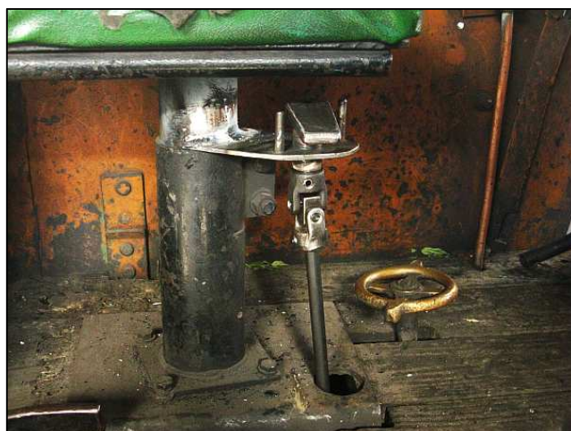
P08 - This is a side view of the new extended injector water kick-lever, (Fireman's Side) which is now hand-operated. The pedestal plate will be painted black in a week or two. The lever originally protruded from the hole in the floor.
