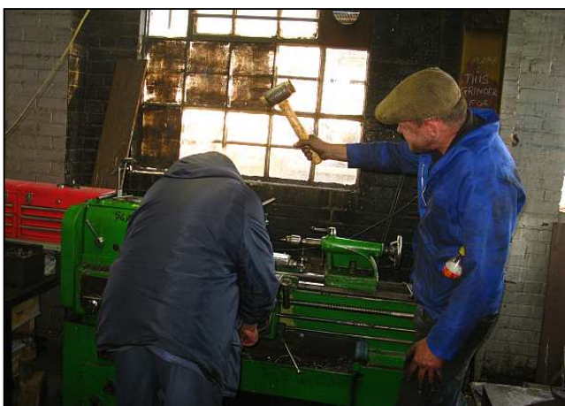
P13 - A new pressure gauge was fitted to the 12AR, but it first needed a matching ferrule on the small bore piping. Shaun ponders whether bopping dear old James on the noggin (with a hide-faced mallet) will increase production.
