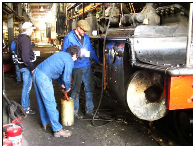
P12 - Susie the 12AR was treated to extra oil. The slide bars are being 'sauced' after the bogie boxes had been topped up. The bogie crown boxes, like any wick system, deliver oil continuously and this one would run overnight.
