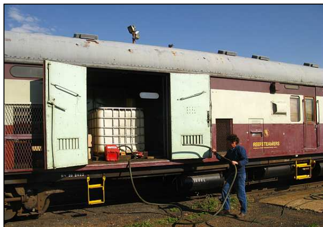
P18 - Captain Curly is doing a similar operation to top up the generator diesel fuel tank in the S&B van. With young Jeandre being busy and away at the SANRASM closure project, a lot of his usual weekday loco and train preparation tasks needed to be done by the weekend volunteers.
