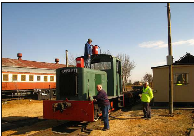
P17 - Sans fuel gauge or sight glass, 'Andrew' the Hunslet tends to be run until he croaks. They caught the level in time. Big Bennett is siphoning diesel into the bulkhead tank while Driver Attie (L) and Shunter Cliffie (R) wait for their steel pony to be 'water' before starting the day's shunting.
