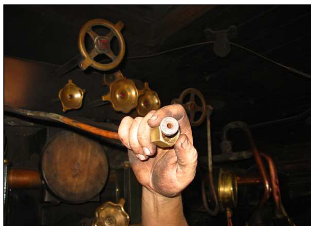
P14 - Seen after the pipe had been threaded through the cab's spectacle plate, this is the new ferrule that was machined out and then brazed onto the copper piping. Ten points for remembering to put the nut on before brazing!
