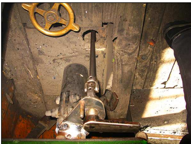
P09 - This is what the fireman would see if he looks down between his knees. ('Off' position.) The lever can now be operated with the stronger, more coordinated right hand. This new arrangement is gonna be great for the guys with big feet that battle with the original floor-mounted levers.
