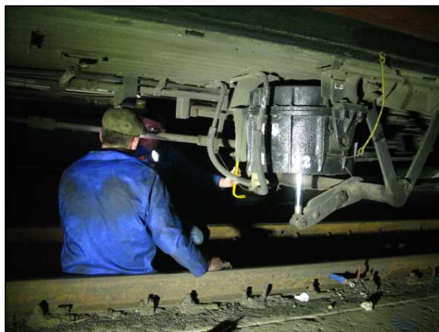
P46 - While we had a vacuum-braked steam loco hooked on the train, we took the opportunity to do a quick (and cold) check of the brakes, although the official vacuum test would still be done in the morning. Gordon is using a mini-crow bar to tighten up the adjustable main pull rod under a coach.
