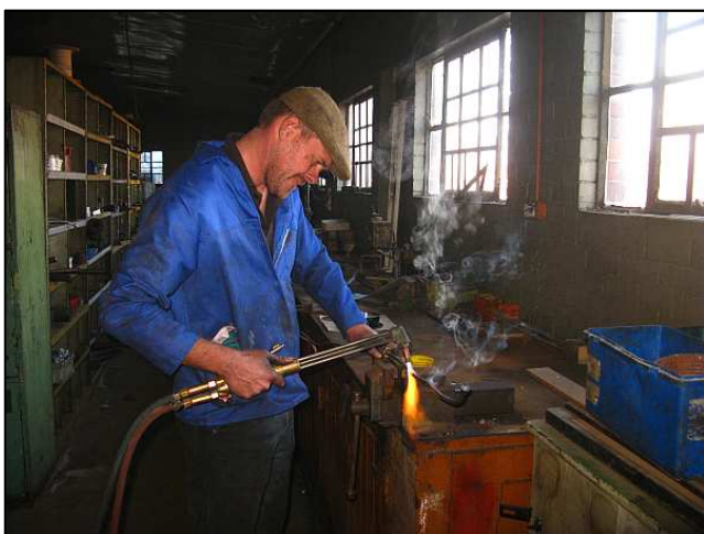
P15 - The copper piping needed to be annealed once it had been removed, to avoid it fracturing when being manually bent into place again. Simply put, annealing is the process of heating to glow and then cooling. Copper can either be slow-cooled in air or salt or fast-cooled by water, brine or oil. Water is naturally the cleanest method for fast quenching.
