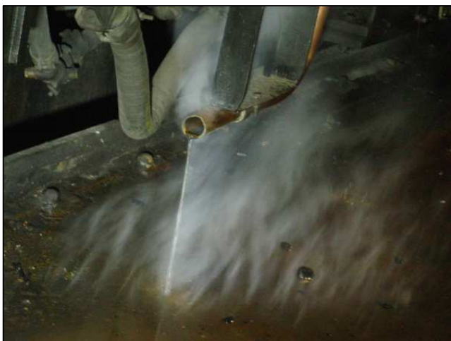
P11 - As seen on the 15F locomotive later that night, this is the constant dribble that we are trying to eliminate. This looks artistic and is a part of the 'living ambiviance' that a steam locomotive has – but it is wasteful of resources.
