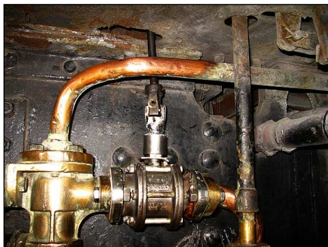
P10 - This is the new valve at the other end of the shaft. It operates with a smooth positive action but does need some strength to operate. Apart from reducing distraction for the Fireman, we estimate a saving of eliminating about 4500 litres of 'dribble water' from the overflows in a typical day.
