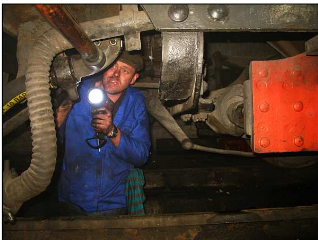
P29 - Smudge wisely did an early road-worthy on the 12AR. Here he is under the cab and using a flashlight to re-check the tightness of the bi-eared collars for the recently fitted water transfer hoses, and then the ballpeen on the elbow bolts.
