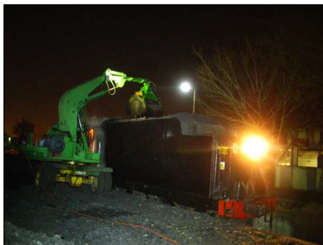
P40 - The first part of the coal loading process. Proceedings were later interrupted by the grab going dead – luckily with the scoop higher than the tender so the loco could still get out. It turned out to be a loose line connector.
