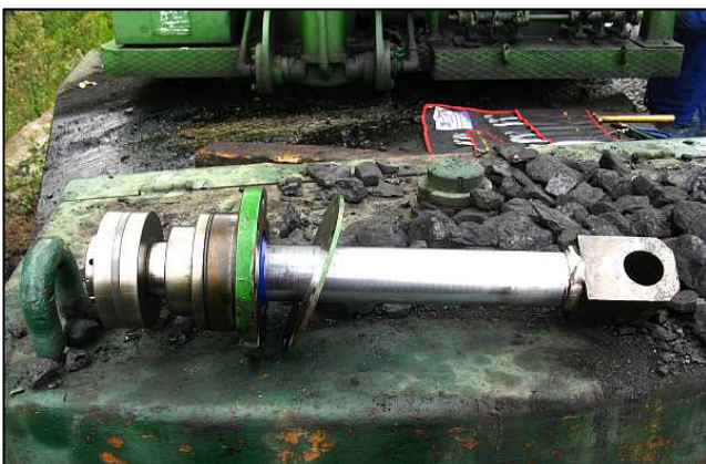
P11 - Here is the serviced and reassembled clam-shell actuator rod, piston and cover gear. The new bright blue seal is the wiper seal over the actual hydraulic pressure seal, while the disk plate is the scraper for bigger stuff.
