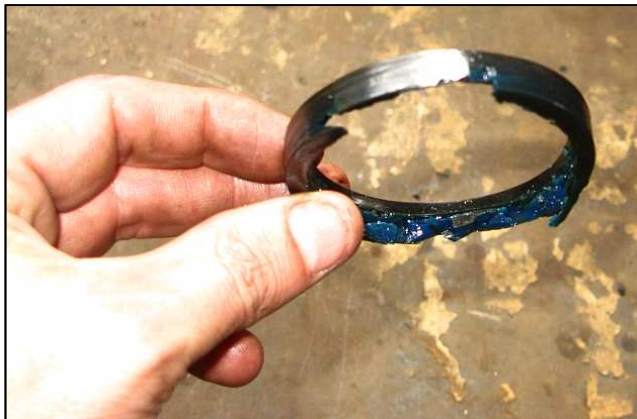
P09 - The hard steel disk scraper plate had been loosely fitted over the end cap and it was too bent to be of much use. This worn wiper seal shows the results of the constant ingress of abrasive coal grit at the dirty end of the machine!
