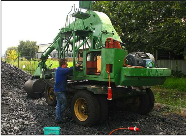
P07 - Simon is seen remounting the hydraulic valves. You will notice that the Yumbo grab is electrically powered via an extension cord. It was originally built as a diesel powered machine and used the Perkins engine that now drives the light-service generator in the S&B Van.
