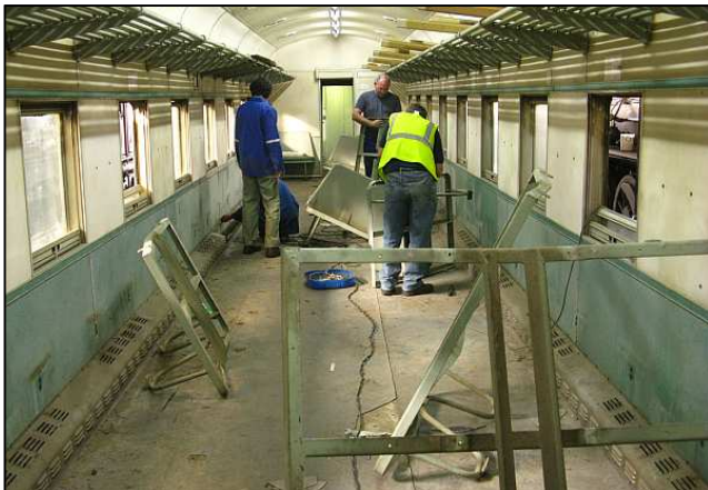
P21 - The passenger cabin is almost clear by 4pm. We have approx. 100 retired aircraft seats stored on our behalf at Rand Central and are discussing the fitting of this coach with those seats for better comfort than the existing. If it doesn't work out, we will work out a padded solution – but we don't want to turn out another 'hard back' coach.
