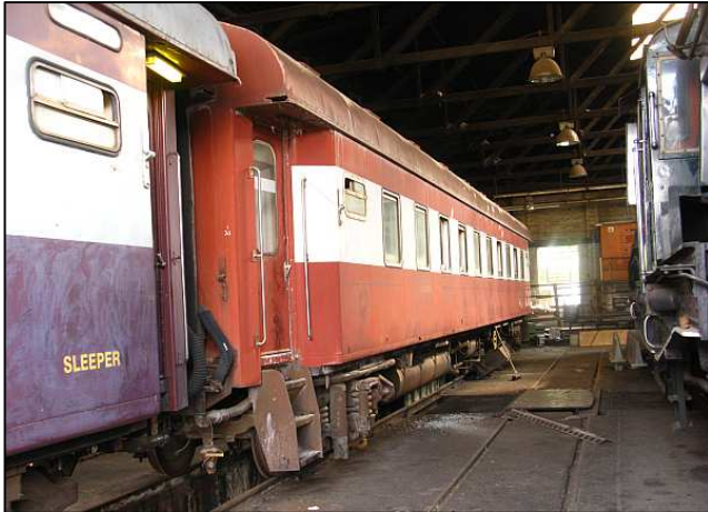
P13 - Work continued on 'Dusty' the Semuma Coach. The contrast in the paint colours is interesting to see, and Dusty still wears the old style oxide red roof. There are so many holes to patch, the coach will likely need to be resprayed.
