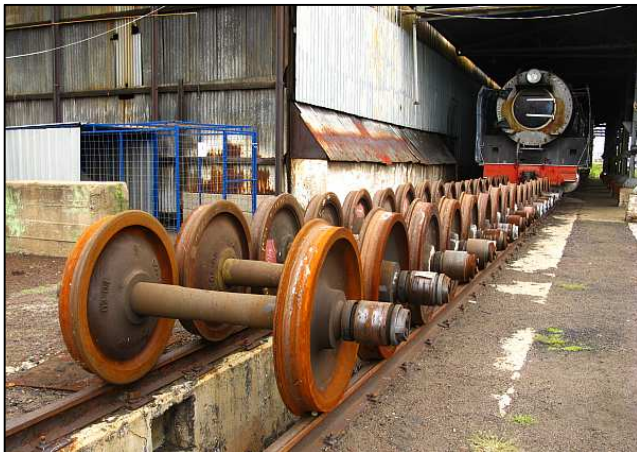
P09 - The axle stock for Shongololo Express's long distance coaches were moved over to the inner track of the old washout shed – lined up neatly in front of FotR's Class 25NC 3404 'Elsabe.' The recent blue structure in the background is the Security Forces' dog cage.
