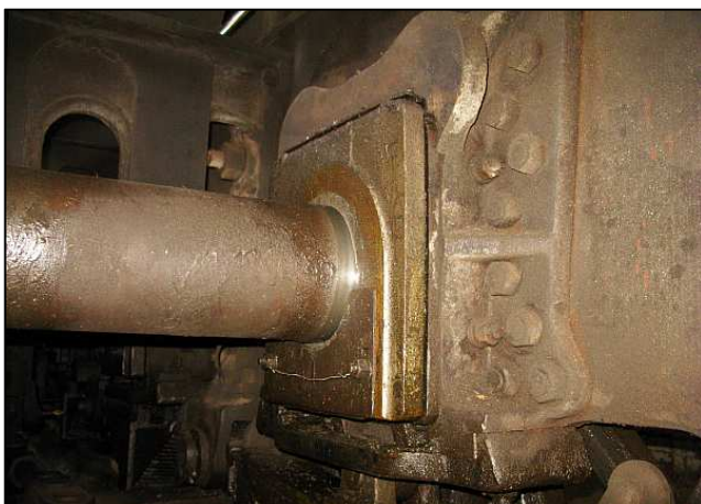
P05 - Here is an axle box, with the correct safing wire. The 12AR's axle wedges need regular checking as this small-wheeled locomotive is prone to knocking her axle boxes loose (fore and aft movement) if the locomotive driver isn't handling the cut-off properly or is a bit too speedy.
