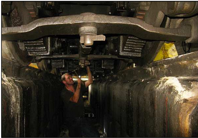
P03 - After the compensating beam was attended to, Susan the 12AR got an extra early underside inspection, including checking the clearance on the brakes (routine) and tapping for loose fittings. You can see a cotter pin (US terminology) in the foreground – which functions like a wedging split pin.
