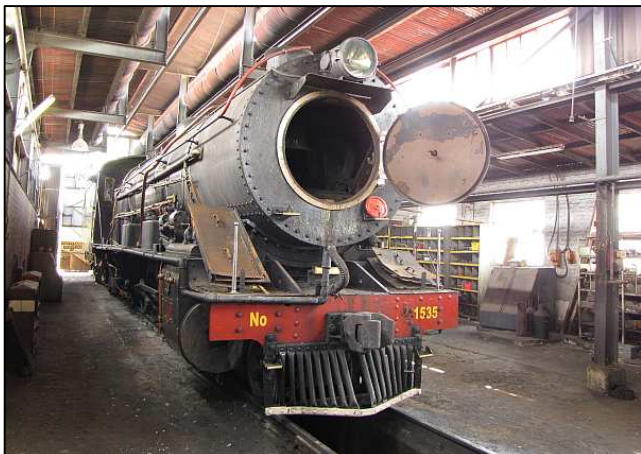
P01 - Suzie-girl has just had her first boiler washout out for the year and the door was left open to draw the air through for drying. Jeandre was tasked to check the baffles, table plate, blast basket, petticoat and washout plugs as well.
