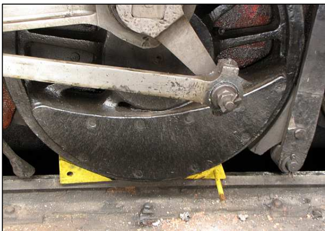
P03 - Properly scotched on both sides of the main driver axle as per our current standard. This is now a mandatory requirement for all standing locomotives at Reefsteamers, even if the tracks on which they stand is supposedly 'flat' and including all stock parked in the Top Shed and 15M shop.
