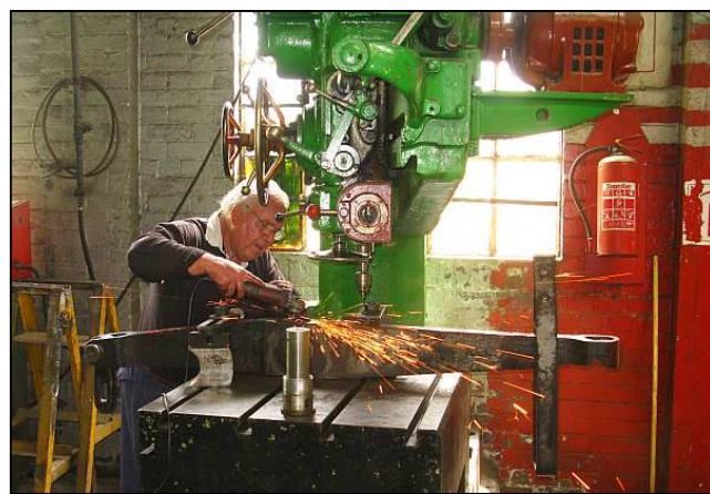
P10 - The dirty and battered surfaces were causing the drill bit to chatter and snag. James had some extra grinding and chamfering to do before the drill would run true while entering the oil passage.
