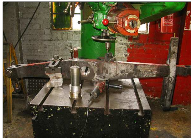
P08 - The looped safety strap (R) could not be removed without bending it or cutting it away. So it got to hang around and 'come along for the ride!' In the foreground, you can see both new and old pivot bearings on the pin.
