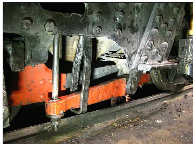
P12 - The finished beam as refitted on 21 March 2014. Although the link to the stirrup rod is actually a closed oval eye, it is still often called a 'camel's paw' by the old boys. It is filled with oil-soaked steel wool to retain oil for the indexed washer beneath. (A system we want to update!)
