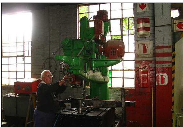
P09 - Using the big Asquith-built radial drill, James cleaned and enlarged the oiling hole, which was full of gunk. It had previously been roughly drilled out oversized, so a standard grease nipple would not fit without a lot of extra work.
