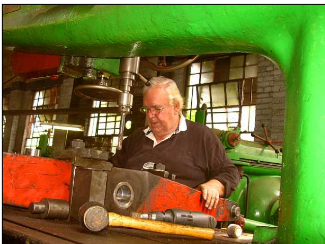
P11 - Framed by his big green rig, a happy James was starting to puff a bit from reaching over his head to operate the tall machine. He started out with an auto-feed setting but then switched to manual for fear of breaking the drills.
