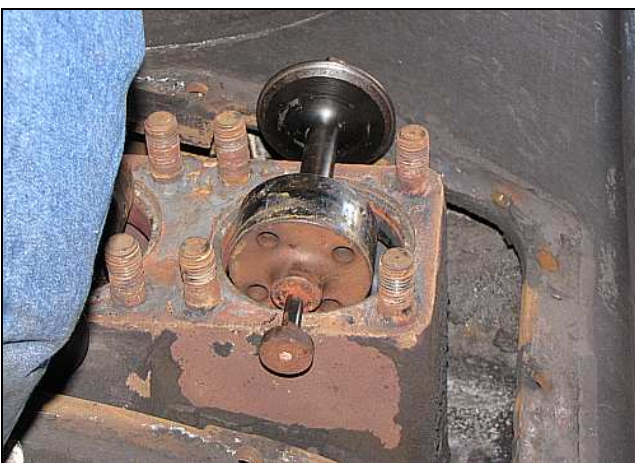
F11 – One of the double-beat valve spools of the regulator waits between its studs. As per Dawie with the clack valves, Aidan was lightly grinding the valves in and then sealing them with silicone for the hydro-tests. The silicone will blow out when the regulator is first used on a live boiler.
