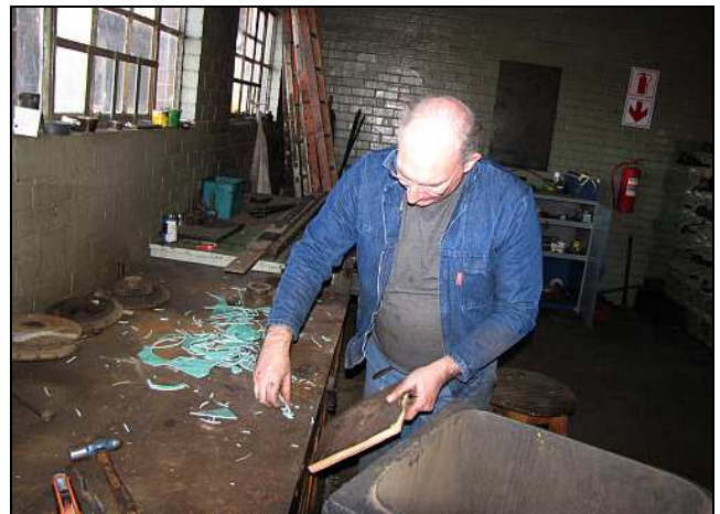
F10 – Aidan clears the cuttings away. This stuff is sheet Klingerite. It's good stuff for hot applications but this universal grade sheeting doesn't handle joints with different materials too well and can be troublesome on brass/bronze joints due to the high thermal expansion. It's fine for this application but laboursome to use, as you can see..
