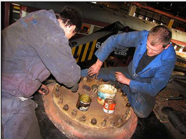
F01 – With the copper sealing ring freshly annealed and replaced under the cover, Swakhart and The Smudge are happily chatting while spinning cleaned hex nuts onto the freshly greased studs.
