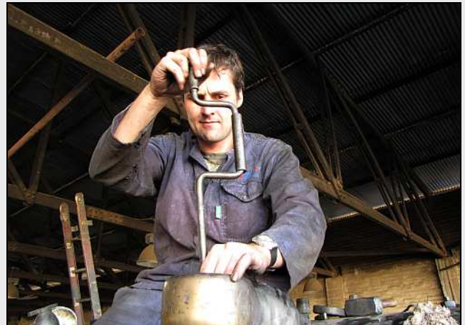
F08 – Dawie was later lucky enough to find a brand new valve cutter head, still in its original protective wax coating. So he was able to cut that seat down smooth and re-lap the valve. But the job will need doing again soon, unless new valve elements can be sourced or fabricated.
