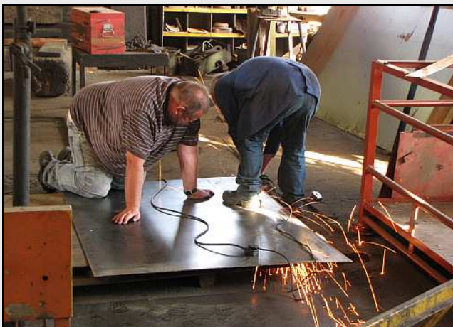
C05 – Gordon and Robbie start working on cutting out steel plates to repair the floors. They were concerned about the length of time it would take to cut the plates and weld them in – especially as there are 4 more coaches still to do! But this job was cancelled after a single cut.
