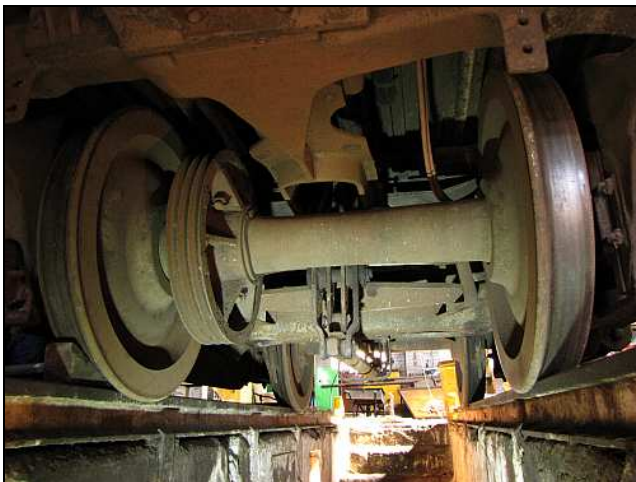
L03 – That unused split-pulley for the axle-dynamo drive will be the next scrap item to go. Hennie would need to get up into the gaps and uncouple the bolster ring and then disconnect the brake rodding. Short guys can stand under the flooring, but then their arms are too short. Sheesh!
