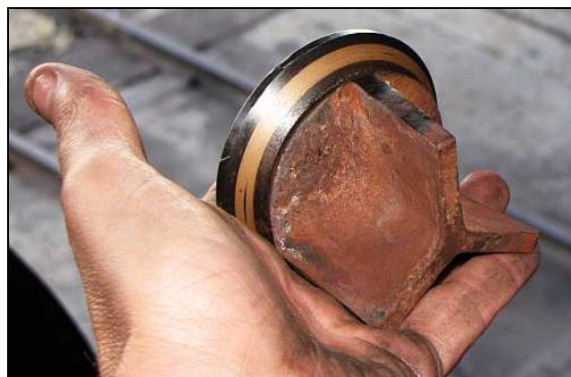
F06 – The problem is that the spinner vanes are a bit worn, which allow the valve to tilt in the housing. A small steam leak can quickly cut a groove into the valve components. It also accounts for the inconsistency that we were experiencing with the steam leak.
