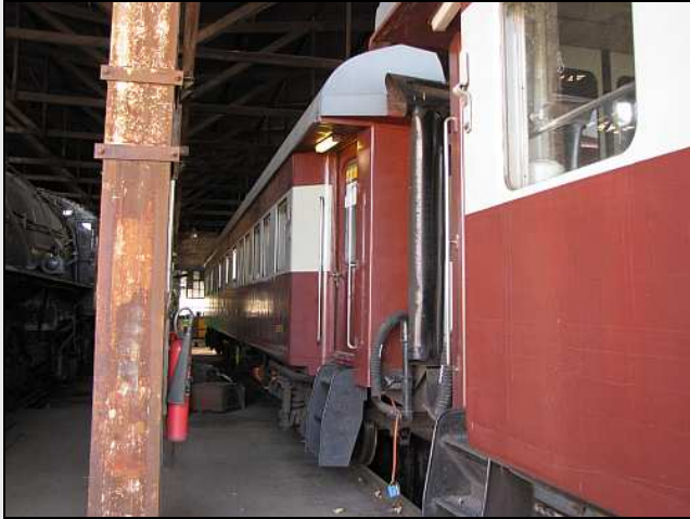
L01 – The Sleeper Coaches all have to be lifted off from their bogies at alternate ends to inspect the pivots, bolsters and their bearing rings. We'll lube-up the brake rods with the coaches up topside, as the light will then be better.
