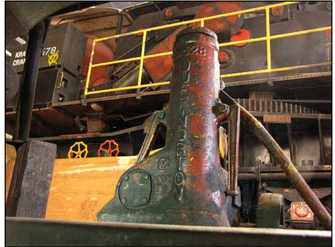
L02 – One of the pneumatically powered 'Duffy' jacks waiting for service. (The manufacturer's name is Duff-Norton – still trading today.) The hand ratcheted jacks are known as 'Bhudda' as they are of the BUDA brand
