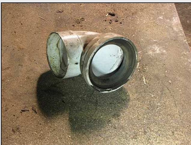
C29 – Another fine Setimela stuff up. To ease the fitting of their PBC waste pipes, they had used the rubber-ringed pan couplers as standard bends between pipes underneath the coaches – so some of the pipes were not rigidly joined.
