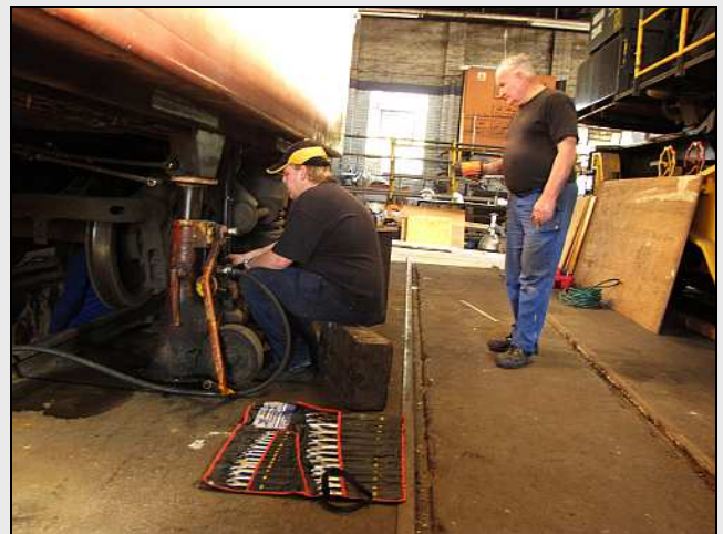
L04 – Victor operates the 'Duffy' Jack on this side while Alan operates on the other side. Attie is aiming his torch at the pivots and brake rods to check for any entanglement or trouble. Gordon was assisting at the end to check that the coach didn't tilt with the two independent jacks at work.
