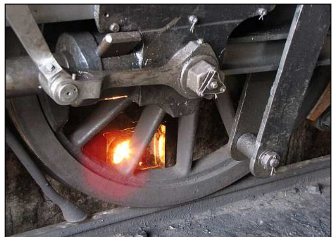
M06 – Class 15F 3046 driver wheel over an illuminated inspection pit. The worn valve gear bushes have been remade in Vesconite and reinstalled, so she's basically ready to run again once the boiler tests are done and the fire arch rebuilt.
