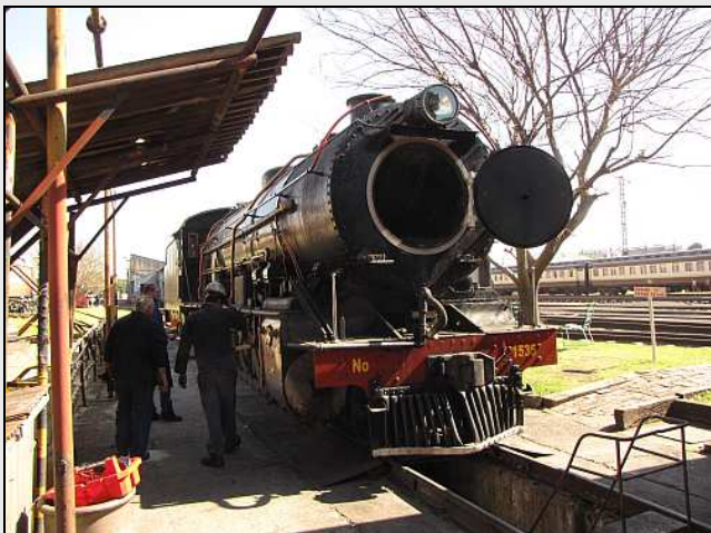
W01 – Our Susie Girl had been pulled out over the ash tracks for some undercarriage work. The smokebox had been cleaned out and washed the previous week. Jeandre had left the door open on purpose to help it all to dry out.
