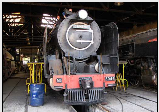
F12 – 15F No.3046 is happily being worked on with two gangers sharing the same pot of grinding paste! Two of the washout plugs incorrectly installed and the blow downs need to be blanked, but otherwise she's ready. Gordon would test-fill the boiler to mains water pressure this week.
