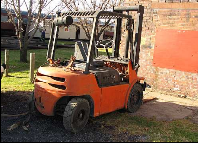
M01 – Shield Chemicals also donated an LPG-burning forklift to the depot. This Hyster is intact and just needs a bit of wiring work and the HT ignition system put together before going back into service, and likely a new battery. We even got four gas cylinders in the deal. Thanks!
