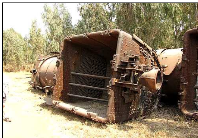
P03 - The original specification welded-trough style firebox base of a GMAM locomotive is visible on this very dead boiler. Notice the lack of the typical double row of closely-spaced diagonally-offset rivets at the bottom of the firebox (now the left) to hold a foundation ring in place.
