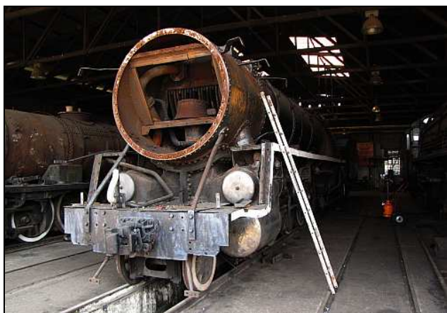
P02 - The raw-looking Class 15F No.2914 on Sat, 23 March 2013. She was then having even more rear-end hardware removed for better access to the ash pan and the condemned firebox foundation ring.
