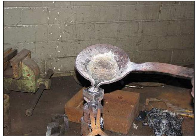
W06 – The 12AR was also treated to a freshly-cast set of fusible plugs as the fitted ones weren't standing up too well. The photo shows the hot, melted lead being poured into the core cavity, while the plug is being held into a mandrel with a semi-hemispherical cavity to mould out the domed head.
