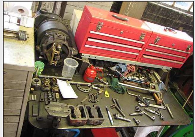
W08 – The Sandstone Crowan Sheldon Steam Crane No.578 project is continuing with further stripping and analysis of the two dismantled feedwater pumps, many components of which are seen on the work bench.
