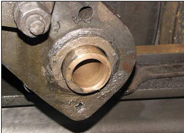
W07 – Class 15F No.3046 has had the front end of her left valve motion stripped due to excessive wear. Pictured is the eccentric bush that forms the bearing between the eccentric rod and the expansion link. When the locomotive was recommissioned 3 years ago, these bearings were incorrectly made from plain old brass instead of the proper phosphor bronze and they have worn badly in service. You can see the outer wear gap even in the reduced photo.
