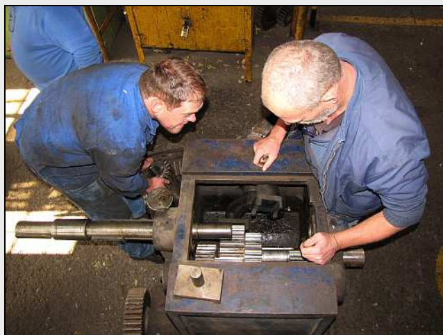
P14 – Shaun Ackerman (L) and John Gundry (R) had just withdrawn a keyed shaft before attempting to fit a sliding pinion gear.
