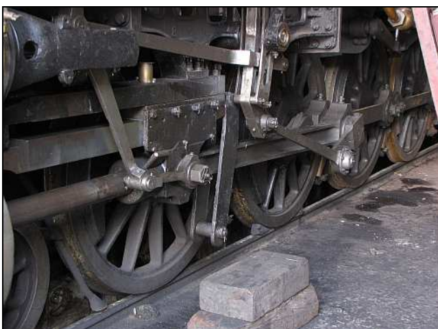
P09 – The LHS valve motion on Class 15F No.3046 'Janine' – just reassembled after replacement of three worn bushes with new ones that were custom-machined in Vesconite™.
