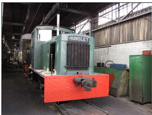
P12 – 'Andrew' the little Hunslet waits for his newly primed engine covers to dry, before they could be painted and fitted. (Since done.) You can see one cover against the cabinets behind the buffer beam.
