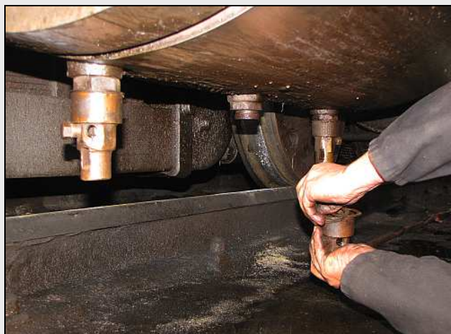
P02 – Fireman Johann Breydenbach discovers some stacked copper sealing rings, while realigning a cylinder cock. (The cocks were discharging inwards.)
