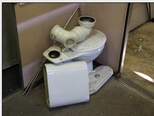
P30 – The close-coupled toilets will be cleaned and reinstated. These will still discharge to trackside, which won't be so bad on a tour that is mainly moving and not using the train as a 'rolling hotel.'
