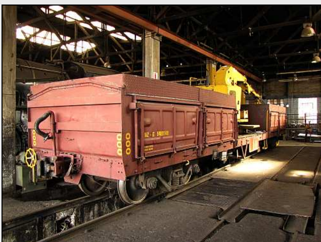
P11 – The Coal Handling Wagon in the 15M shop after the bent, cracked clam-shell grab was repaired and reassembled, and a bent scuttle plate straightened and welded back on again.
