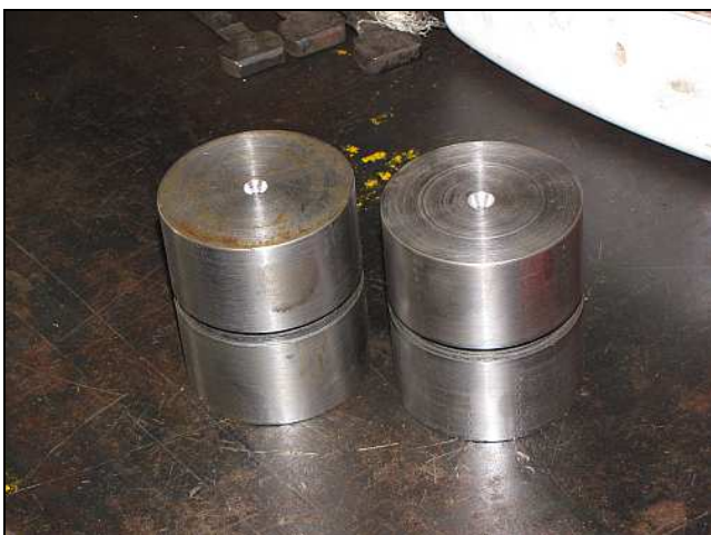
P21 – A pair of steel blanks (By James Thomson) that will become new steam-driven pistons for one of Steam Crane No.578 boiler feedwater pumps.
