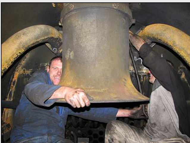
P07 – Michael holds the gwalan n' tube socket combination firmly onto the bolt, while a cheerful Shaun reaches for the lower end to give it a pull.
