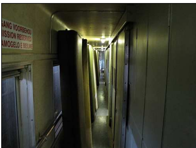
P29 – A silver class corridor full of bunks that had been removed. Silver class compartments will now run with two bunks along one wall, but more widely spaced and using the foam mattress as a chair back.
