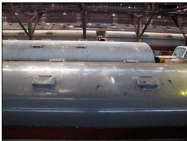
P24 – Where once the GMR locos underwent running repairs, the RS coaches now sleep. Note the details on the 'Monsoon' vents, with the side loops acting as rain shields for the actual vent apertures.
