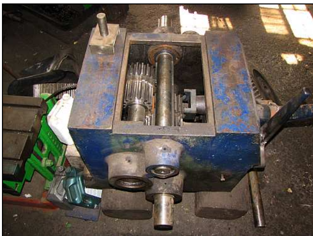
P13 – The incomplete Input Gearbox for the Wheel Lathe drive. It was being temporarily reassembled to check the meshing of the gears and the bearing fits.
