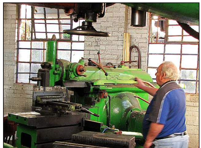
P94 – Due to the lack of volunteers skilled in these areas and also not required elsewhere, we weren't able to have many live-action exhibits in the 15M workshops this year. Here, James Thomson is letting one of our two Thule Shapers run on a piece of scrap steel.
