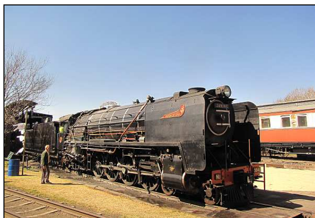
P86 – Just as in the lore for service pachyderms, steam locomotives can move surprisingly quietly. Class 15F 3046 had uncoupled and been turned around the balloon, and had just backed in slowly for fire servicing. The visitors would only catch-on once they heard the intermittent raucous hiss of the grate shaker stirring up some ash!
