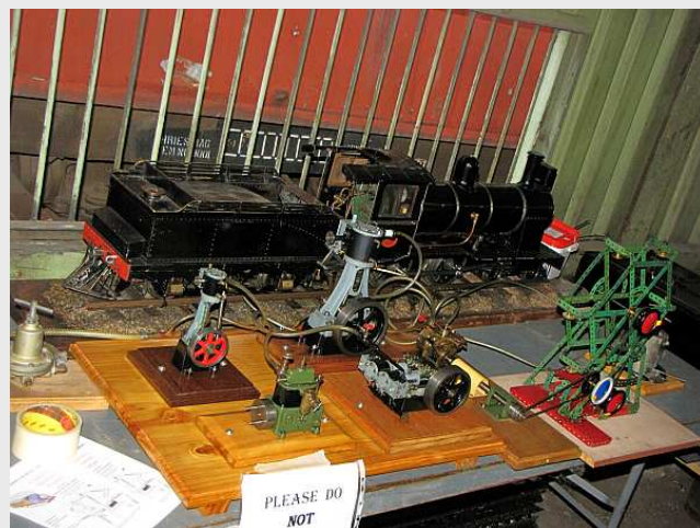
P100 – A display of model engines running on compressed air, including a marvellous compact little bronze V4 oscillating cylinder engine driving the ferris wheel.
