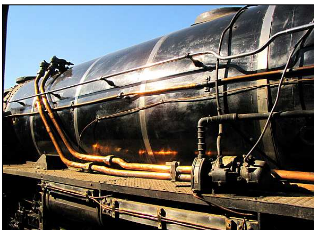
P111 – From the rearmost coach, one had an eye-level view the characteristic double-feed pipe arrangement on the 25NC. This is a heritage from her days as a condenser when the boiler was fed from pumps instead of Gifford Injectors mounted on either side of the cab underbody.
