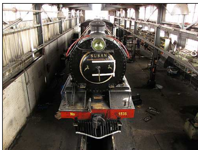
R06 – Susan, the last surviving Class 12AR – A forehead view. Note the clench bars resting on the front risers – the smokebox door wasn't latched closed.
