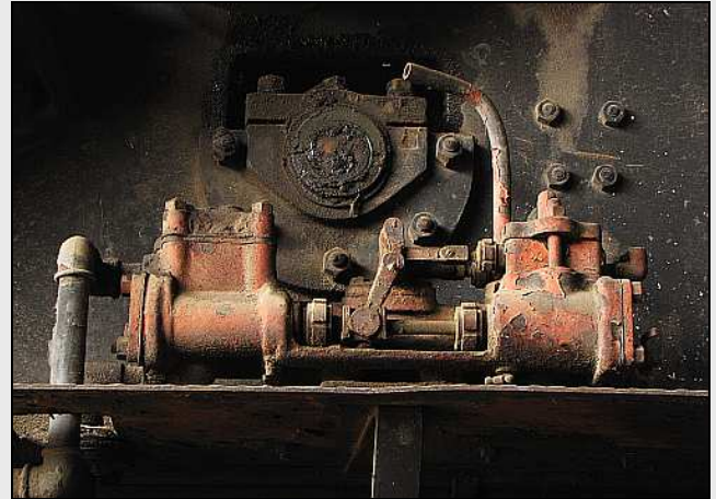
D02 – Here is a very similar duplex feedwater pump as fitted to the 36 ton Booth Rodley Crane No.96. The twin cylinder steam engine is to the right, with the water pump at the left, and you can see the valve hammers in between.
