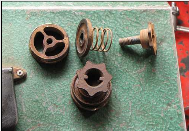
D03 – The outlet valves (four for each feed-water pump) all survived in reasonable condition, with springs and adjusting nuts intact. They just need to be cleaned, matched to their seats and then individually lapped in again.
