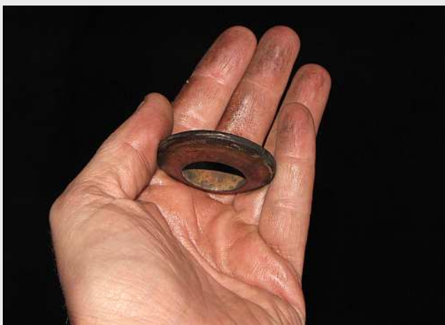
R15 – A close-up of one of the double-conical olives that seal the joint between the water column cocks and the backhead's flanges. Unlike compression olives, as in many solid-wall fuel or hydraulic lines, these don't crush into place. Unfortunately, they can shift during installation and a dry, cold fit can't be tested. Fitting water column cocks onto a steam locomotive is a lot trickier than it looks!
