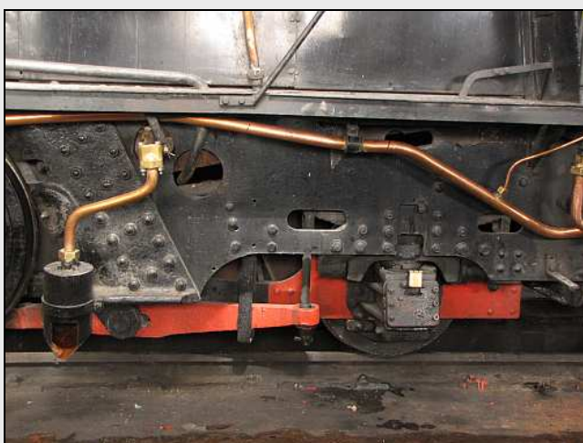
R05 – A side-on view of the equalizing beam (in red) and the rear suspension. Notice the small upper oval-shaped access holes which make that ash pan such a joy to clean.
