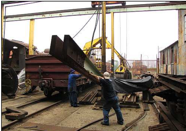
S03 – Juan guides the suspended load straight as the beams are carefully lowered, with the other, heavier end (with the clamping plates and rams) already on the ground. The strange, sideways tarp in the middle-ground is covering the two tool towers for the wheel lathe.
