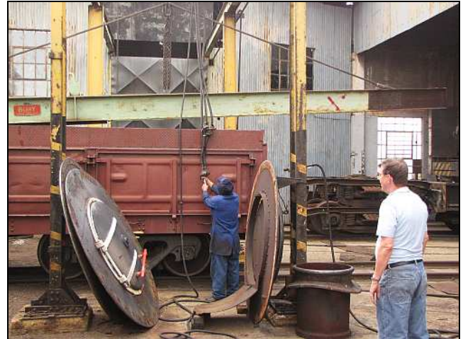
S02 – The swager gang managed to lift it with a cable sling using the pneumatically powered crane – but the load was too asymmetrical. The coal grab was used carefully at the end to keep the cable sling from running through the hook.
