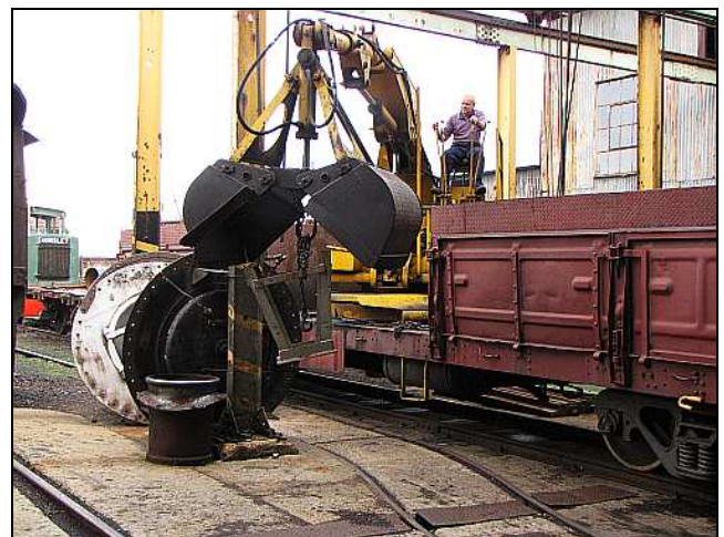
F12 – Andrew took over on the grab's controls in the 15M yard to warm up before tackling the next project – the Tube Swager. Notice the damage to the coal grab's bucket – done by a previous staff member by directly lifting coach bogies. Repair work started on the bucket last week. (21 st )
