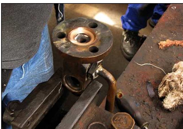
R17 – A sign of a good seal would be a matching contiguous, concentric ring of bright, clean metal on the seat and on the sealing olive itself. This one is only half way through the process.
