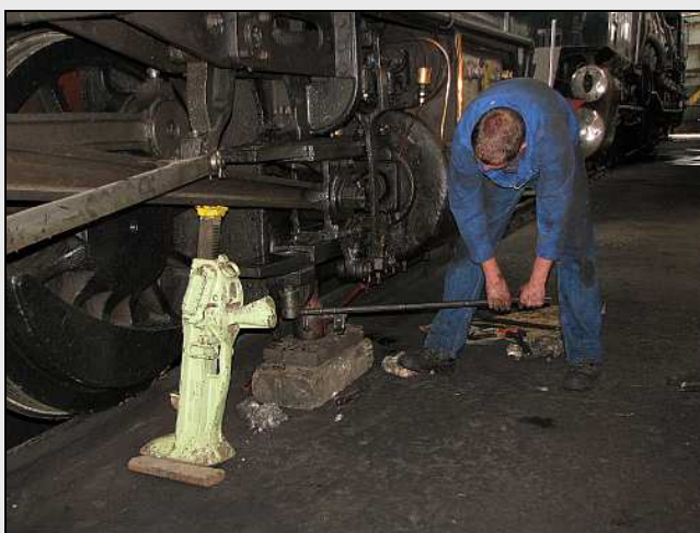
R11 – Doctor Smudge is tightening up the rear shim bolt to seat a newly inserted shim on top of the existing shim-stack. The front end is held on by two smaller bolts. Note the jack under the crank rod – it is taking the weight of the rod, bushing and crosshead away from the lower slide for measuring.
