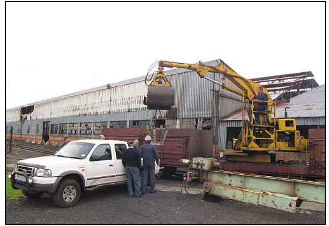
F08 – A nice easy load for the coal grab and the fly press's stand is lifted upside down. The 4-way octopus chains hanging from the coal grab's bucket are shackled to the central impulse plate and they are removed for coal loading service. Dawie (R) and Dennis had come out for a look.
