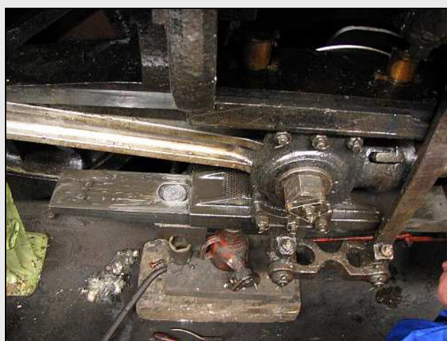
R10 – The ideal slipper gap on this locomotive would be 1mm. The slide bars are too unevenly worn to get this clearance set up, so a compromise had to be made. Eventually, the four slide bars will need to be removed, and the white-metal surfaces re-machined straight and parallel.
