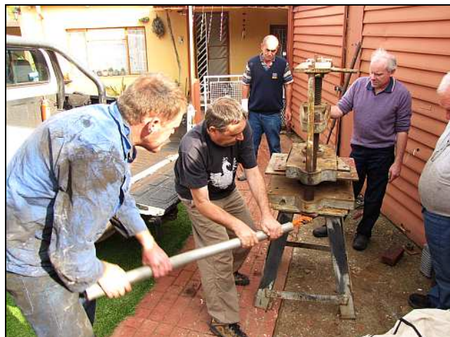
F02 – The fly press was smaller than any of us imagined it would be, but none of us were fooled by its ‘diminutive’ size in terms of weight. We took turns in removing the guide rod nuts to split the press into two easier-to-handle pieces.
