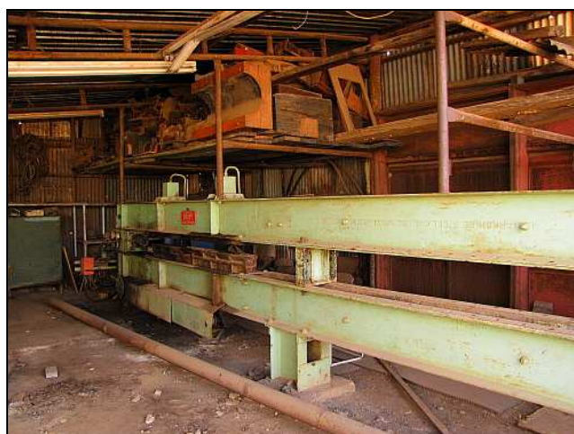
L12 – The Tube Swager at SANRASM North Site’ Machine Shed in Sept. 2010 – it also held up the shelving and the shed roof itself! Visible are the tube V clamps and vertical rams to hold the tubes in place. The center piece can be unbolted and relocated to suit the length of the boiler tubes.
