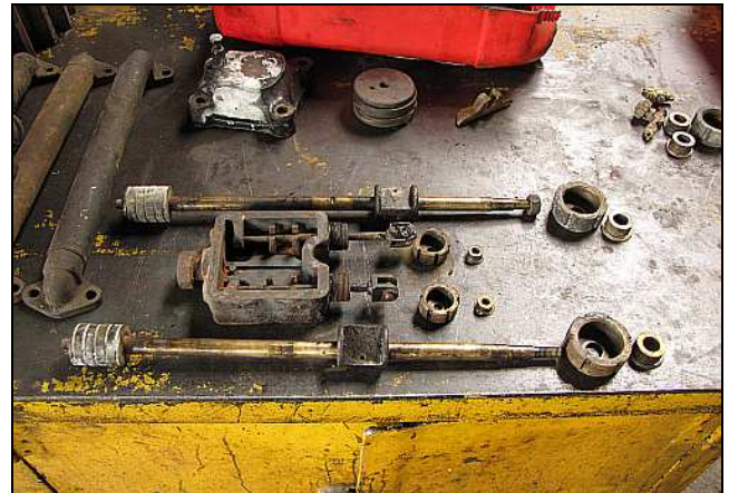
D04 – The valve gear all survived intact, but with serious wear at every joint and at every gland. Here you can see the valve chest between the piston rods and packing nuts. The water pump rings (L) had corroded into their grooves.
