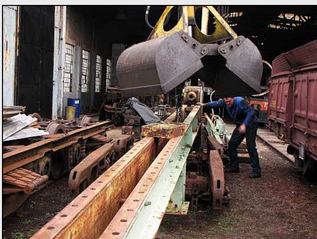
S11 – The lower half of the swager is guided into position. In mid-field you can see the tube stopper that acted as a very useful adjustable counterweight during the operation. In the background, alongside those windows, is the location to which the Tube Swager will eventually be moved.
