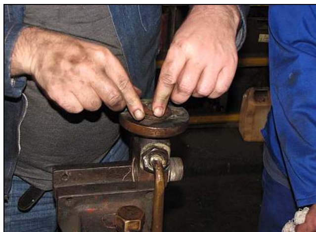
R16 – The olives are lapped in like a poppet valve against its seat. Grinding paste is applied to the conical surface and the olive rubbed vigorously against its matching recess. The same process is done with the other side for the backhead and the two sides must not be flipped. But even a ground-in olive will leak if the cock and its flange are not parallel or the flanges are distorted.
