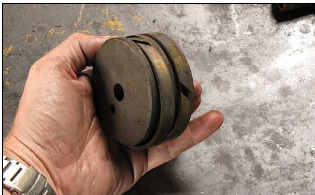
D05 – The two steam-driven pistons are worn as well and new ones will need to be made. They will need to be made to match the cylinder sleeves, which need to be bored out oversized and parallel. The piston and valve rods are also worn, but they will be machined to consistent sizes and re-used with seats and bearings remade for a custom fit. It will save time but has the disadvantage of rendering the pump parts no longer interchangeable with each other.
