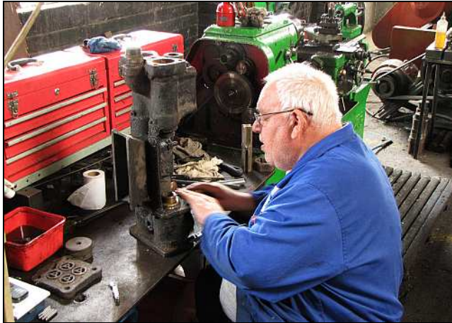
D01 – His name is James and he can make a lathe sit up and beg! But for now, he is happily absorbed, with a cup cake inside him, with further strip-down of one of the boiler feed-water pumps from Sandstone's Steam Crane No.578.
