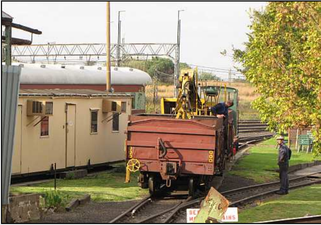
F07 – The other end of the shunt – the coal handling wagon is approaching. Seen from the ends, its genesis from a DZ type gondola wagon is clear. In this pic, I liked how the brown leaves of the foreground tree merge in with the T&P tree which is actually far away in the background.
