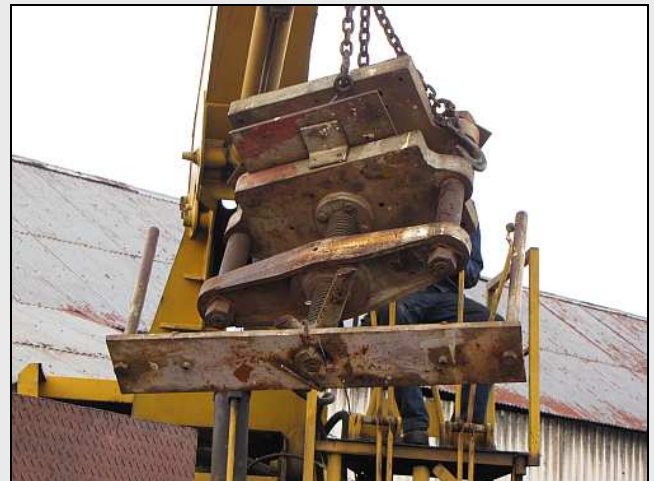
F10 – A top view of the press going up. By replacement of that handle with a properly weighted one, we expect this to be useful for small work. The two existing hydraulic presses are powerful, but they are also hard to modulate.
