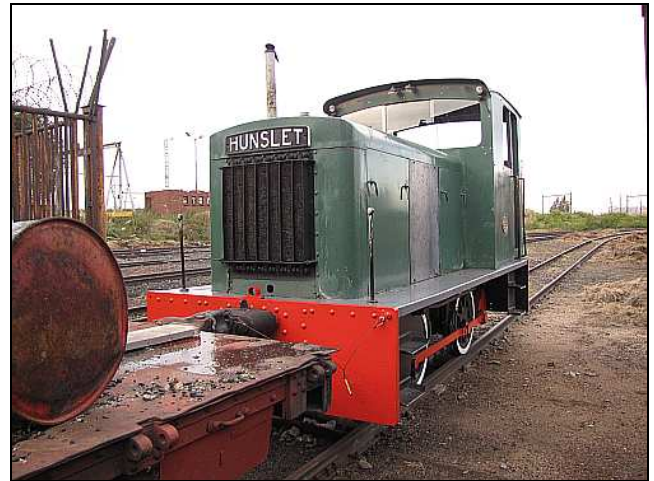
M08 – ‘Andrew’ the Hunslet Taylor shunter has recently been smartened with painted wheels, rods, walkways and buffer beams. Notice one of two new engine covers. It is of corrosion resistant steel, but will still need painting soon.
