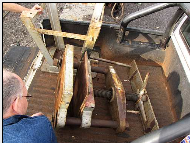
F04 – A view of the press itself. Fly presses use weights on long levers to add inertia to the turning motion. They can be used as die punches too. This press used to have a weighted fly wheel – of which some spokes can be seen.
