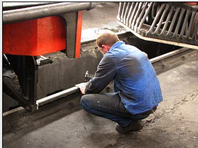
R14 – Rail heads are naturally plentiful around any loco depot and they are also useful as impromptu anvils. The incomparable Dr. Smudge is seen tapping a bend out of one of the rectangular two-holed front shims.
