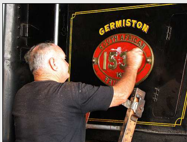
M18 – Oude Drywers never die, they just get demoted to cleaners! (Right back where they started, decades ago!) Attie is aware of the irony, but he is still happy to do this stuff. That ‘Shield’ brand polish worked well on the brass oval, but the buffing machine took some of the red paint off the inset surfaces. (As that paint was never primered.)
