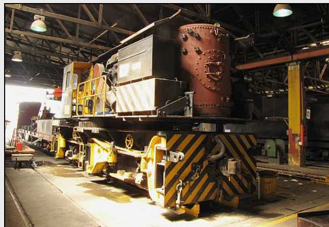
P02 – Crane No.578 is shopped-in for boiler testing. The foundation ring rivets all need to be replaced as they hadn't clenched properly when they were previously installed by parties unknown. The boiler base leaks under gravity fill.
