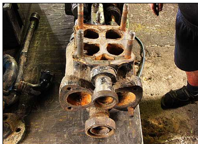
P04 – This complicated casting is the duplex water pump, with the lower pipe as the inlet and the upper pipe pressurized by valves – thus the inlet is 'swamped.' The bow-tie shaped flange is for the pump's cylinder heads. The casting had cracked into three pieces and had been re-welded. James plans to have a new one fabricated.
