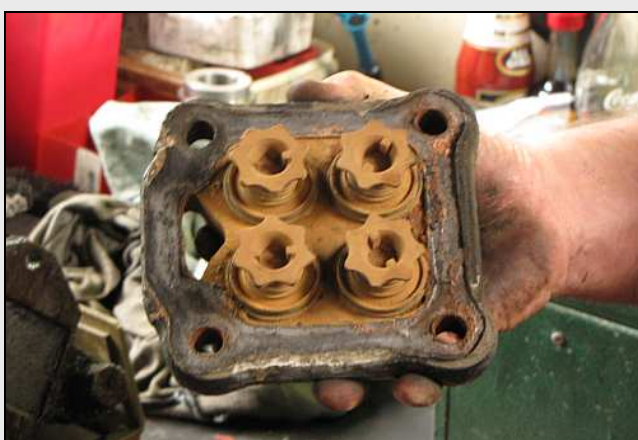
P05 – Here's the upper side of the valve plate. The spring-loaded poppet valves were all mercifully intact on both pumps. The disks will obviously all be lapped in. The water flows from the bottom up through the one-way valves and then down to the outlet via that triangular aperture.
