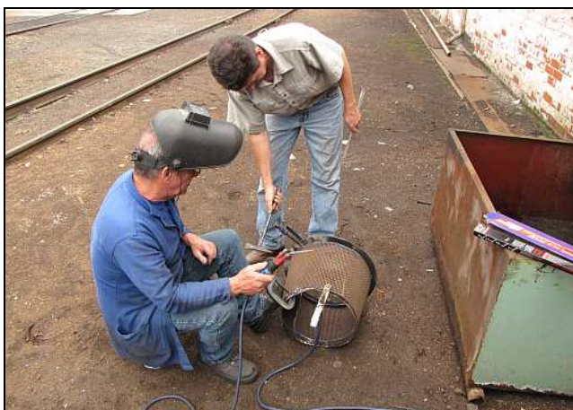
B09 – Alan taps the slag off the welds while Gordon (sitting on a paint tin nearly hidden by his overalls!) takes a breather. The chaps cut down a spare Class 15F cone to get a decent grid 'basket' and were cutting and shaping in a customized particle shield as well as fitting the new cone to the Dawie Cone's existing upper flange. (The wide end.)
