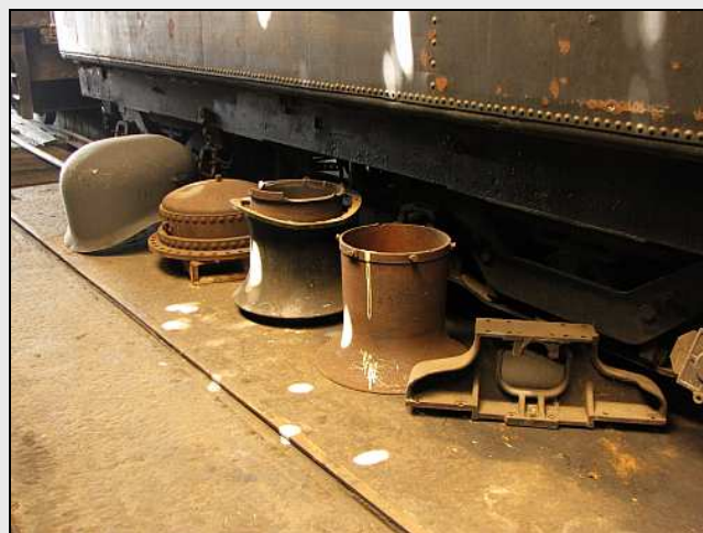
M14 – The bits belonging to 12R No.1947 ‘Rusty Rosie’ have been neatly lined up and out of the way. From rear to front, a dome cover, a steam dome, the original chimney, a spare blast petticoat and the steam reverser’s pedestal.
