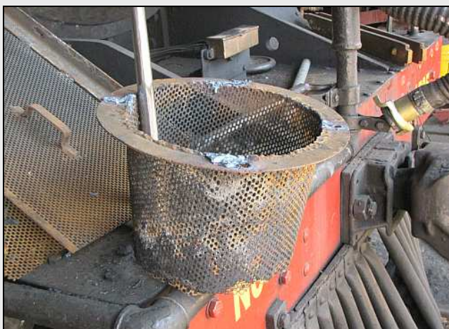
B11 – Here's what 'Susan's' exhaust 'basket' looked like in May 2012. The lower end was being eroded away.
