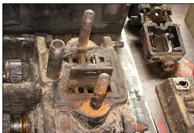
P06 – One of the D-valve elements and the port plates. The 2 nd & 4 th of the five ports are not admission ports as may be supposed. They expose more valve area to the differential pressure between the live steam and the cylinder – helping to press the valve down for a better seal.
