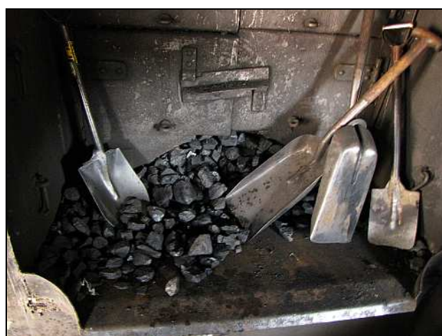
M12 – Seriously, how many shovels does The Mini Mienie need when firing the 12AR? The round-nosed shovels as on the left are better for coal trimming as they are easier to dig into the coal – the smaller point exerts higher pressure.
