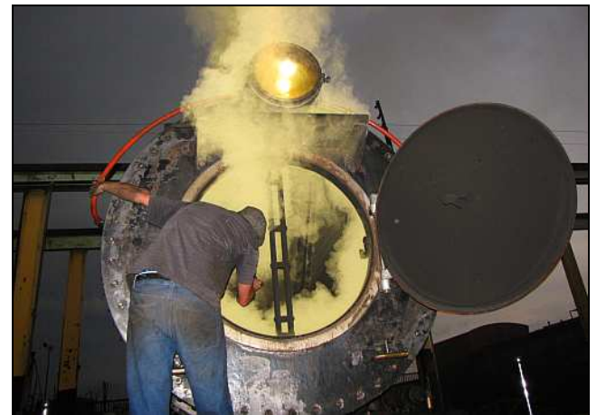
B04 – Where today’s work started – during the steam test, the induced draft blower was found to not be working. Shaun Ackerman is seen trying to ‘smoke-out’ the bug. We could hear the blower roaring inside, but there was no draft.
