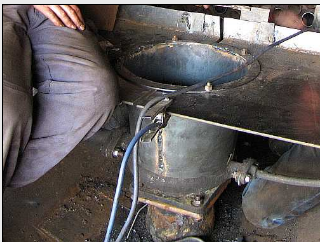
B07 – THIS was the problem – the solid-walled blast cone that we had Dawie Viljoen fabricate for us to try reducing the 12AR's tendency to throw sparks through the chimney when working hard. It turns out that the laminar turbulence, and the inability of the blower's steam jets to mix with the surrounding gasses at their source, render the blower ring totally ineffective – although the exhaust worked fine.
