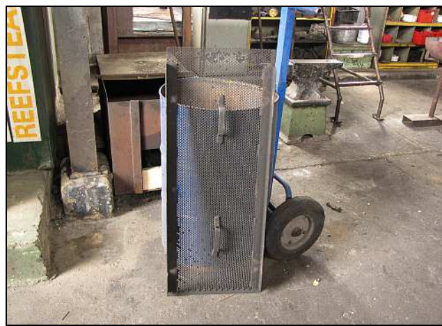
B12 – One of the three spark arrestor plates, which is still fairly clean! What a chore these are to unclog!
