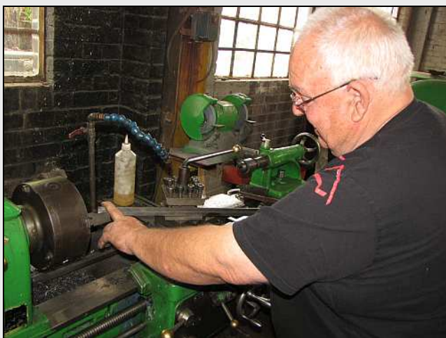
M07 – Our chaps have been battling with this lathe recently as the cutting tools are starting to chatter. James shows the cause – the lower clamping plate on the tool holder has become distorted. James is planning to make new plates, and a matching tool holder for the other end – one dedicated to machining and one for cutting threads.
