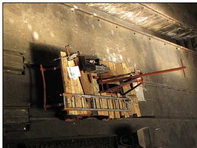
M20 – The deck planks have been put back onto the pump-trolley, all with more 'character' after being used to support components in the 12AR's smokebox. The trolley's crank rod had been removed to immobilize it, before someone hurt themselves playing on the unfinished little machine.
