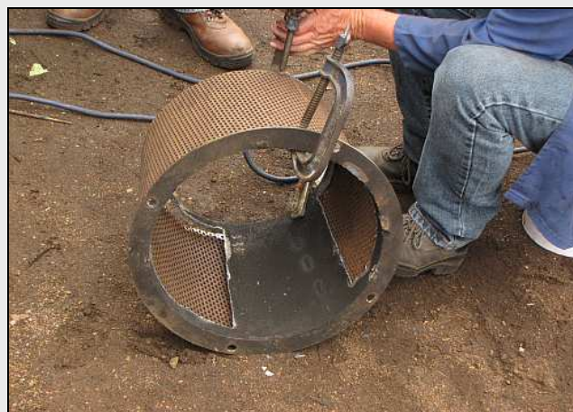
B10 – A view from the top down of the new cone clearly shows the new shield segment that will face the tube plate. Thus the 'sparks' that get through the lower, center boiler tubes will still not have a direct path right up the smoke stack - but the blower ring's annular jets are still contiguous with the smokebox's air-space via that conical grid.
