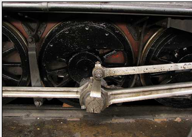
B03 – Susie’s driving wheels are now all black – the spokes were originally bare steel. The motion has already been wire-brushed but not yet scrubbed and wiped clean. It’s a surprising amount of work cleaning all that naked steel!
