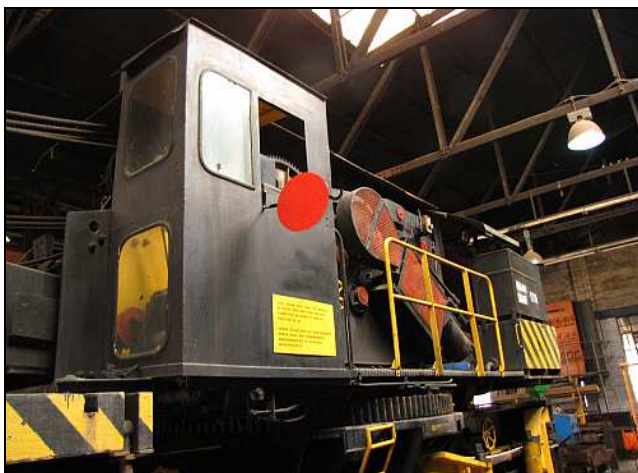
M05 – Sandstone's Steam Crane No.578 is now also correctly flagged-out for maintenance work. This old crane has even has its own built-in anti-intruder system – once again, a swarm of wasps have made their home within the cosy, secure confines of the geared slewing ring.
