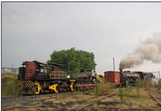
P01 – One of the first jobs for the 12AR, shunting Sandstone Heritage Trust's 60T Cowans Sheldon steam crane from the Carriage Shed into the 15M workshop. The two titular donkey pumps had been removed previously.
