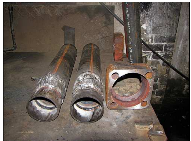
B30 – The steam pipe ends and the steam chest collars wait ready at the end of the day. The smaller pipe ends are to be expanded into tapered rings and then the collar loosely slipped over the pipe before it is tacked together.
