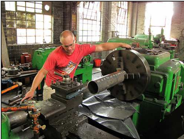
B25 – Mike exchanges Millsite Style for ESKOM Style and turns the big lathe by hand to cut the inner chamfer. This pipe has to withstand boiler pressure, so the welded edges have to be chamfered for full deep penetrative welds.
