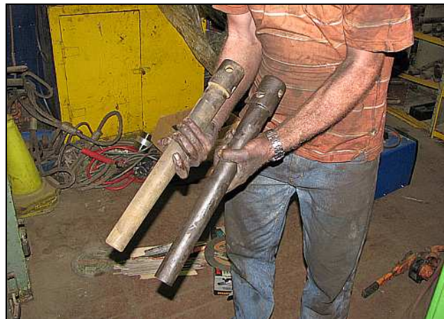
L14 – Just one more despondent rummage in the tool store (soon to be vacated) and SUCCESS. The bigger conical expansion mandrel had been found. (It is the one on the left.) So, we could have one more go at the leaky flue tube.
