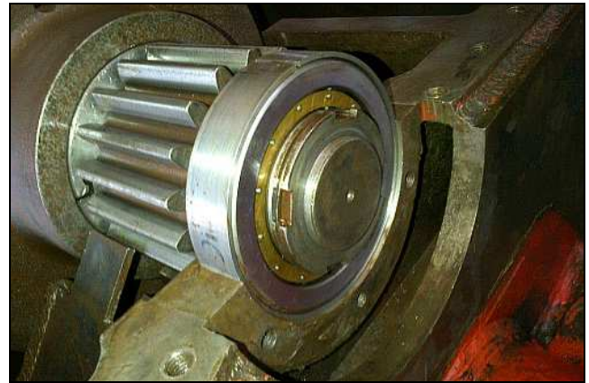
G08 – This gear is the jackshaft drive pinion. It survived the break-up of the jackshaft's old gear's teeth, but the old roller bearing got a good dose of the grindings via oil transport over the gear teeth. The canted steel ramp is one of two oil runners which fill up the 'upstairs' oil sump from this gear's drippings. (Pic by VLM)
