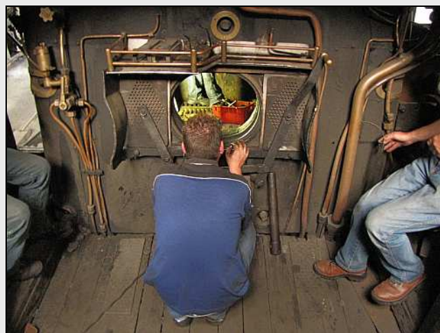
L08 – It is fascinating watching guys working in the firebox and Simon gets caught in the single-channel 'Tube-Tube.' The wrapper sheets and boiler got wetted with that extra leak, so the fellows would concentrate on those tubes instead and check for external leaks again during the week.
