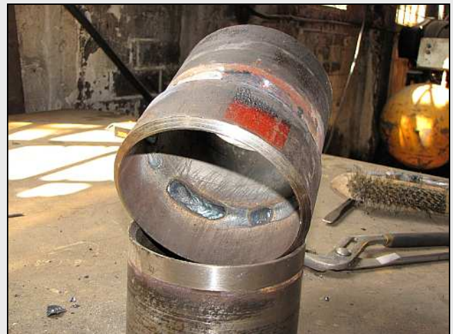
B28 – Here's a view of the start of the second pass of the interior weld – as seen through the full width ring that would be welded to the rest of the straight down-pipe section. Note the cleaned and chamfered edge at the near end for deep-penetrative welding to the straight section.
