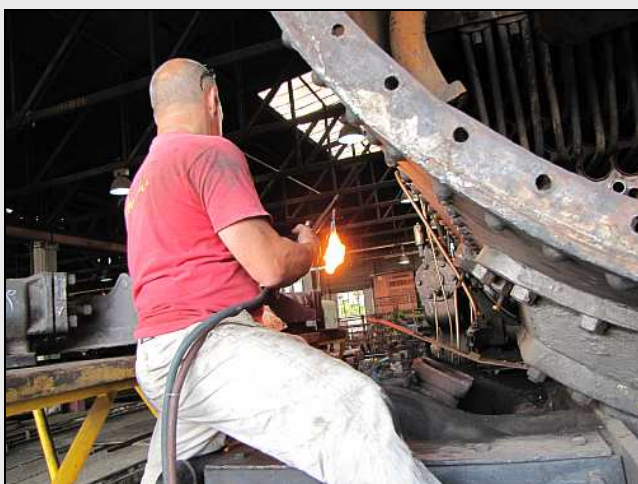
B15 – Michael was also having one of those moments. He had many today, in fact. The acetylene torch's pintel needs servicing and it kept flaming-out with the unforgiving tightly tapered flame necessary for the close-quarters work.
