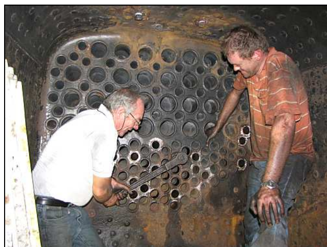
L18 – The flue tube seemed to seal up OK. Gordon Bennett has a go at a tube. Due to a general abdominal hernia risk, he wasn't able to take the ratchet up to the full-squeeze, but he did manage to get a few good licks in.
