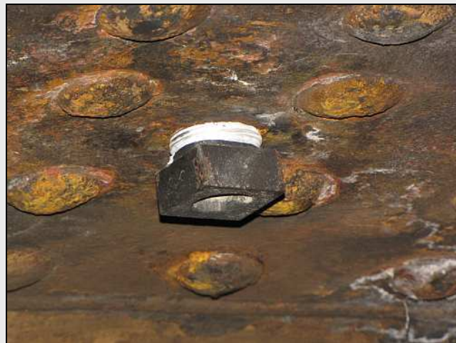
L20 – A cleaned and serviced fusible plug. (The other two will be removed before the first light up and they will be cleaned and the lead section re-cast n' date-stamped.
