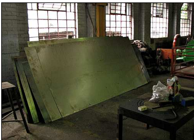
B17 – A load of steel plate has come in. This is for the fabrication of baffle plates and repairs to the table and toe plates for the 12AR's smokebox, and the leftovers for 15F 2914 – although she will need even more plating to repair to the horizontal sections of the tender's coal bunker.
