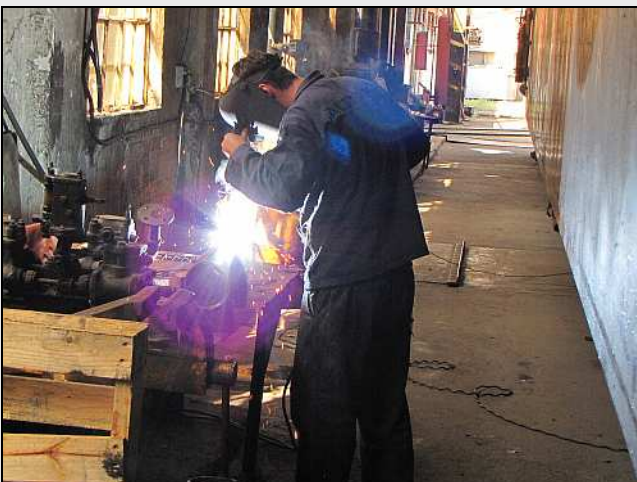
B29 – The magnificent Viljoen was happily occupied welding these pipe ends for most of the day and it kept him out of our way. Both steam pipes will now have matching 6.6mm diameter thick walls and should last many years.
