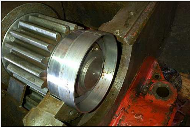
G07 – They had forgotten the seating rings, as they had been stored separate from the rest of the components. Gordon found them. These bearings and the previous set (both metricated) are slightly smaller than the originals, hence the need for spacer rings. In fact, the first set of spacer rings were made from brass strip! (Pic by VLM)
