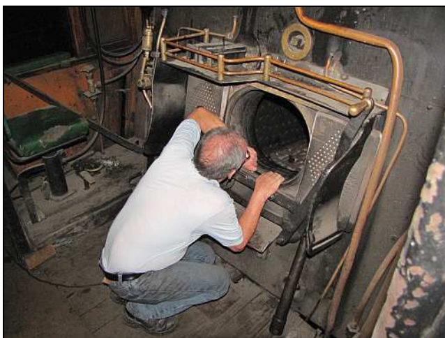
L07 – For the afternoon test, Gordon is keeping an eye on things and for instructions concerning the boiler pressure. Jeandre had mistakenly loosened a safety valve blanking plate to vent the boiler during the week and hadn't made a water tight joint – so that caused some leaks on Saturday.
