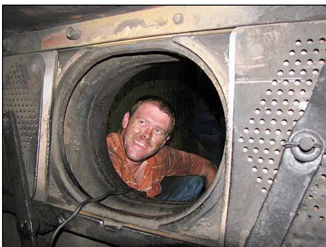
L11 – Dr. Smudge looks cheerful enough, but there was a little rat of worry scurrying within his mind. We had run out of taper on the mandrel for the flue tube's big expander, and two of the smaller tubes just would not stop weeping.
