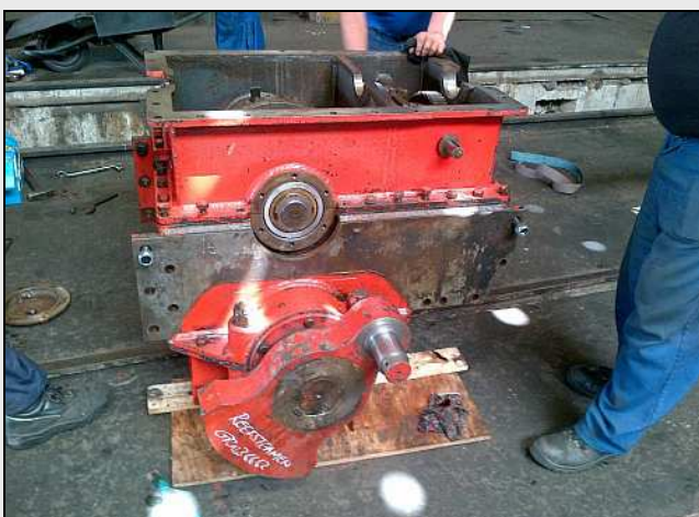
G11 – The upper frame is being bolted in. This gearbox goes together like a big ferrous sponge layer cake, with silicone sealer applied as an oil seal on the joints. Notice the new square key on the counterweight. (Pic by VLM)
