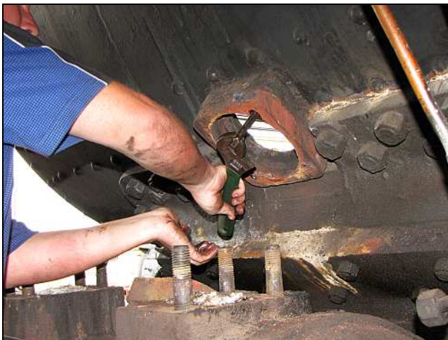
B09 – Simon is busy re-tapping the stuffing box cover for the vacuum seal. 'Big Robbie had just finished removing the upward pointing studs with the largest stilson wrench he could find. Simon was about to discover that not all of the old stud's remains were out and that hole was too shallow.
