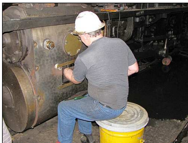
B16 – Aidan patiently settles down and removes the lube line's cover plate to try his luck at fishing around for that dropped punch. Us steam-doctors really don't like leaving tools inside the patient – but this one could not be retrieved.
