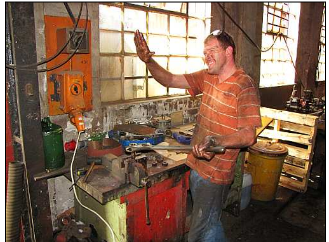
B08 – A potentially incriminating photograph that will remain forever in my archives as collateral. Actually, Shaun wasn't doing a Nazi salute, but joking about something taking off. Notice the die running on the stud.
