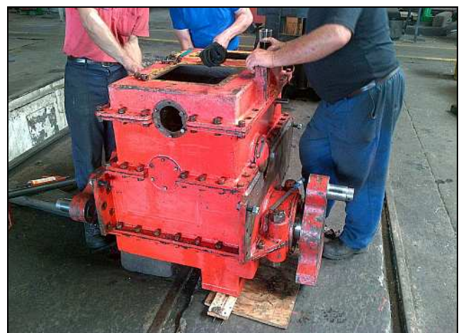
G12 – This rear view shows the gearbox is almost done and Attie (with the coke and boep) has ambled out to check progress. While it is clean, you can see the literally dozens of bolts that hold this 3D jigsaw together. (Pic by VLM)
