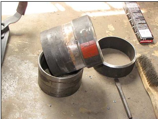
B27 – Dawie was busy making the lower end adapters as the steam pipes are wider than the sections that go into the steam chest flanges. The cut off piece was necessary to allow access for welding to the inside of the lapped join for a smooth path for the steam and for a stress-free transition.
