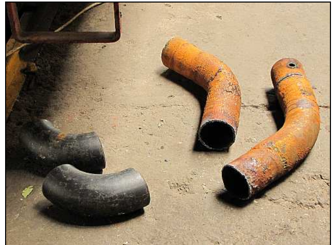
B26 – As complicated as the old down pipes looked, there was actually only one bend within the lower pieces once removed. We had the new bends fabricated and bent for us, while the straight lengths were standard sections.
