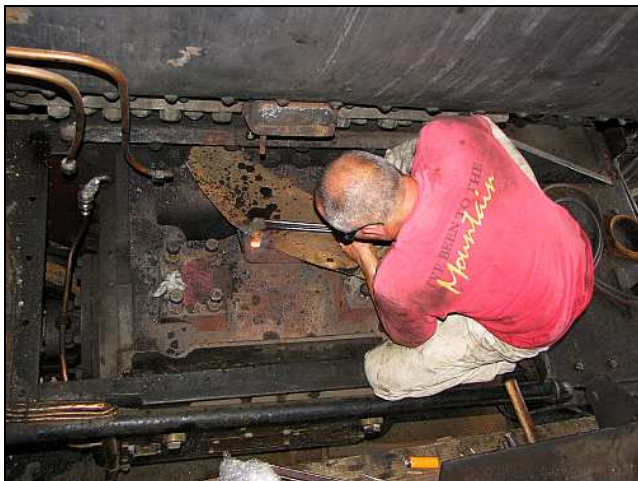
B13 – Another top view at the right steam chest (cf B04) – a stubborn Michael gets stuck into those stubborn studs. The new steam pipes need to be fitted and measured in-place for cutting, so all the old studs need to be removed beforehand, to be able to use temporary drifts and bolts.
