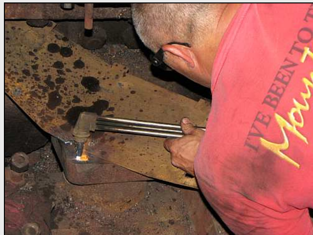
B14 – This picture shows the exacting nature of this work – Michael had to burn away the remains of the cut-down studs without damaging the flange. If you look closely, you can see some of the old threads are still intact. Naturally, the holes will be re-tapped, even drilling out, if necessary.
