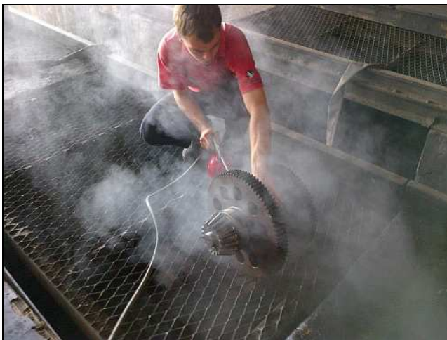
G09 – Jeandre Gordon does a final close-up diesel spray on the two-speed cluster shaft. The gears themselves are mounted on roller bearings - as they are not shifters, but are rather free-wheeling gears engaged by a double dog-clutch arrangement. Jeandre took care to clean those bearings. (Pic by VLM)
