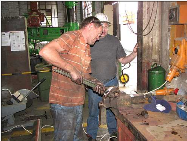
B07 – Of the studs pointing up from the steam chests, 3 out of 8 survived. Here, Dr. Smudge is running a clean hex nut along the threads, with lots of oil, for a rough cleaning and straightening before re-cutting the thread with a proper die.
