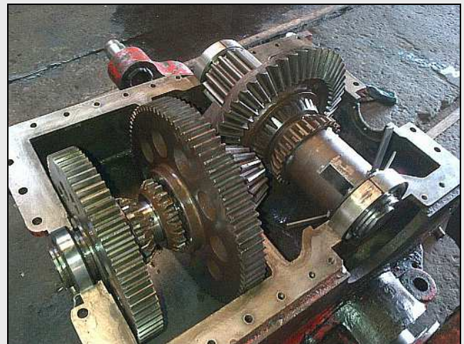
G10 – The shafts are in with the two speed cluster shaft in the foreground. The cross-shaft was once a reversing shaft and had a second crown gear working with that dog clutch. Reversing is now done with the hydraulic clutch. Note the oil dippers that take the place of the missing bevel gear in terms of drip-fed lubrication for the bearing. (Pic by VLM.)
