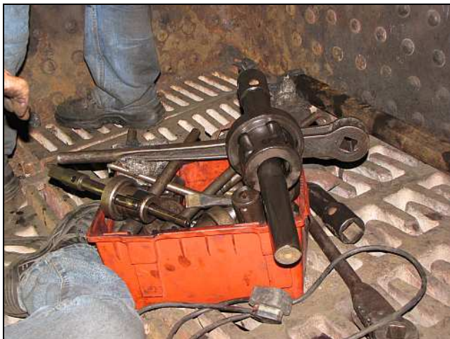
L19 – That big clanker on the top of the lunch box is the FLUE expander – compare it to the visible TUBE expander on the left. The mandrel is the second last one that we used.
