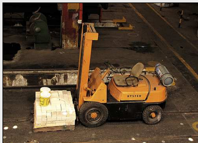
B18 – The fire arch bricks have arrived. The 12AR doesn't use special cast bricks as many of the more modern engines do. However, these plain-looking rectangular bricks have been cast with a 2 degree slope on the flat sides, to help build up the arc-shape of the fire arch.
