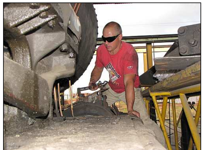
P12 – Mike 'Rekots' Thiel was tasked with removing the cut-in-half remains of the right side studs in the afternoon – requiring some delicate work with that torch! His compact but muscular build came in useful for those tight quarters!
