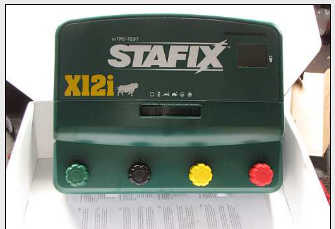
M18 – Here's the beast which was mounted and energized on 20 th Jan, although the HT wasn't wired yet. An interesting feature is a photo sensor that allows the setting of a different voltage for night time use – usually higher as that's when the buggers roam. Being mounted above a workbench, it will be easy to increase the battery capacity.
