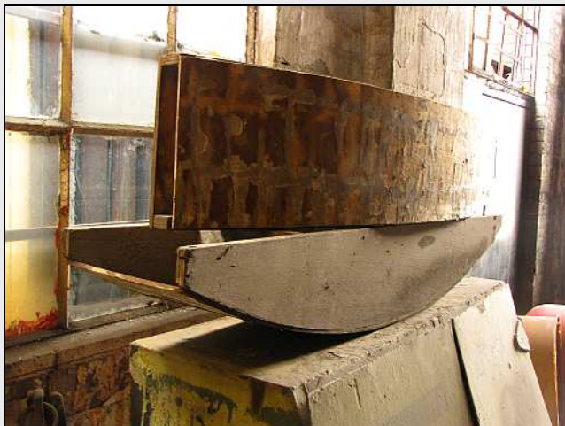
M07 – This pair of boat-shaped frames are the formers upon which the fire clay bricks of the 12AR's fire arch will be erected. As she doesn't have arch tubes, the fire arch will need to be supported while the mortar dries. (Even though it will use a wedging keystone, like a Roman arch.)
