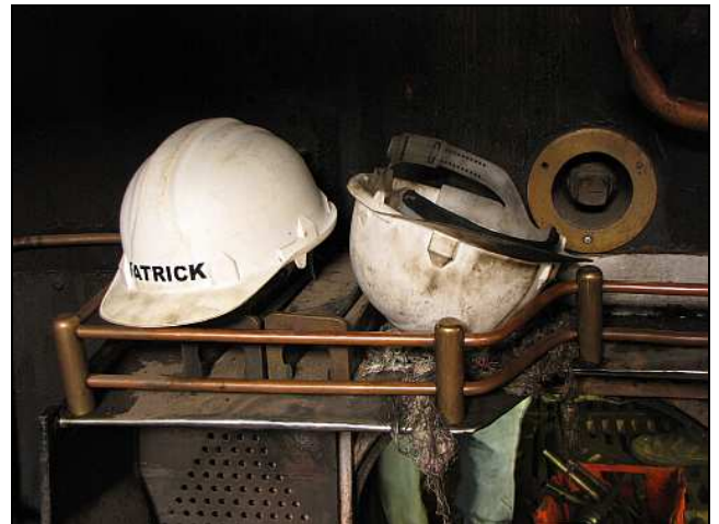
M16 – Hard hats are generally not worn for firebox work as it is generally quite hot enough in there, and they tend to come off in transit through the firing portal. However, more than one Reefsteamer has bopped their loaf on the crown sheet and the protruding fusible plugs in the 12AR.
