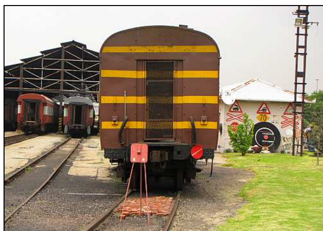
M06 – A stationary train properly protected with 'red flag' boards, indicating that the train is not to be shunted. The rule is that only the person who erected the board may take it away. The train was using mains electricity at the time.
