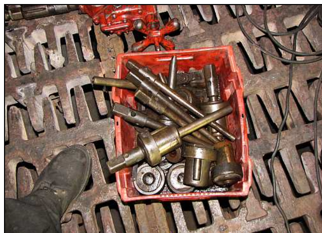
B08 – A box of assorted tube expanders and conical mandrels showing the different sizes. You can clearly see the inclined-axis rollers that tend to drive the expander inwards as well as imposing a tapering force onto the tube. It is the mandrel that sets the expansion plane of the rollers.
