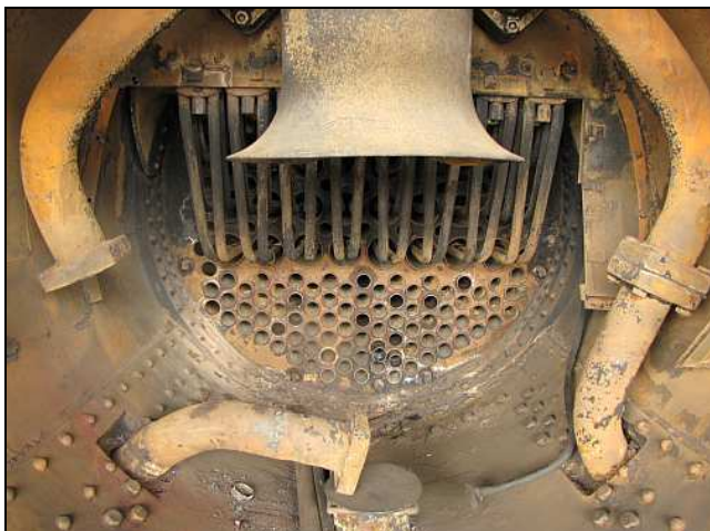
B01 – A view of Susie’s cute ‘little’ smokebox just before the boiler boys climbed in. Both of the steam down pipes would be removed by the end of the day and the blast pipe would remain safely capped. The thin grey-looking pipe to the right is the steam line for the blower. Can you spot the five visible washout plugs in the front tube plate?
