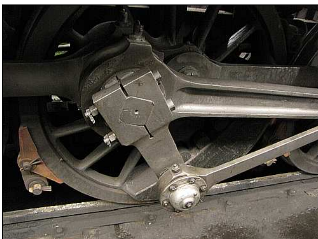
M09 – Monochrome Motion. A study of the RHS return crank on 15F No.3046, with a rusted cast iron brake shoe providing nearly the only colour. Note the cotter pins safely retaining the journal bolts, the bolts themselves routed through semi-circular slots in the square crank pin end.
