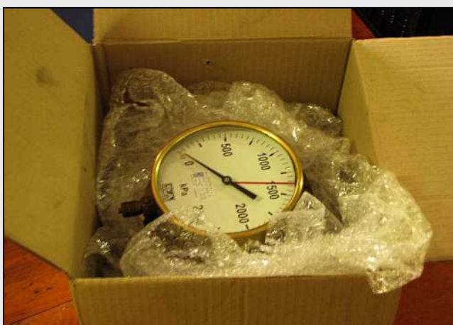
M05 – Fresh from the labs. A set of newly-calibrated boiler pressure gauges and duplex brake vacuum gauges arrived last week. These are for 15F 3046 'Janine' and 12AR 1535 'Susan' – the 15F already so fitted for the new season.
