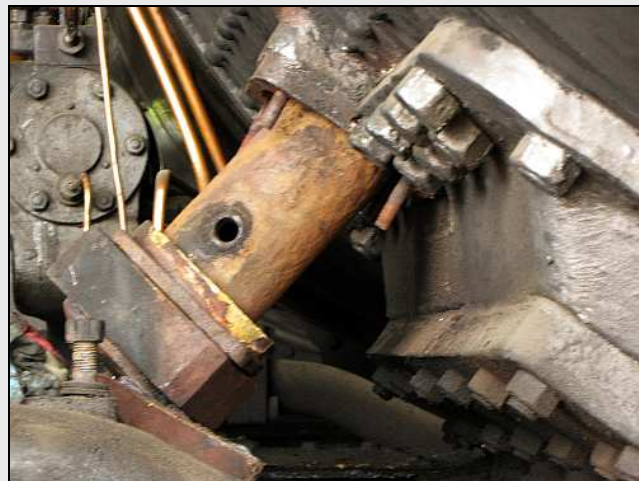
R08 – On a model steam engine, this is usually just a cute piece of threaded brass tube. The real pipe had been expanded within the flange and would need to be cut away. Note the detail of the 12AR’s composite smokebox saddle.
