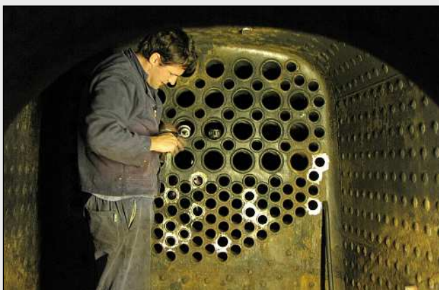
B03 – At the other end, Dawie is adjusting his vernier calliper. On the 12AR, the tube ends must protrude 8mm from the tube plate to get a proper rolled bead without interfering with adjacent tubes, or being too short to weld. As this tubeplate is slightly warped, each tube has to be individually measured and positioned to suit its location.
