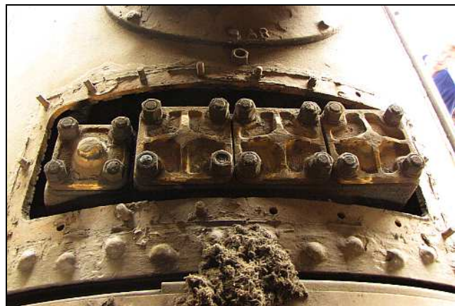
M02 – The exposed regulator chest on Susan the 12AR, waiting for the hydraulic boiler test. A quick test was done before the tubes were first removed, so the regulator's valves are already ground-in and sealed with silicone.
