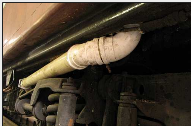
H06 – This is an experiment in using standard PVC pipework – note the awkward geometry to get past the frame and clear the bogie at the same time. The bracket at the far end is to be bolted to a welded extension bar – at a higher point to clear the bogie. If the experiment fails – the pipe can be removed again with no damage to the coach.
