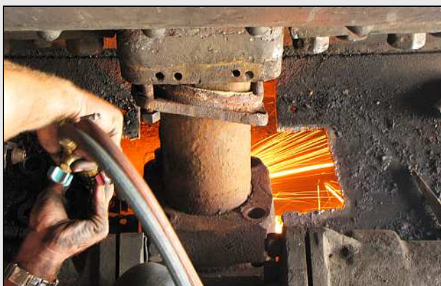
B09 – The last of the seized studs is getting some serious heat treatment to cut right through, before drifting the upper shank out. You can see by the extra access holes (for the collar ring) drilled into the smokebox's protruding boss that this pipe has been removed before, since the original boiler was replaced and this loco became a 12AR class. (The pipe is noticeably thinner than the opposite counterpart.)
