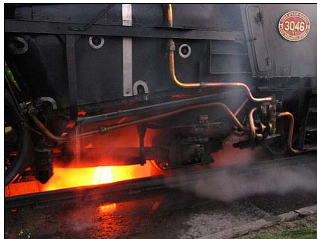
M16 – 15F No.3046 drops her fires on the third last trip of 2012. She will need to drop her fires for a while at the end of March 2013 for her three year boiler inspection. Thus, we are in a bit of a scramble to get 12AR 'Susan's' boiler going, including refabricating the front-end draft gear and replacing the steam down-pipes to the cylinders.
