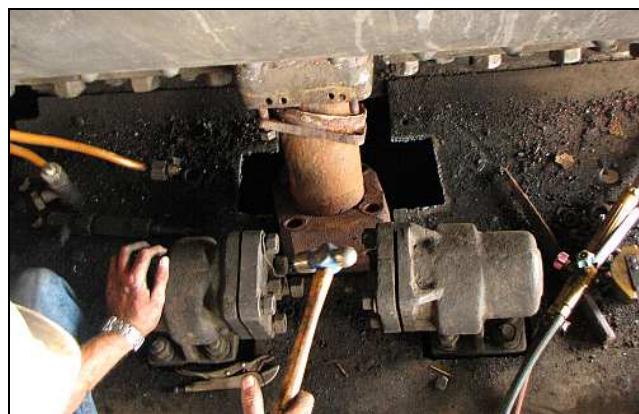
B10 – With all the rotating, a hole was found in the down pipe. The steam leak under the now cut-away pipe fairing had earlier been misdiagnosed as leaking vacuum breakers. (The down pipe fairing is in one piece with the steam chest cowlings on the old Hendrie-type engines.) Instead of repair, the valves pictured had been naughtily borrowed from the similar 12R 1947 'Rosie', but to no avail.
