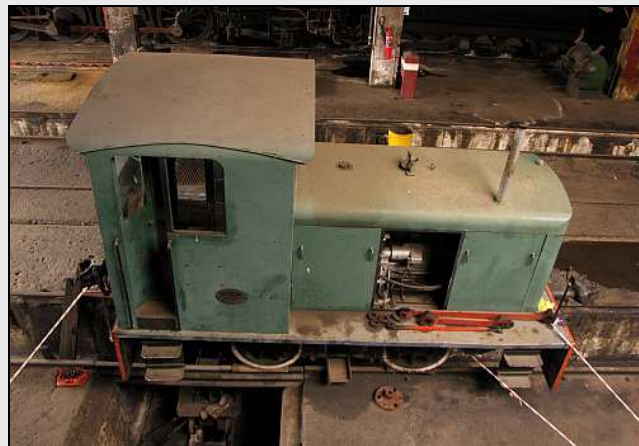
M18 – An increasingly dusty 'Andrew' is still waiting for his gearbox. Won't be too long now, as the new jackshaft gear has been cut and will be going for hardening before 25 Jan.
