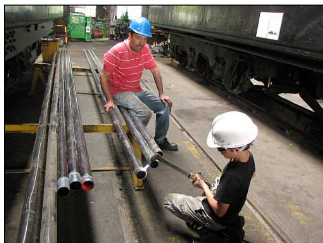
A06 – Big Daddy Waddy Wood Would (www!) be supervising the work and keeping the tubes rolling to spread the heat. Joshua got to learn about which part of the flame is hottest. Notice the center tube still glowing cherry red. (Photo un-retouched.)
