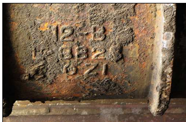
M06 – There has much been debate in the past to whether 12R No.1947 'Rosie' started life as a Class 12A or a 12B. The cylinder foundry marks show that she was a 'B.' (For 'Baldwin') When the loco is intact with cylinder cladding on, apart from the front bogie axle spacing being 2 inches longer, the original loco was visually identical to a 12A.
