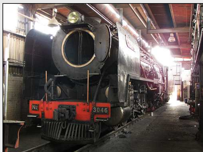
M04 – 15F No.3046 'Janine' rests cold with start-of-year smokebox cleaning in progress. (No trains booked this January.) She has exceeded her 4-month duty cycle and is well into overtime, but the old grinder has been running reliably while we await completion of the 12AR's repairs.
