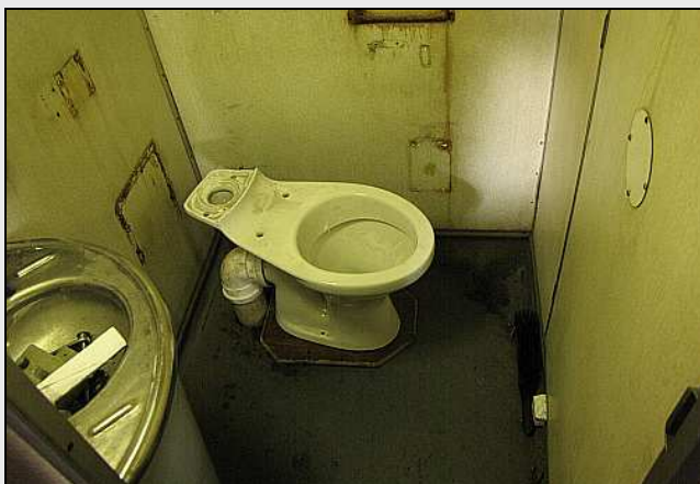
H03 – A domestic water-trapped porcelain toilet being fitted to Sandstone's Sleeper as a trial unit. This is one of two pans we had spare with a close-coupled cistern. (Future fittings will have remote tanks) It has been fitted loosely for future adjustment. Note the extra marine ply mounting pad.
