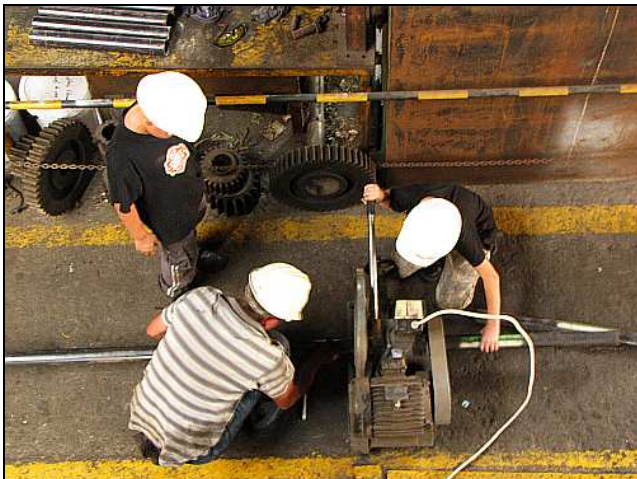
C09 – While setting up the boiler tube firmly in the clamp, Shaun teaches the youngsters the principle of cutting shy of the marked line to allow for a margin of error. Tubes protruding a bit too much at the front tubeplate can be always be ground back a little more after being expanded.
