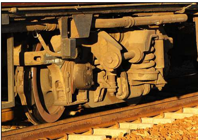
H05 – A sunlit commonwealth bogie, with a still intact land-power socket next to the jacking point. (Above the axle.) The drag link is angled for the track curvature too.
