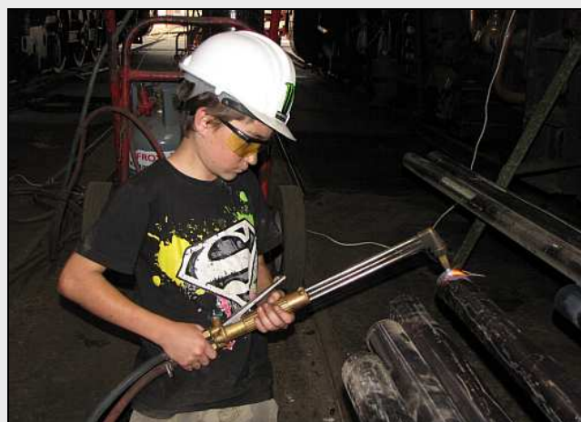
A04 – ‘Dad! You’re going too fast!’, he grumps. You can clearly see the streak of hot steel as the tube is being constantly turned. Josh was starting to hold the torch a bit too close at this point and the flames would soon star-out.
