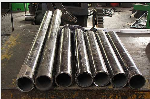
M05 – Neatly stowed cut-offs from the 12AR's new boiler tubes. A bit too heavy for use as wind chimes, we often keep them as rollers or for scrap steel, and the longer bits (Left) are useful as cheater pipes. However, workshop management is currently strict about discouraging the hoarding of steel scrap on a 'just in case' basis.
