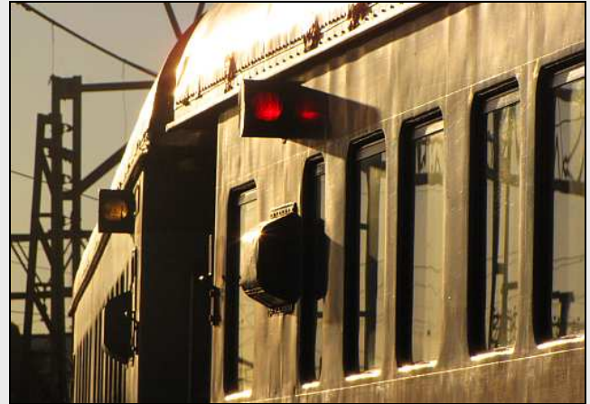
H02 – The wing-light lenses are beautifully backlit by the sun. They have sliding translucent-red plates behind their clear glass lenses. These two are functional but are usually unused as only the end-coach lights need to be illuminated.
