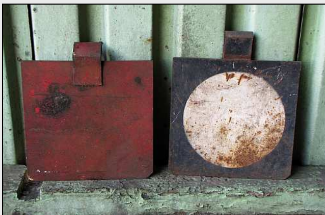
M11 – A matching pair of old wing-boards. Being daylight versions of wing-lights, they were used for goods trains without guards vans. The white-on-black target board reassures the driver that the tail vehicle is still on the train.
