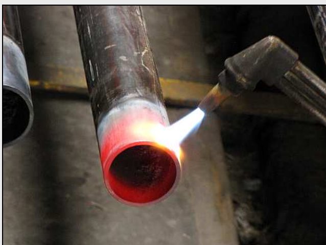
A05 – A close-up of the tube being annealed. The ends are softened by the slow cooling (Ductility), making them less liable to split when expanding them into the tube plate. It also homogenizes the metal – removing stress points. It also burns away any scale and the protective coating.
