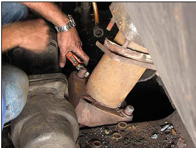
B07 – A hopeful tweak with the Bobbejaan (Baboon) Spanner actually got the front stud out, but there was no room to swing for the rears. And we weren't then up to taking the vacuum breakers off from the valve chests.
