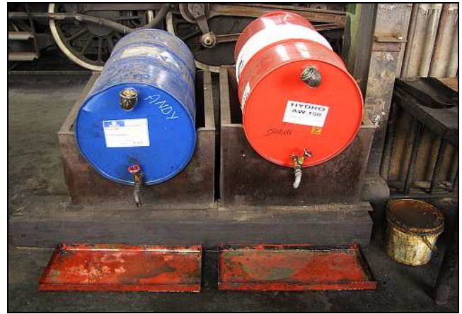
L08 – Oil on tap, with clean and empty drip trays and no sand on the floor, the way it should be. The oil drum labels can be a nuisance as they aren't always intuitive. Reefsteamers normally puts the steam oil on the left and the MH on the right.
