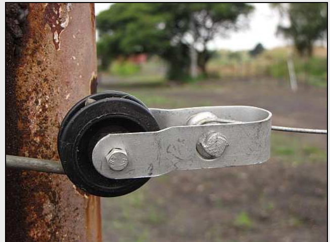
G16 – A close-up of one of the older-style turnbuckles, complete with a simple ratchet mechanism. We found the following day that once these have been fully tightened-up, there is no undoing that tensioned wire without cutting it.
