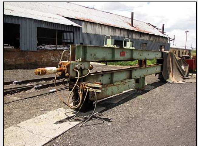
L10 – This is the Tube Swager that was rescued from the closed SANRASM site. This machine will be going next to No.8 bay (Where the Booth Rodley Crane is) and is to be restored to operation. Apart from the size of the machine, it was incorporated into the roof structure of the building it was in, which delayed its move. You can see the extra roof strut brace still present halfway along the tube channel.
