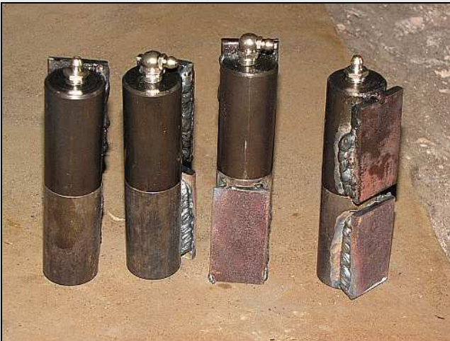
G09 – Here is a close up of the hinges that were 'nipped-up' the previous week by Aidan Mac Cee. They were pre-welded full length to mild-steel base plates by Gordon, with a TIG welder, for easier and stronger welding against the circular posts out in the field.
