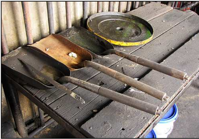
L07 – The inner bench of the oil store shows the broken coal shovels, which are used as spill-sand scoops while awaiting new handles for coal duty. The dustbin lid has been adopted as a spill tray for decanting oil bottles. Note the green colour of the compounded steam cylinder oil.
