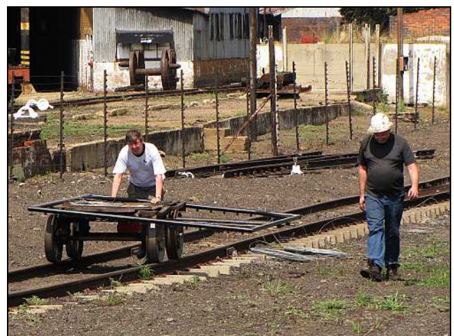
G18 – Nicholas (L) and Aidan trundle along to the western horizon with the first leaf of the new road vehicle gate and more work for the rest of us! The gate is actually balancing on extension poles shoved into the braces for the manual brake on this old man-powered rail inspection trolley.
