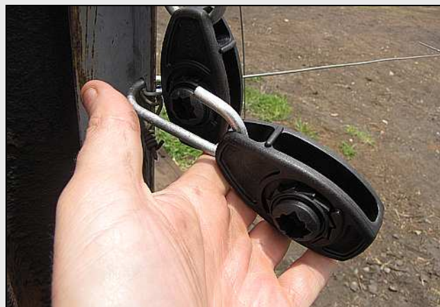
E04 – A cleverly designed ratchet turnbuckle which doesn't have a separate pawl. The barrel fits in a slotted hole and can move sideways. It uses the weight/tension of the wire itself to engage the ratchet cam into the integral pawl teeth.
