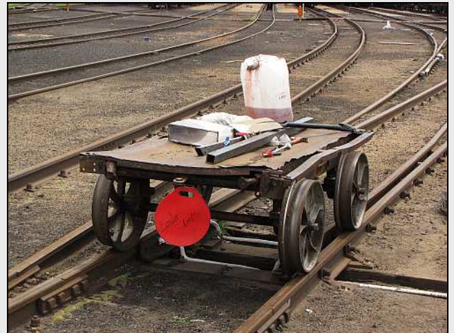
E08 – The gang were using the tea coaster as a supplies trolley. Since being used to transport concrete sleepers for the head shunt, those wheels are even more buckled. The hand writing on the red EOT marker says 'Boiler Empty.'
