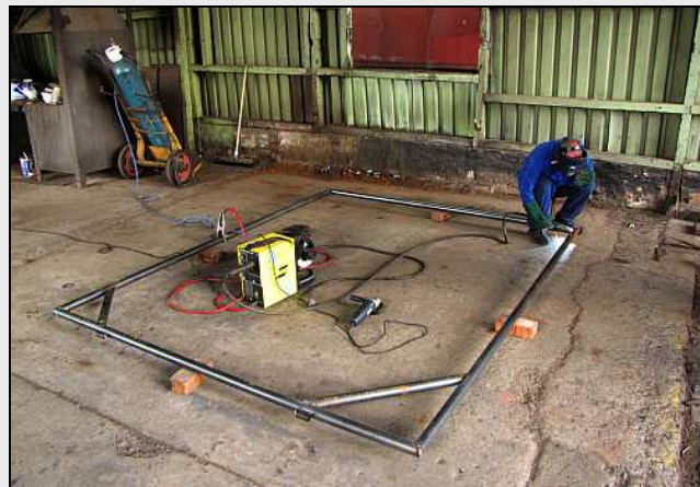
G20 – In the cavernous (and a tad cooler) forge, Gordon Bennett is busy doing the fill-in welding on the 3 rd new gate to be fabricated in two weeks. We had already recycled a pedestrian gate, and would be fitting another recycled pedestrian gate the next day and for the following week.
