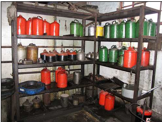
L09 – As befits a large depot, we still have a good collection of oil pots, including the half-height paraffin cans. Souvenir and train room décor hunters – keep out! The oil feeders themselves are assigned per footplate crew member and are not pooled. The 'mop head' in the top left corner is a bundle of spare wicks for the multitude of oil cellars in the vicinity.
