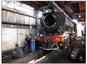
W04 – 12AR No.1535 'Susan' was reported to be blowing within the smoke box with the regulator open. The problem turned out to be a perforated superheater element. Unfortunately, it was in the top row so the three elements below had to be taken out as well. Conveniently, the smokebox front plate did not have to be removed.
