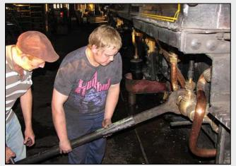
W05 – The 12AR's left injector was running poorly, picking up hesitantly and only in the rear quadrant. The crew were struggling to keep the water level up in the hardest parts of the route. The injector was partially dismantled on 29 April and we found that the steam cones hadn't been replaced as they should have been in 2012. Luckily, the new cones were found stashed away in the brass store and refitted.
