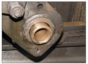
W07 – Class 15F No.3046 has had the front end of her left valve motion stripped due to excessive wear. Pictured is the eccentric bush that forms the bearing between the eccentric rod and the expansion link When the locomotive was recommisioned 3 years ago, these bearings were incorrectly made from plain old brass instead of the proper phosphor bronze and they have worn badly in service. You can see the outer wear gap even in the reduced photo.
