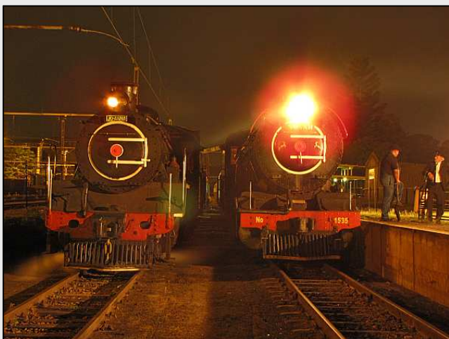
P47 – A front view of the old girls standing calmly side by side and happily submitting to being the focus of attention. The differences in the pitches of the individual boilers is obvious in this shot.
