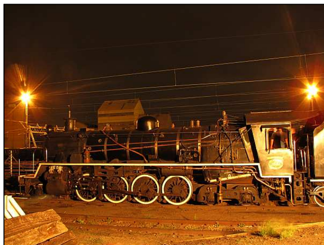
P48 – The 24 Class eases forward and I caught her in her funny-wheeled entirety in the slot between the platform and the storage tracks. Coming from a depot stuffed to the soot-crusted rafters with 4-8-2 'Mountains', the 2-8-4 'Berkshire' arrangement always looks a bit lop-sided to me.
