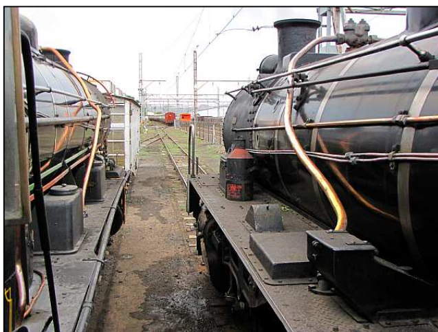
P36 – A driver's eye view down between the two locomotives at the end of the photo shoot. I found the differences in the sandboxes to be interesting. The odd thing is Reefsteamers has found that the more old fashioned loose-mounted cookie-jar style lids on the 12AR are the best design for keeping the traction sand dry.
