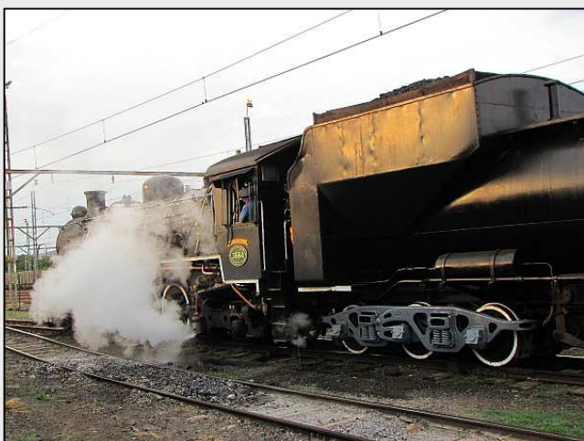
P35 – Even a 24 Class can look good sometimes! Here, the smartly turned out engine and tender is the backdrop for a slightly-opened demonstration blow down.
