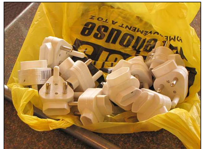
P24 – The little details that help. Each compartment was provided with a two-pin adapter to ease the charging of cell phones and cameras. Luckily the familiar CEE7/16 two-pin design is also used in both Switzerland and England from whence most of our guests came.
