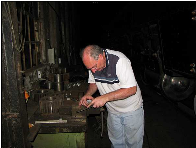
P43 – One of the electrical phases had gone down, which meant no lights in the 15M shop – just IDEAL for last minute prep. Undaunted, Aidan is seen using a file to dress the square shank of a bathroom door handle.
