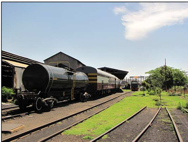
P11 – Resting on the old washout station approach tracks, the Staff and Baggage Van had been coupled up to the drinking water tanker and most of the loading of service items already done by today. A freezer would be changed out for a larger capacity unit and sundry items loaded.
