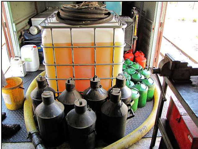
P13 – Some of the kit with traction sand and oil bottles on board. There was about 900 litres of diesel in that tank, with 500 litres already loaded into the John Deere Genny's tank. The diesel ran out 1 ½ days before the tour ended with the original estimate being 100 litres burned per day.
