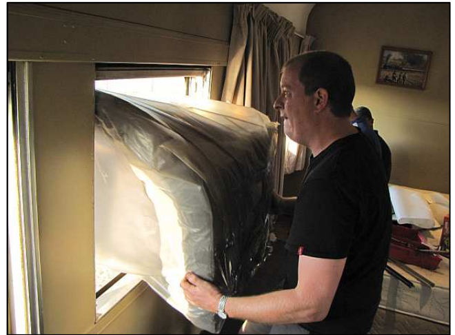
P20 – This meant that every gold and silver compartment needed to have one window pane removed before the chairs could be loaded. That caused some extra cursing but with typical RS stubbornness, the job was completed.
