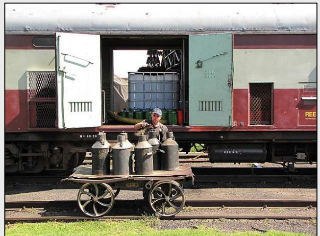
P12 – A one-Jeandre-powered wagon had made its way to the S&B van, with nine bottles of fresh loco traction sand on board. We don't normally use these bottles, so they were a bit rusty and encrusted with old sand. Before being loaded, the bottles were given a quick cleaning with a stiff brush.
