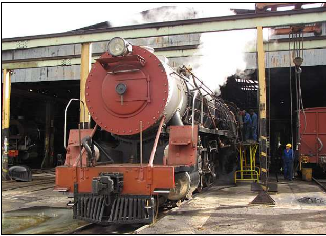
P01 - After over a decade of storage in an incomplete condition, Class 15F No.3046 had the remaining boiler and backhead fittings mounted, and then underwent boiler testing on 9 th April 2010. It was the first time that this locomotive had been in steam since 1992 (18 years) and 22 years since the locomotive was retired from then-Spoornet service. (The retired but still-intact locomotive underwent 4 years of annual boiler testing as a reserve.) The RHS picture shows a view of the newly primered coal tender and a view of the Archimedean screw for the mechanical stoker.
