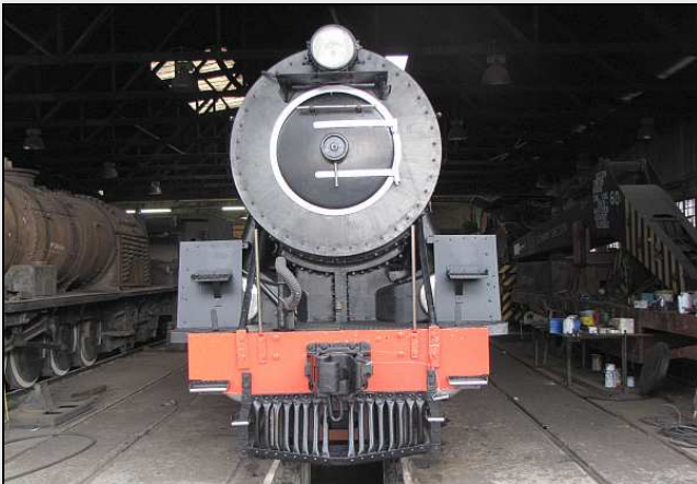
P02 - With smokebox newly painted in black etching primer instead of the traditional graphite, on 1st May 2010, Class 15F No.3046 was waiting for her smoke deflectors, as well as some final stoker, reverser and injector repairs.
