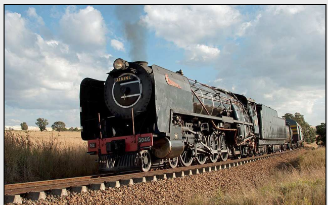
P17 - Reefsteamers normally runs their locomotives for a four-month duty cycle. (About 8 x 190km trips). Due to lack of alternative motive power in 2011/2012, this marvellous machine has been running all of our trips for just over a year. As of end March 2013, 15F No.3046 will be staged for a new 3-year boiler ticket. (Pic by A. McCarthy)
