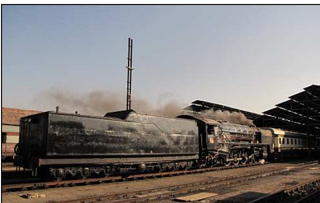
P16 - On a Saturday shunt at the Germiston Steam Loco Depot, which is preserved by Reefsteamers, Class 15F No.3046 is moving long-distance touring coaches. You can clearly see the massive ex-Class 23 Type-EW tender that many Class 15Fs inherited when the Class 23s were retired en-masse due to metal fatigue cracks in their frames.
