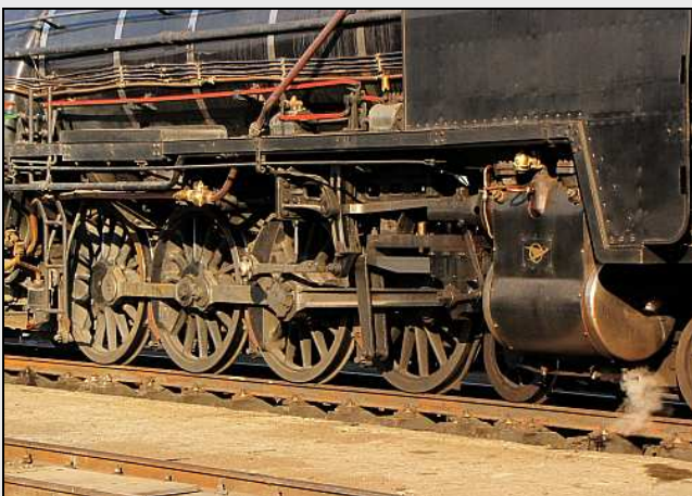
P14 - The Class 15F was based on the previous successful Class 15E, but with conventional Walschaerts valve gear. Although an older design, they proved to be rugged machines with easily maintained valve gear. 255 examples were built, becoming the most numerous class on the SAR.
