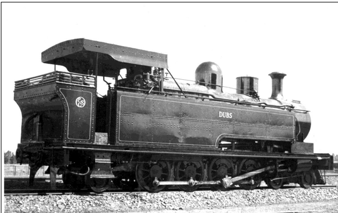
Dubs A of Escom in about 1949. 100 of these locomotives were built for Natal Government Railway, between 1888 and 1900. Umgeni Steam Railway has a Dubs A, which is under restoration.
