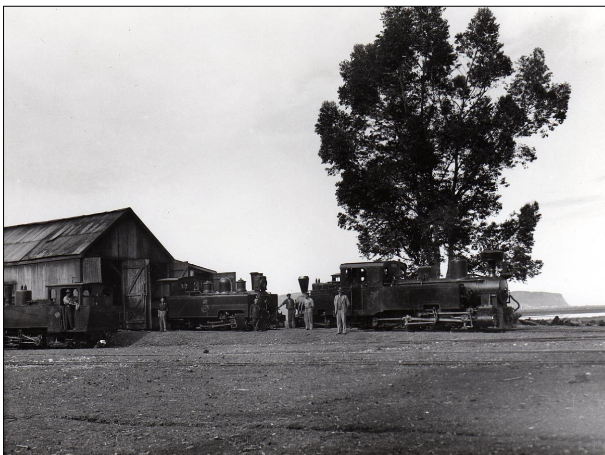
Scene at the loco shed of the South Western Railway, Knysna. Knysna heads are visible in the background. Locomotives are, from left to right, SWR No. 1, O & K No. 1175/1906, SWR No. 2, O & K No. 2240/1907, SWR No. 3, O & K No. 4880/1907 and SWR No. 4, Hawthorn and Leslie & Co. No. 2687, ex SAR class NG3, No. 4. The O & K locomotives were wood burners, while the H & L locomotive ran on coal.
