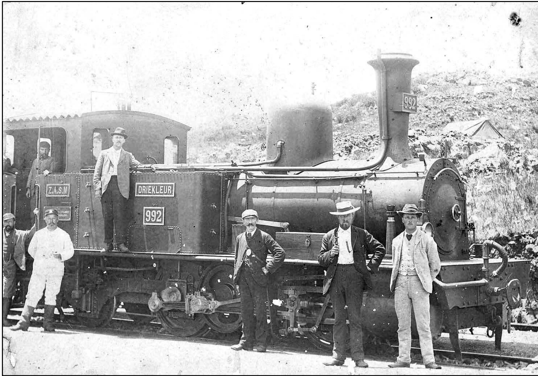
NZASM Rack loco No. 992, Driekleur, built by Emil Kessler, in 1894, works number 2643. A total of four of these locos were built and they remained in service, on the Waterval Bo to Waterval Onder section, until 1908, when a new route, with easier grades, was opened.
