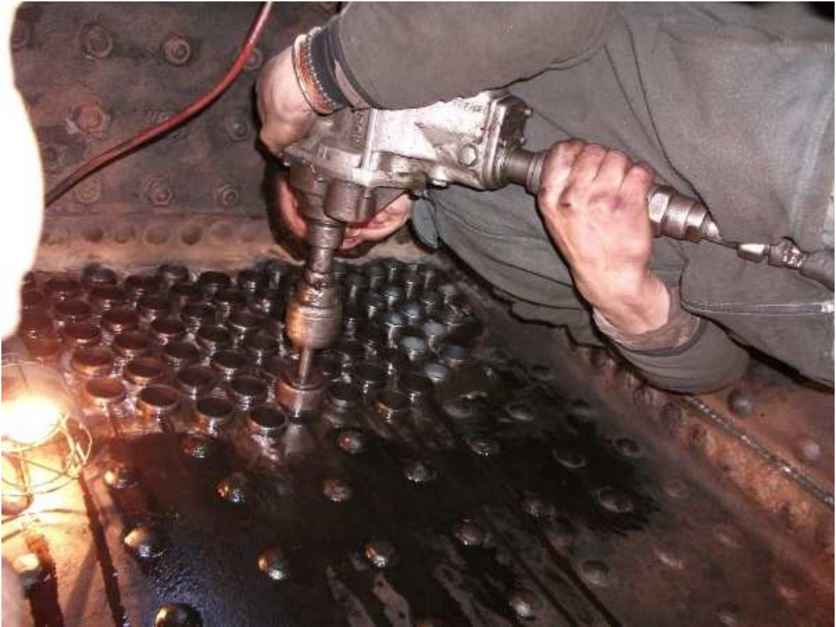
Expanding tubes firebox end
