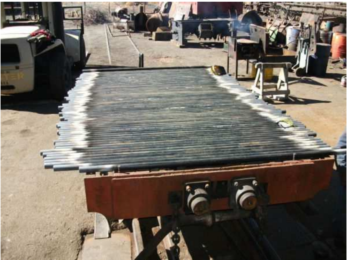
Annealed boiler tubes ready to use.
