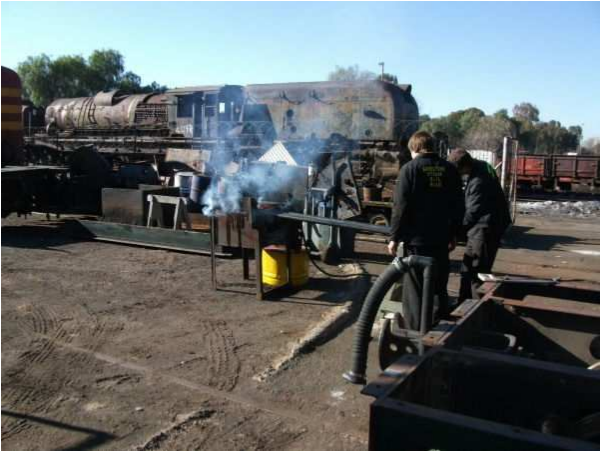
Diesel fire use to anneal the Lawley locomotive tube ends.
