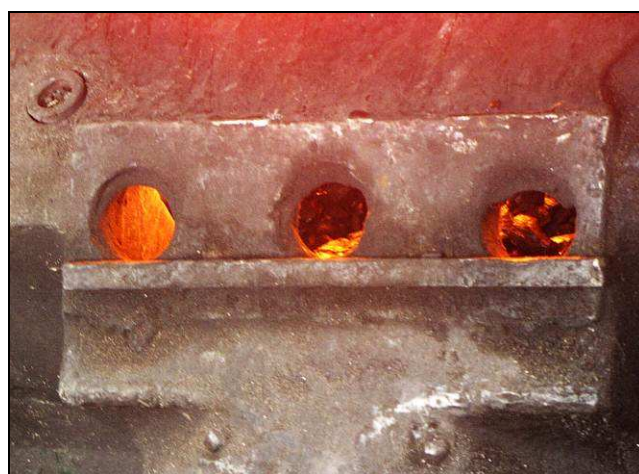
C06 – A new charge of coal has taken up nicely, visible through the inspection ports on the spreader table’s atrium. There is often a bolt placed in one of these to temporarily change the spread without having to adjust the steam jets.
