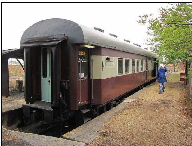
T17 – The Staff and Baggage van, type GD-1 and one of only 20 made and the only one currently serving in preservation, stands duty in the coal dock as a stand-by generator for the 15M shops.
