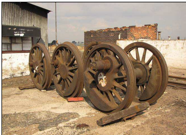
T13 – The axle packing project of a few weeks ago, now seen in daylight. There is still a fourth axle (and two front bogie axles) on a service track within the Running Shed. The area behind is the old sand bunker, although we draw our traction sand from a pile of white builder's sand stored and kept dry within the covered Forge House.
