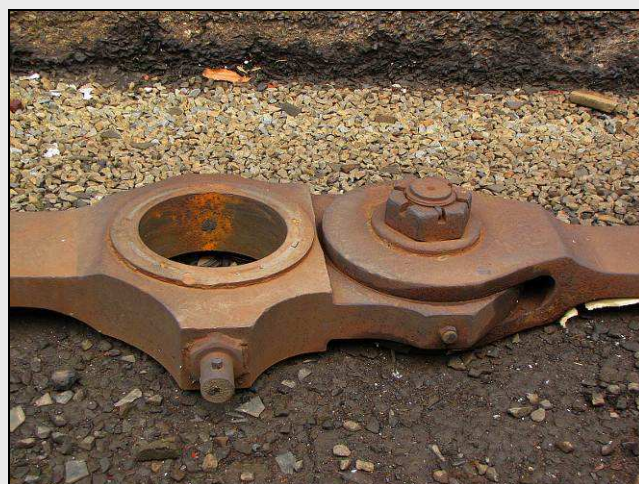
T10 – A pair of newly-revealed coupling rod knuckles – dumped aside and long-hidden on the normally occupied siding. Note the sharp profile between the pin boss and the tongue – not great engineering but seems to have worked!
