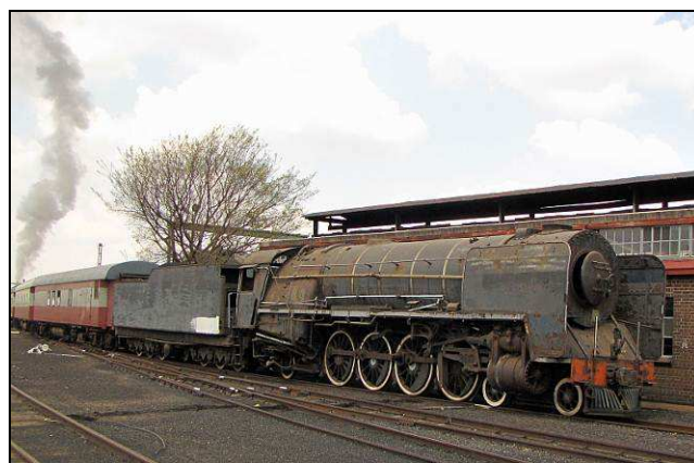
S16 – Although looking pretty knackered, 15F No.3135 is known to have a fairly good boiler and could be a candidate for future restoration, once we get some smaller engines running. We were using the coaches as handles to reach into those sidings and spread the weight out a bit, rather than have two heavy locomotives coupled together
