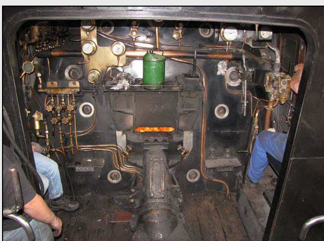
C05 – A more general view of a rather sooty 15F cab. You can see the effects of a blower-less ‘opsteek’ in two sooty updraft streaks on the regulator cross-shaft, the blackened stoker jet gauge and a nicely blackened lubricator.
