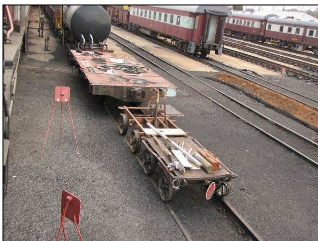
T09 – The tea trolley and a pair of coasters. These are surprisingly useful around the yard. The middle coaster is actually a man-powered pump wagon sans the lever and ratchet. However, it still has the reduction and axle gears.
