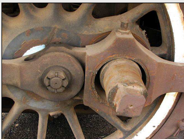
T11 – The same components on 15F No.3135 – hangin' a bit loose without the bronze bushings. A loco being shunted like this makes a metallic gritty hissing sound. This coupling rod was still attached to the other wheels though, so no danger of it dropping off from the shunt!
