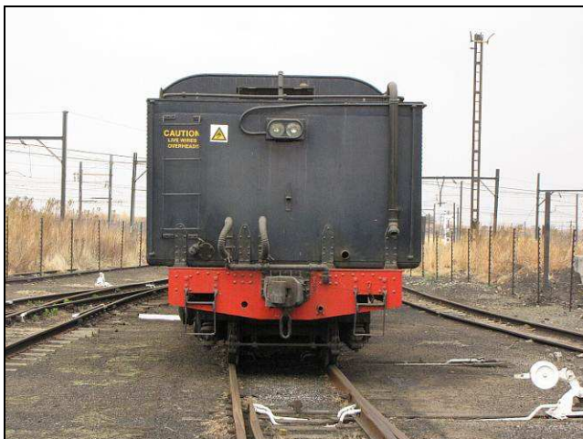
S13 – Just to freak out our overseas friends with their boring 4ft 8½ inch gauge sledge-irons, how's this for a classic Cape Gauge overhang shot? Notice the point blade stretchers are painted white. The theory is that it makes it easy to see if they have broken or have been removed.
