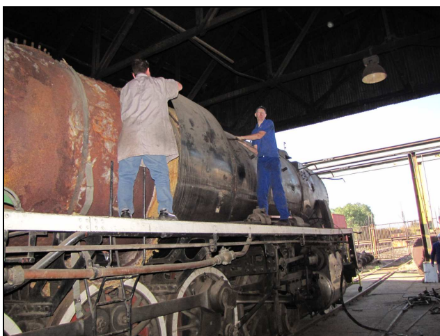
P18 - The plates on the right side of the locomotive came off a lot easier as the welds had been removed. But the front two plates still needed to be winched to get over the obstruction presented by the reverser.
