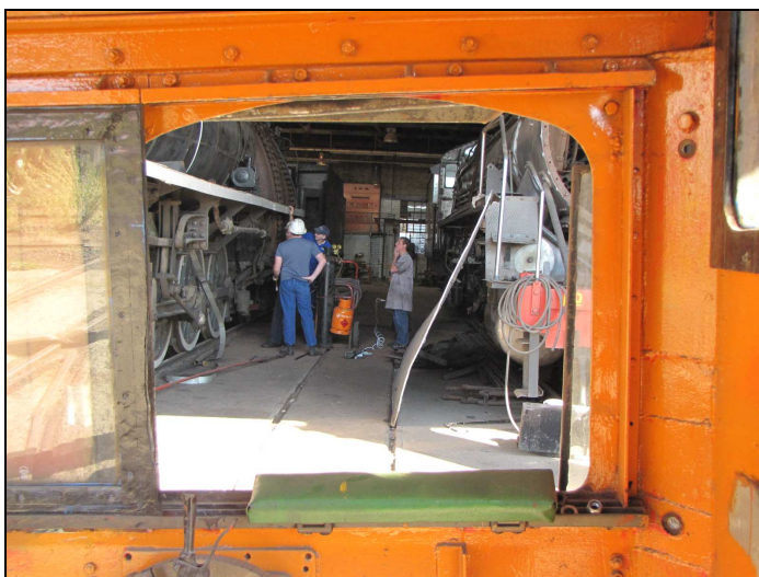
P02 - At the start of the job, after stripping the fire arch and the grates for inspection, the cab had to be removed to provide access to the firebox's corner. Here, seen through the driver's window of the disembodied cab, the strip-down gang is planning their first angle of attack. (Which would be the firebox throat plate covers – Aidan McCarthy had already exposed the firebox's tapered flanks during the previous weeks.)
