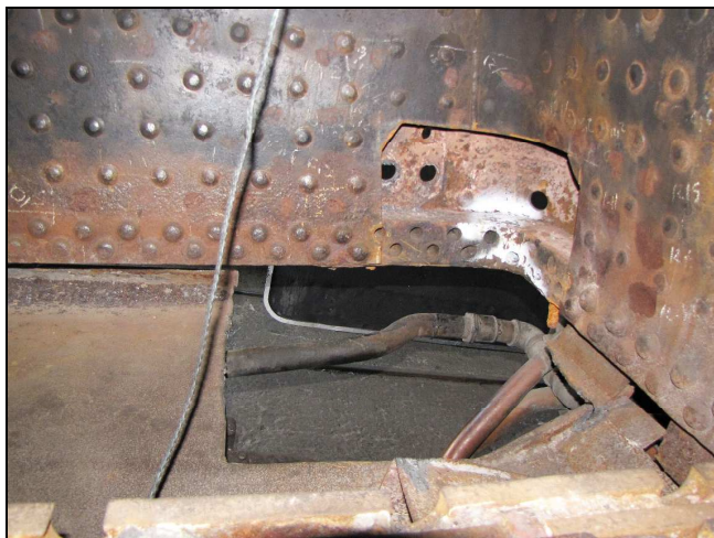
B07 - A more general view of the repair area in the firebox corner, showing the cut out in the underlying ash pan hopper. Admittedly, it was a somewhat brutal way to do the work, but it has really eased access, especially if only one person is working on the job at a time.
