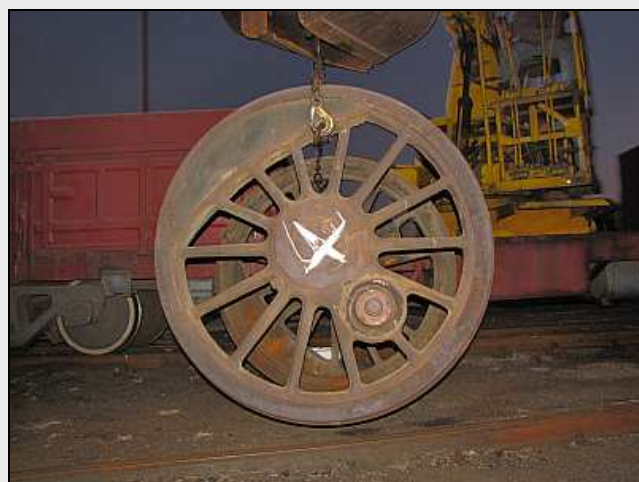
W12 – Wheels aloft! (2 nd axle) Robbie had to slew the grab in discrete steps to avoid the load swaying at the end of the swing. He also kept the load as close to the ground as possible, in case the grab wagon started to overbalance. Yes, we did some top-soil ploughing with these wheels!
