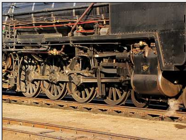
U04 – Wheels of Steel at front-dead-center. Notice that the curved expansion link is vertical. (She is also a hair off mid gear.) That vertical position is one of the check points for valve gear geometry when building a model live steamer.
