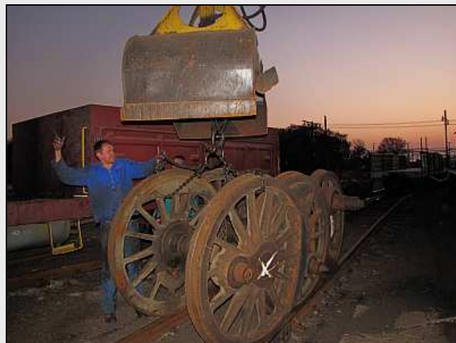
W08 – With a standard, twirling, upward pointing finger, Dr. Smudge signals Robbie to take the first lift. He is also very carefully holding the spider hooks in engagement without getting his fingers nipped in between loading surfaces.
