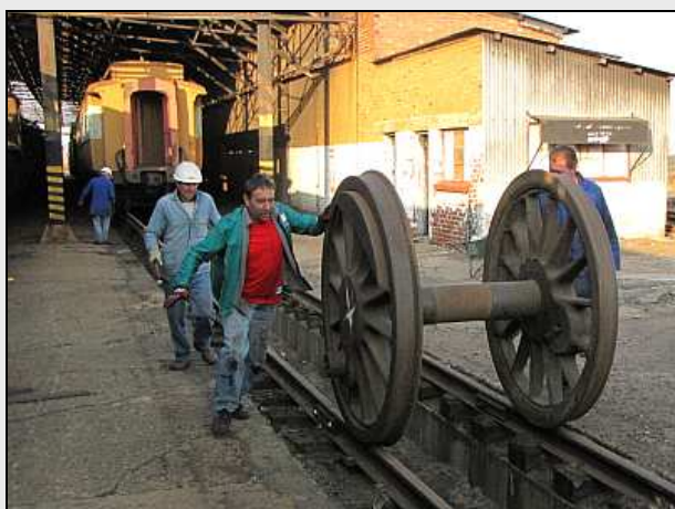
W05 – While rolling the last set, the fellows changed their minds about the slinging and decided to instead place the axles on the concrete slab in the background. But they needed to clear the pits because of the hoisting involved.
