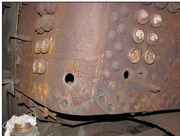
B02 - The exterior of the firebox corner that is under repair. All the truncated and offset rivets have been removed from the foundation ring and stay holes respectively. The holes just need their burrs reaming out and they are ready to go.
