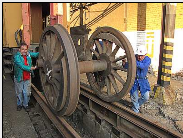
W04 – The last of the three axles at this end of the coach are moved. You can clearly see the 90 degree orientation of the crank pins. But you will also notice that the counterweights are not symmetrical to the crank pins.
