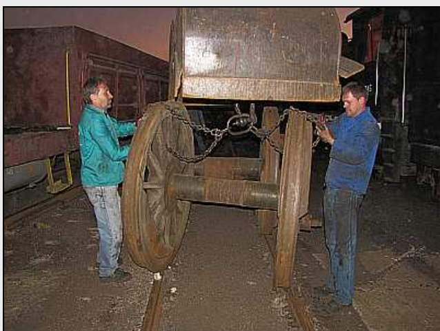
W09 – A picture taken later for the 2 nd axle shows the very useful octopus-chain that we were using as a two-hook lift with the hooks interlocking in pairs on either side. It also provided flexibility for the axles to find their own balance.
