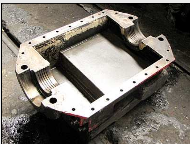
H05 – The lowest enclosure, with an integral sump and oil pan, is now miraculously free from silver-coloured sludge. Note the labyrinth seals for the jackshaft bearings.
