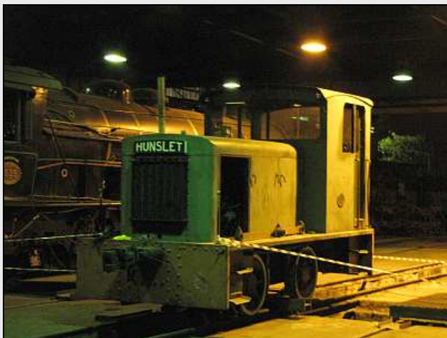
H01 – Still awaiting quotes for the required jackshaft repairs, 'Andrew' the Hunslet remains balanced on an I-beam for gearbox replacement. Notice that the removable bridge rails have been re-inserted under the rear wheels.
