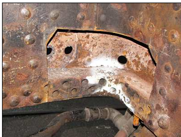
B06 - Here is the cut-out area in the firebox's lower corner, with the newly welded foundation ring as marked for crack detection. The new patch needs to be very carefully cut and dressed to custom-fit this hole as closely as possible.
