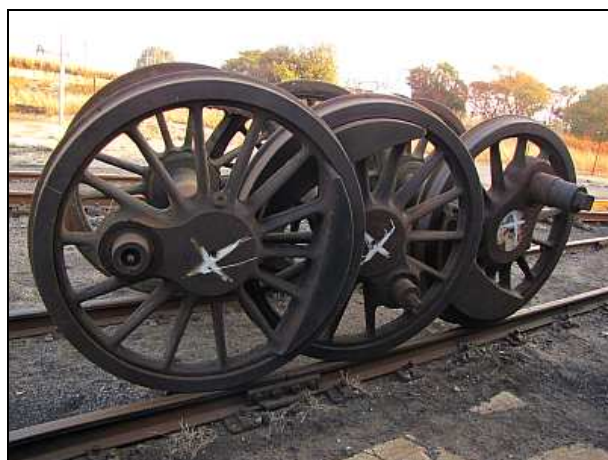
W06 – Scotches rule! How's this for a compact 0-6-0 wheelbase? Once the first and second set were scotched, the heavier driving axle was allowed to roll back. The axles telescoped together but still managed to stay on the rails!
