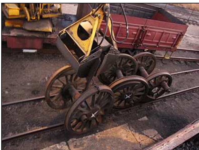
W11 – Perhaps the trickiest part of the operation would be the initial lift with the weighty load swinging to find its own center. The grab and boom gear was operating at close to capacity and the hard-to-modulate valves would cause the load to pendulum. Everyone is standing safely clear!
