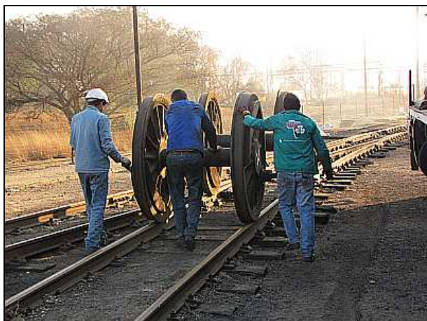
W03 – The game plan was to shunt the wheels out with a loose cable sling around the axles and tied to a coupler. Alan (Left) has a scotch to retain the wheels on the slope. The further axle is the heaviest, being the main driver.
