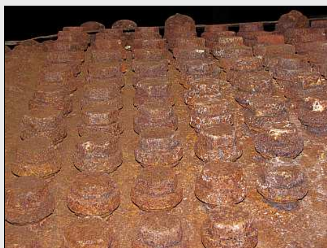
B12 - These caps will also need to be de-rusted and painted - it is gonna be a nasty job with all of those crevices and valleys! But we'll do this AFTER the boiler tests, as the primer coat may mask small gravity-fed leaks.
