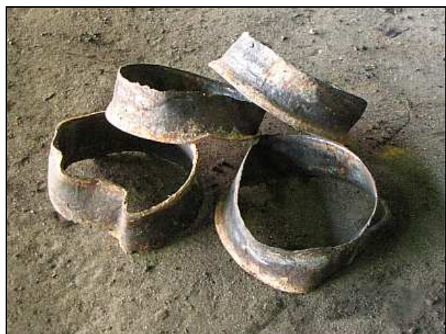
T05 – These are the crushed remains of old copper ferrules, which are used to seal the rear ends of the tubes at the firebox end. You can see that they protruded from the tubeplate when those old tubes were originally installed.
