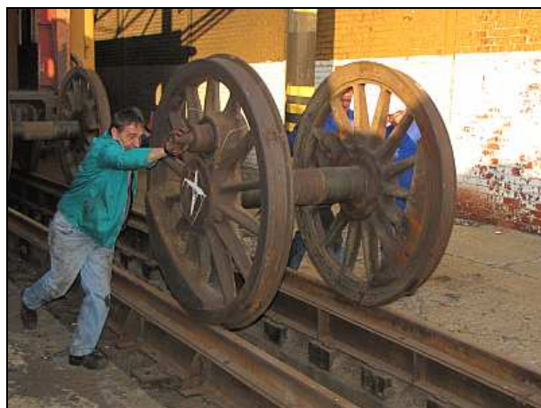
W02 – Two people moving a multi-ton wheel set uphill shows the foundational principle upon which all railways depend – the matching track and wheels are there to consistently reduce friction, as well as providing guidance.
