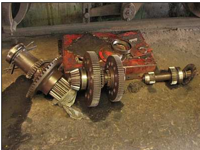
H03 – A selection of shafts. Left is the old reversing shaft (With one bevel gear previously removed and oil dippers added) ; center is the two-speed counter shaft + dog clutch set ; right is the input shaft with a fixed two-pinion cluster.
