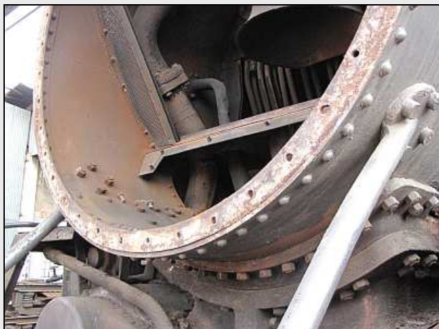
B01 – A poor quality accident repair. Not only is the front cover plate distorted, but the smokebox's replacement barrel had been rolled skew. You can see how the lower flange protrudes. It is recessed again along the center line.
