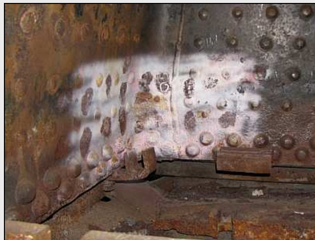
B08 - By contrast, here is the opposite (LHS) corner in its original state. It has also been painted and dye-tested for cracks. (These are the known vulnerable spots in a Class 15F locomotive's firebox) Note the welded seam, and the foot brackets that support the fire grate runner rails.
