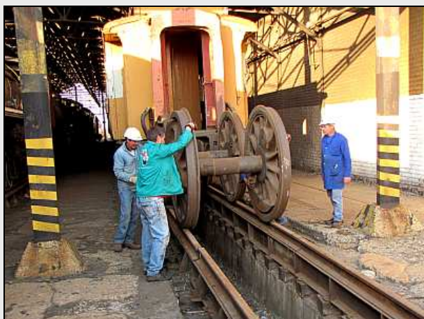
W01 – During the yard clean-up project, a spare set of 15F driver axles needed to be moved to allow access to this wooden-bodied coach. The tread beams are a bit weak here, so we were reluctant to bring a heavy locomotive in.
