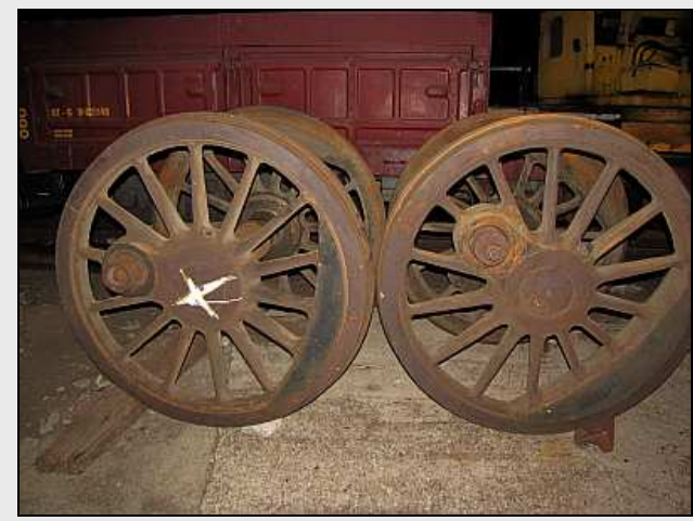
W16 – Efficiency! Two axles safely 'scotched' and out of the way of our rails on a previously unused slab of concrete. It also means that the wheels won't sink into the soil under their weight over time – especially after a good thunderstorm. I always find the skinny spokes remarkable!
