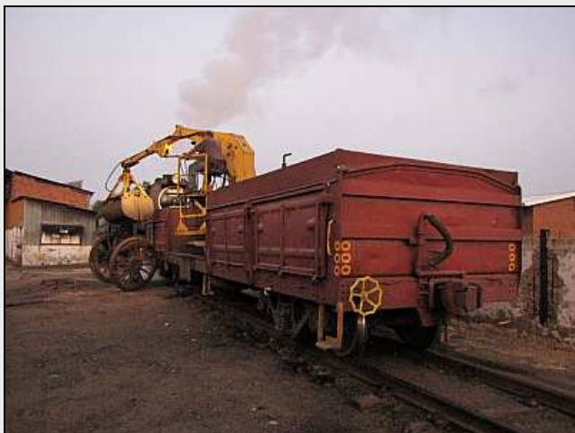
W13 – With the wheels safely snugged in against the grab wagon (without too much bashing) the whole lot is shunted backwards to get the side-slung wheels onto the concrete slab in the background. That is 15F No.3046 in the shot.
