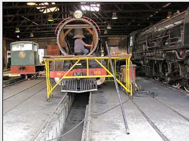
T02 – A front view of the work area. The visible boiler tube is the No.8 tube that cannot be fitted until a built-up hole in the rear tube plate has been checked by the boiler inspector, and permitted to be used, repaired or patched.
