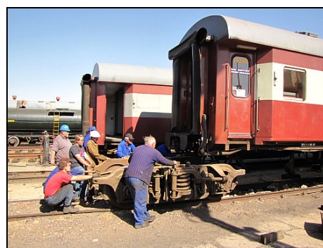
The donor bogie rolls in a bit too fast – notice the two human brake shoes doing their best to dissipate momentum!
