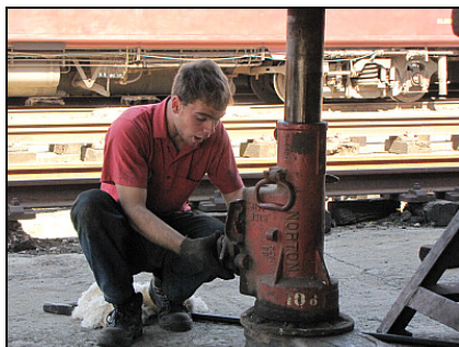
Jacked up, ek se! Jeandre looks a bit startled, but he is actually confirming instructions in terms of coordinating the heights of the jacks on either side.
