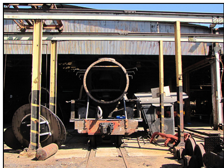
Class 15F 2914 joins the 'faceless brigade! You can see the uneven putty (light brown) from this distance away! No wonder she had no induced draft from the front end!
