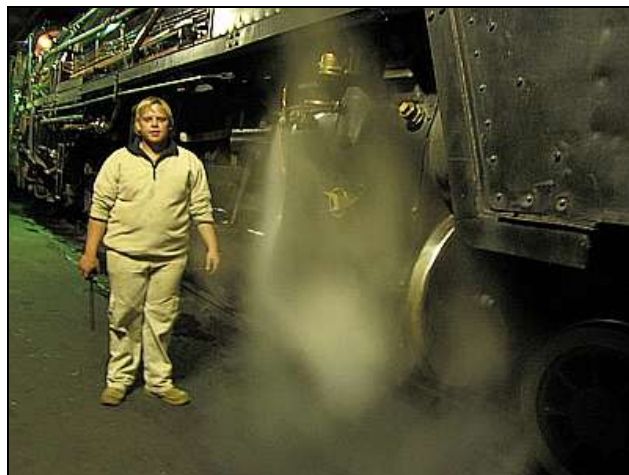
S02 – A Mienie Blow Down. Although not strictly required for every run, some of us bake-heads are getting into the habit of opening the lubrication line chokes and blowing out the oil lines well in time before the morning preparation.
