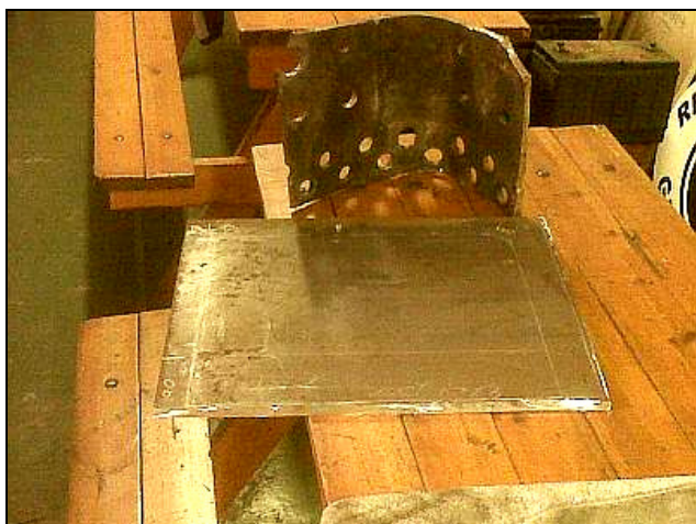
F03 – The old and new firebox inner corner plates waiting in the workshop canteen. The currently oversized patch will need to be hot-rolled to get that curvature right without cracking.
