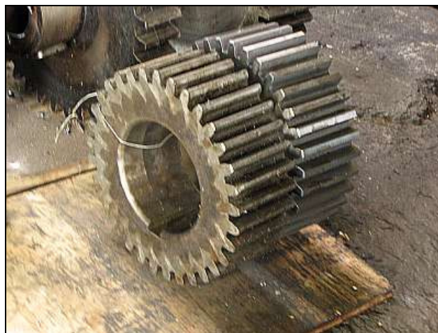
M04 – Although a certain clapped-out old 15F is hogging most of the limelight with her dramatic repairs, the depot wheel lathe rebuilding project is still going on quietly in the background. New gears are still being cut one-by-one and new keys are being manufactured for the freshly skimmed shafts.
