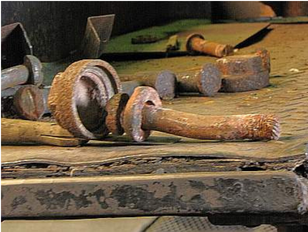
F07 – This old flexible stay put up a good fight. You can see the washer which provides the flexibility for the head, whereas the screwed-on cap provides the actual pressure seal. This stay rod got bent while being hammered out.
