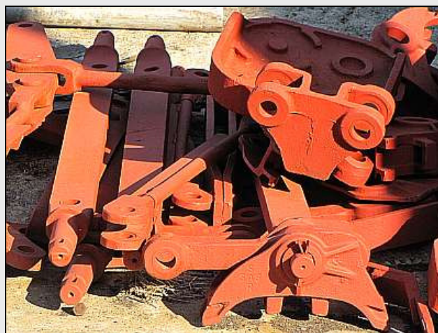
M06 – Rhapsody in red ... a pile of brake beams, pull rods, relay rods, and a spring bracket await re-assembly.
