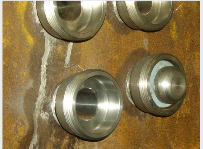
F08 – For comparison, here are some new flexible stay seats recently made and fitted to Umgeni Steam Railway's Class 19D. Note that one has already had the stay rod inserted and tightened. (Pic. by Edwin Andy Anderson.)
