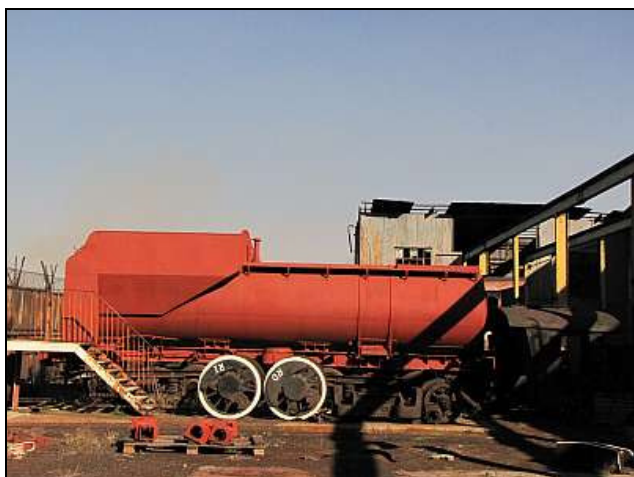
M05 – Trying out a flangeless pair of 14R drivers for fit on a oxide primed vandy tender? Back to the drawing board!
