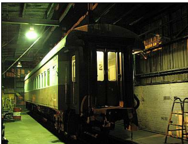
C15 – Coach No 28332 takes on a different look at night with the interior lights energized from a land-power line. With the elimination of the original inverters, the lights actually draw less current than they originally did, making hooks ups easier.
