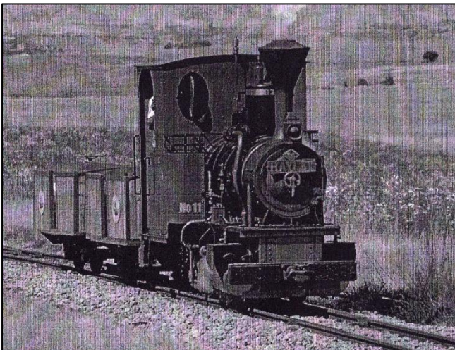
0-4-0T loco with inside frames, of the Sranger – Kearsney Light Railway; gauge 2ft.
