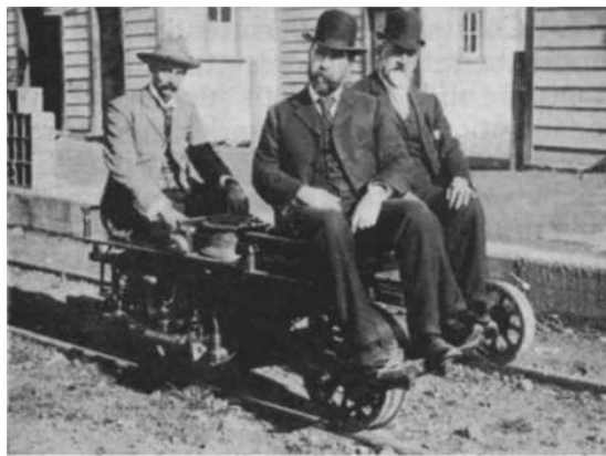
One of the first motor jiggers introduced on the N.Z.R. The snap was taken at Mercer, about 1902, and shows (at back) Mr. C. Holm Biss, District Engineer, and front (left) Mr. H. Buxton, District Traffic Manager, and Mr. H. J. Jones, Stationmaster.
