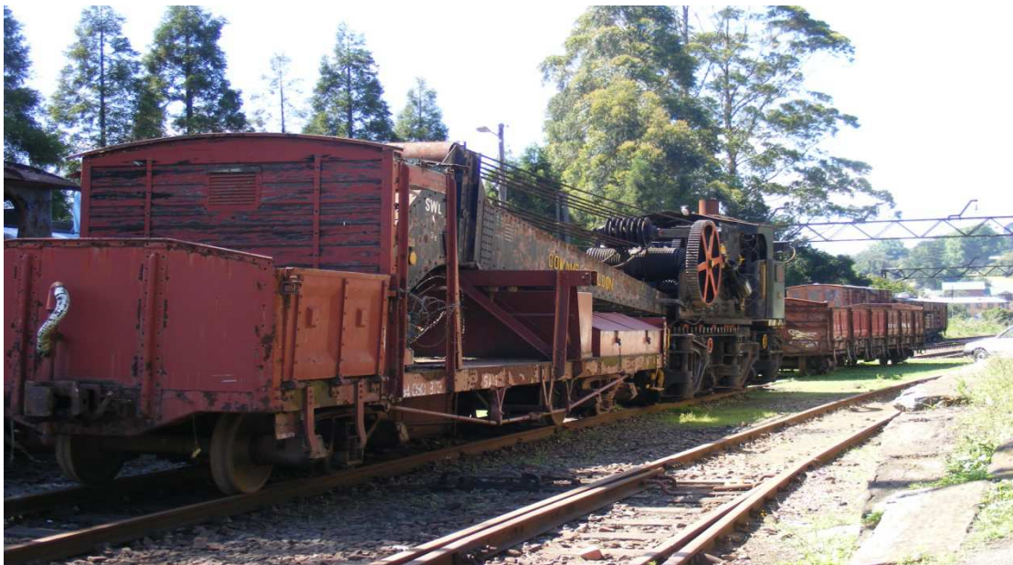
THE COWANS SHELDON CRANE 184 WHICH HAS BOILER CERTIFICATE
