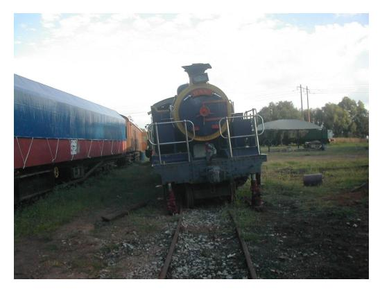
Pics above are of the jacks, which have a 50 ton capacity and 14" lift, and the North British tank jacked up. I had hoped that we could rerail the front bogie but it doesn't want to know. If you get the front bogie wheels on the rear ones derail and vice versa. As it's going out by crane I intend to leave it where it is and lift it from where it stands.
