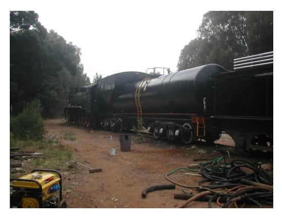
Three pics above are of the Wardale modified 19D, We've done one side and top of the tender, a long job as there is a lot of flaking paint and surface rust. We'll carry on and finish the repainting as this is a well known loco and it will be good to show it off properly.
