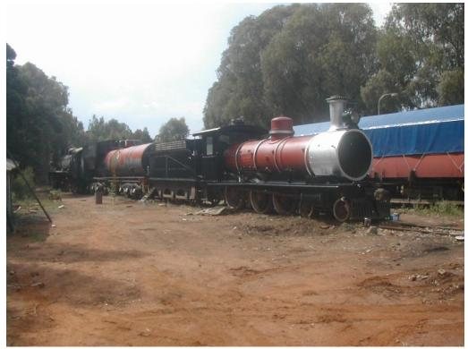
Above 6 Class 473 before and after. We did complete boiler, cab and tender, looks pretty smart now. The smoke box front and smokebox door are missing, we have a door, pin and mountings, will need to fabricate a new smokebox front. With all these we haven't done below the running plate or inside the cab as there is a lot of grease around and we don't have sufficient water supply for a pressure washer.
