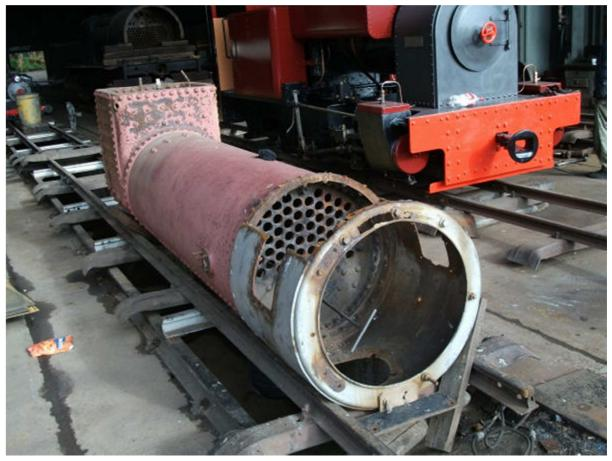
The photographs show the locomotive in its fully disassembled state. Indications are that the boiler is repairable. We do not have any technical information on this locomotive and would appreciate photographs of these locomotives in use, drawings etc.
