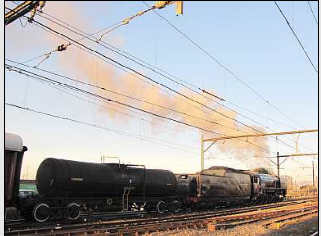
P42 – The great length of this traction combination is apparent in this run-by. The 'Spoories' call these 'Torpedo Tanks' although the term originally came from the circular-section tank drum of the Vanderbilt type tender.
