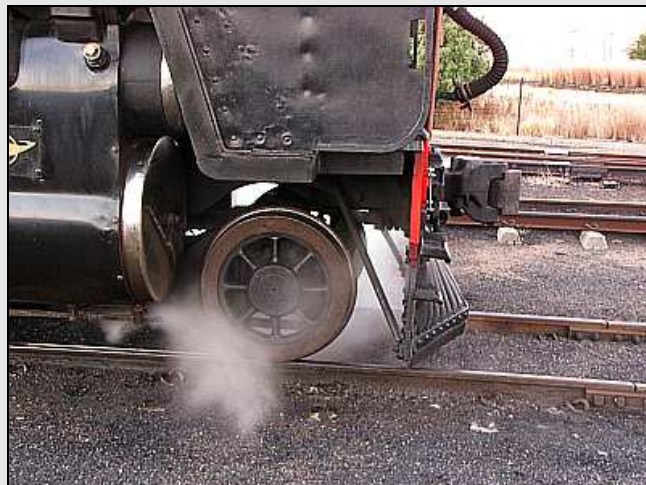
P30 – Being Cape Gaugers, there naturally isn't much space between the frames. But it is always startling to see the open gaps and 'see-throughs' around the wheels and under the boilers. Here the bogie axle looks a bit exposed.
