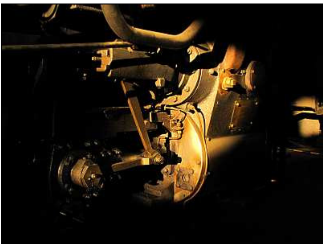
P45 – Where the steam meets the steel ... No.3472 'Elize's' massive rear cylinder cover, combination lever and union link are nicely highlighted.
