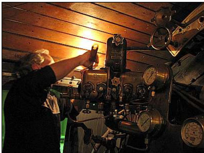
P01 – Temporarily swapping a pair of oil lines to assign a working port (center) to the left cylinder, and an erratic port to the less critical application of the mechanical stoker. A longer small-bore copper oil feed pipe had to be fitted to reach the crossed-over stoker port's outlet.
