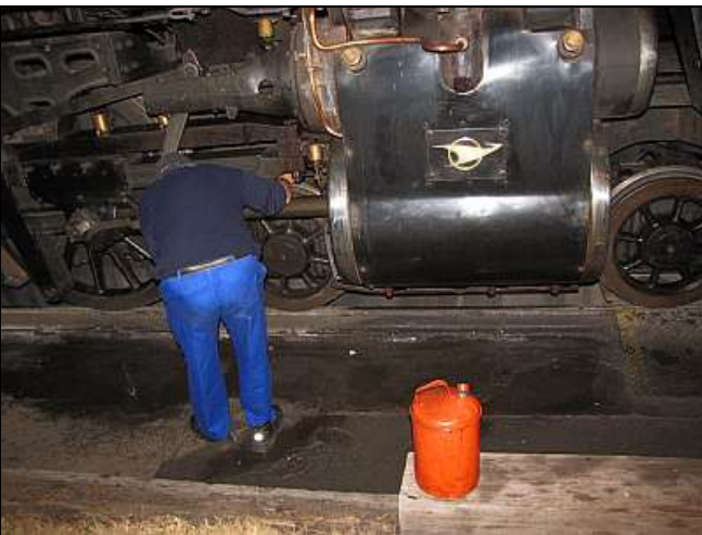
P13 – The flare lamp has either gone out or is missing and Piet is now topping up the bogie axle boxes by feel and instinct in semi-darkness. Luckily, the 15F's bogie wheels are spoked and allow for easy access to their axle boxes.
