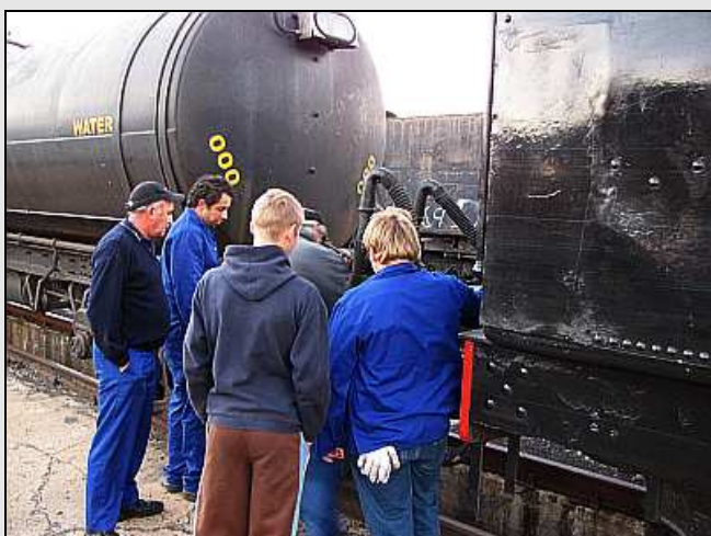
P31 – If it doesn't leak, it's not a steam engine : whether it's oil, hot or cold water, steam, vacuum, sand, amps or air. The fellows are wrestling with the tanker's water coupling. The rubber sealing rings are less resilient in the winter chill.
