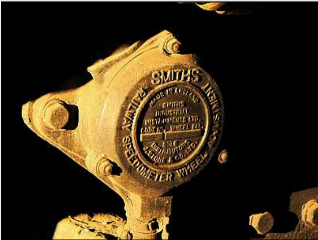
P47 – The terminal head for the pulsed speedometer. These are universal across the later SAR locomotives with the speedo sets being calibrated for the wheel diameters.
