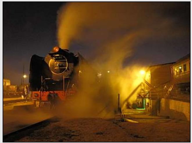
P14 – Fireman Bob-Tail Matthee steams out the stage with the mechanical stoker's exhaust as it just starts to pick up its crunchy load. Fire cleaning was very simple with only a relatively thin layer of soft, fluffy ash to scrape out.
