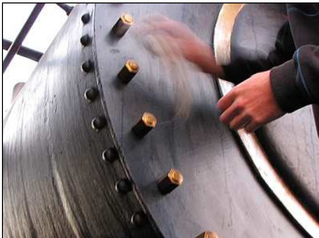
P29 – Brass nuts for Hott-Nutts. Slowly but surely, the non-ferrous décor is slowly re-appearing on the locomotives. Attie's nose wheel is back up as well. But the plain black etching primer is permanent – no graphite paint!
