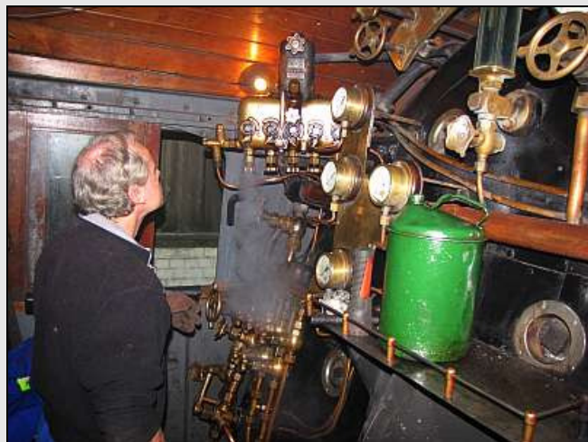
P02 – Andrew does a test blow-down of the now-stoker sight glass. There is a blockage somewhere, which cannot be repaired in time on a live loco. As the pipe work no longer had a non-return valve, Andreas needed to switch the stoker steam off before safely working on the lubricator.
