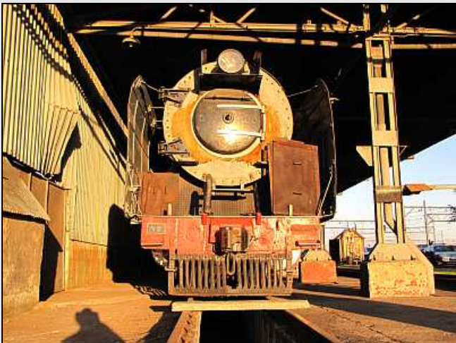
P43 – Recently shunted to the old boiler-washout area for security, Friend of the Rail's 25NC No.3404 'Elsabe' lifts her rusty face to the sun. On the buffer beam are stacked the spark arrestors (right) and the baffle plates (left).
