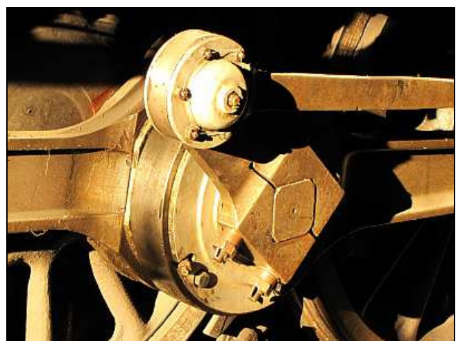
P52 – Details of the roller bearinged return crank – including the usually-unnoticed thrust plate between the two housings. Contrary to popular belief, these bearings DO need greasing on occasion – but not for every run. We top up this housing with pumped white grease once a year.
