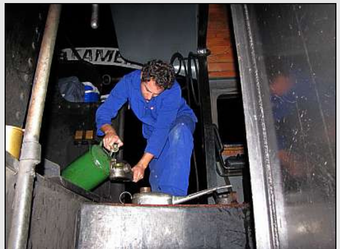
P10 – Recently qualified fireman Andreas Matthee fills up the short-spouted oil feeder to start topping up the Detroit-type lubricator for the day's work. His face is still intact and burn-free, so he listened to the updated stoker instructions.
