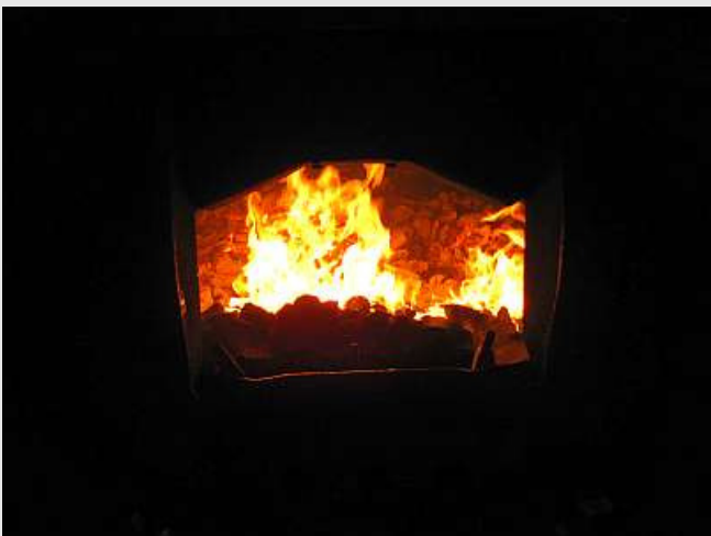
P07 – A sharp truncated, full-width coal bank burns on the leading edge. The central and front firebed stayed aglow untouched for more than 5 hours with the hard high-carbon coal. This class 15F rail-grinder actually LIKES this stuff!
