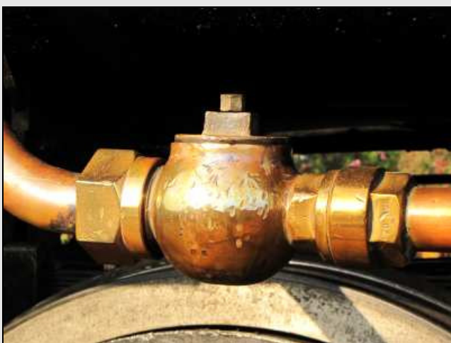
P27 – The non-return valve in the left side boiler delivery pipe. These had been brightly polished by Oom Attie, but were already starting to oxidize with the heat and humidity. Note the decades of hammer n' spanner-blow marks.
