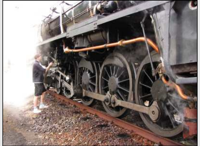
P06 – With steam shrouding the locomotive’s front end, ‘Hott-Nutts’ George is in a world of his own, applying ‘soft grease’ to the expansion link trunnion bearing.
