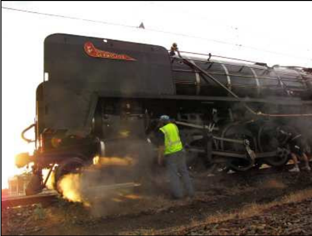
P05 – The rising sun is at coupler height. It is always astonishing to see how much fresh air and ‘through-gaps’ there actually are in a locomotive’s frames and motion. Louis is adding MH oil to the two crosshead slide oil pots.
