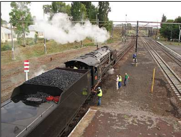
P09 – Johann Beret-bach has re-laid his fire and she’s on the blower, as evidenced by the lifted plume on the stack. Louis is wisely wiping his hands clean at the ‘waste cubby’ before trying to use those handrails with greasy hands.
