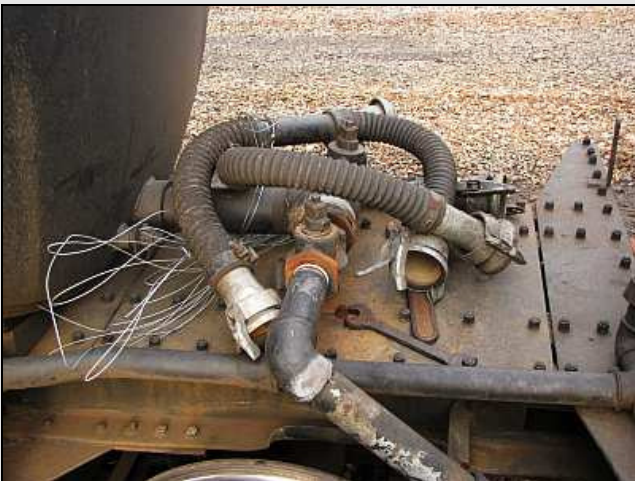
P07 – Just some of the paraphernalia required to keep a long distance bean-boiler going. These are spare water transfer hoses with bell couplings, baling wire to tie down the clamps and spanners to operate the transfer valves...
