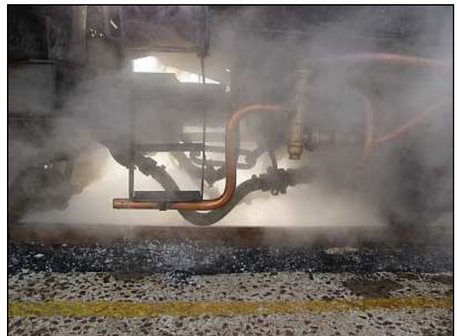
P20 – The loco interlinks. From front to rear, RHS Injector Water Feed, Vacuum Brake Pipe, Safety Chain, Stoker Steam (McCaughlin Coupling) and far back, the LHS injector feed. The draw bar is visible above the pipe work.
