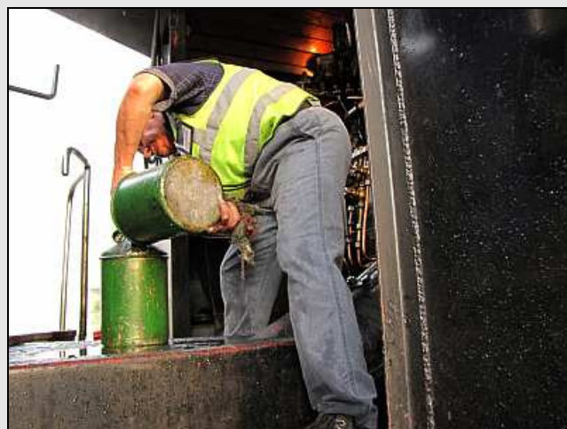
P02 – Normally I at least drain and fill the lubricator, even if I don't have time to blow down the sight glasses and fill the metering chambers with water. But I chickened out this morning, as I didn't know then if it was a fault on the loco or procedural error, which caused the trainee burns yesterday.
