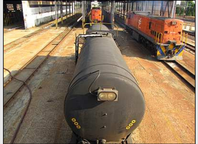
P30 – We do it Garratt-style these days, hauling 1 or 2 31,000 litre water tankers to extend our range. This WAS a Garratt's tank once, hence the fitted lamps. We would use the extra water for the coaches as well as for the loco.
