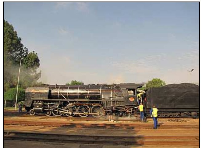
P24 – They are just passing up the water bottles just as Johann starts the second round of fire cleaning to do the rear half of the grate. The 15F's drop grates are in the centerline of the fire and Johan does the front half first.
