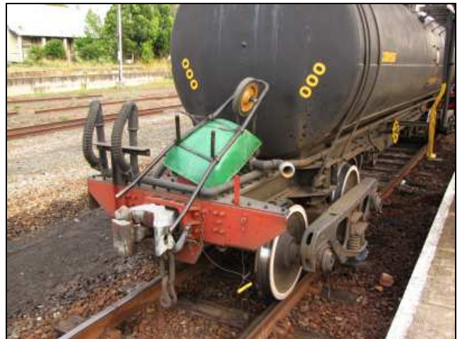
P08 – ... and a barrow quickly stashed at the other end. Naturally, this would NOT be done at the leading end of a vehicle and definitely not within a coupled train. The barrow, of course, is for the shifting of ashes n’ clinkers.
