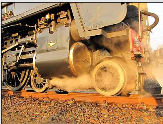
P03 – The warming-up steam chests add atmosphere to a mellow morning as the valves have been set to forward gear to shift the linkages to allow access for lubrication. Nothing like the smell of tallow-n'-steel-scented steam! ☺
