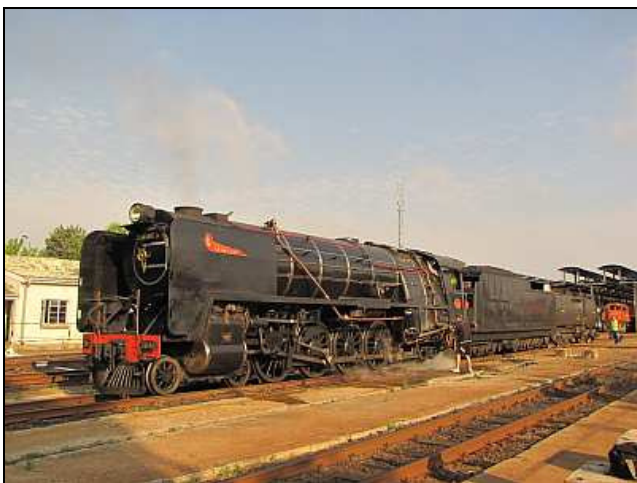
P21 – The fire shovin' is done and George is just 'shunting' the ash pan kibbles now. We had copious quantities of light ash but little clinker. That fire had been burning for over 24 hours, so we actually did quite well!
