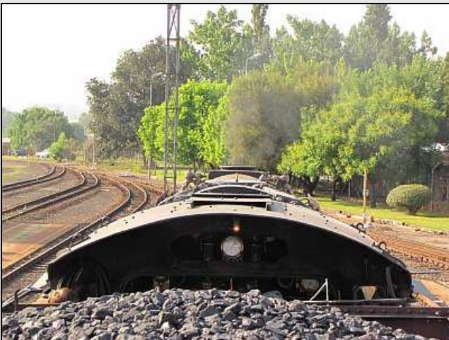
P31 – Servicing is done, the tender tank is almost full and she's about ready to pop with boiler pressure at 1300kPa and climbing. Notice the canopy lamp is still burning and has survived a session of reciprocating fire irons and slices.
