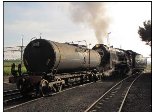
P07 – Shunting the auxiliary water tanker in curiously monochrome light. Andre was driving and didn't couple up TOO hard. ☺ The locomotive's front coupler hadn't centralized and it missed the knuckle, but they got it hooked up on the second attempt.
