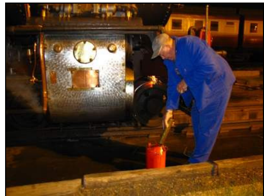
P25 – Keeping railways hours, but only one or twice a week, is a holiday for an old railway man. Frans is sucking MH oil into a syringe to top up the old fashioned bogie axle boxes on our class 12AR 'Susan.'
