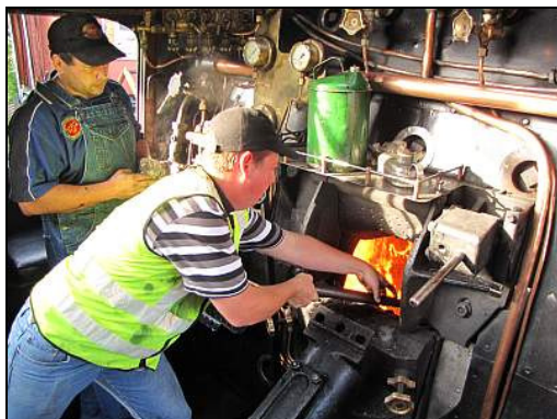
P05 – From generation to generation. The trainee driver gives a trainee fireman (Simon Bennett) some tips on firing right at the back of the wide 15F firebox, through that awkward winged firing portal.
