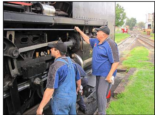
P06 – Checking the valve gear for any missed grease nipples. There is always at least one...
