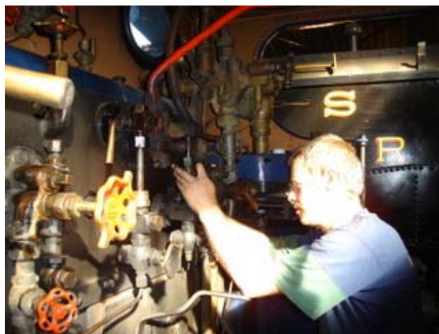
Derrick fitted a new gauge glass rubbers to the gauge columns that were leaking.
