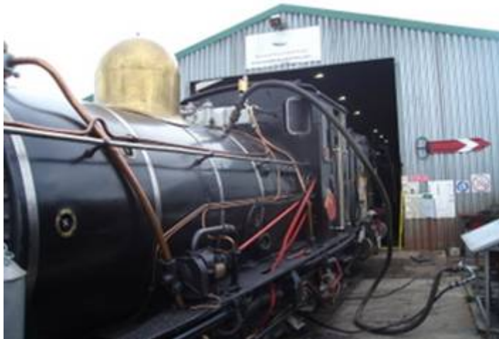
NGG 16 number 153 boiler being filled with the 2 " pipe from the large centrifugal.
