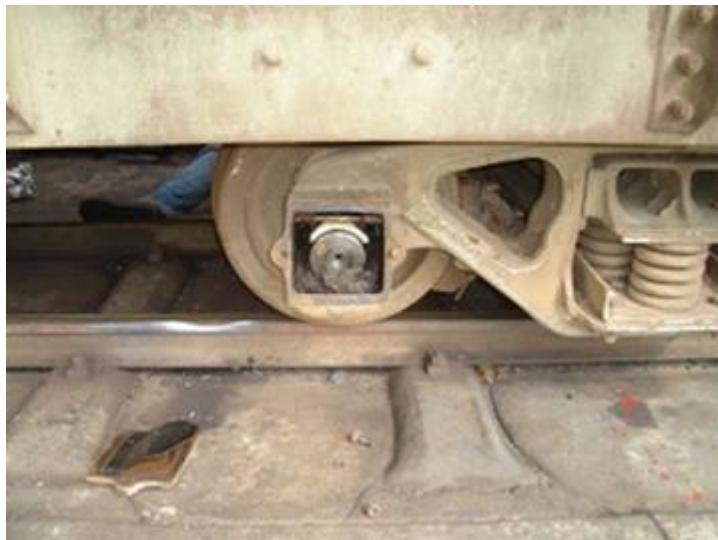
The old axle box wool was removed and new wool soaked with oil was used to pack the boxes again after the bearings were fitted.
