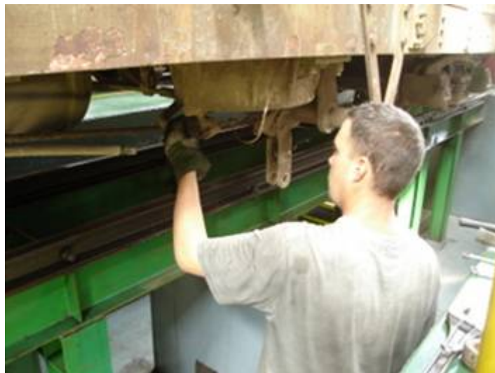
Wouter stripping the vacuum cylinder release valve to fit a new one.
