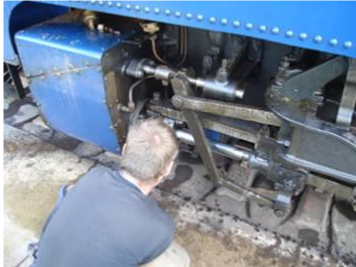
Derrick busy removing the piston gland to repair the leak.
