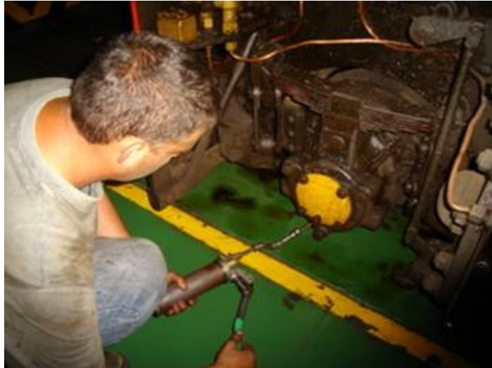
Wouter greased all the roller bearings with white bearing grease.
