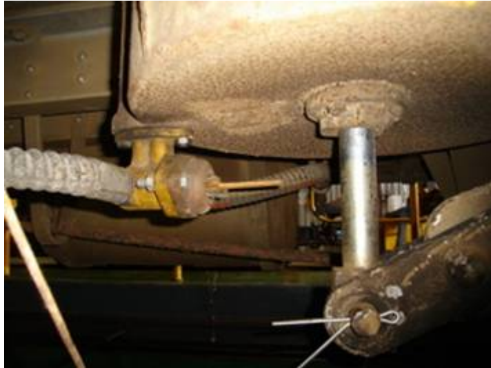
A new overhauled release valve and good second hand piston rod was fitted.
