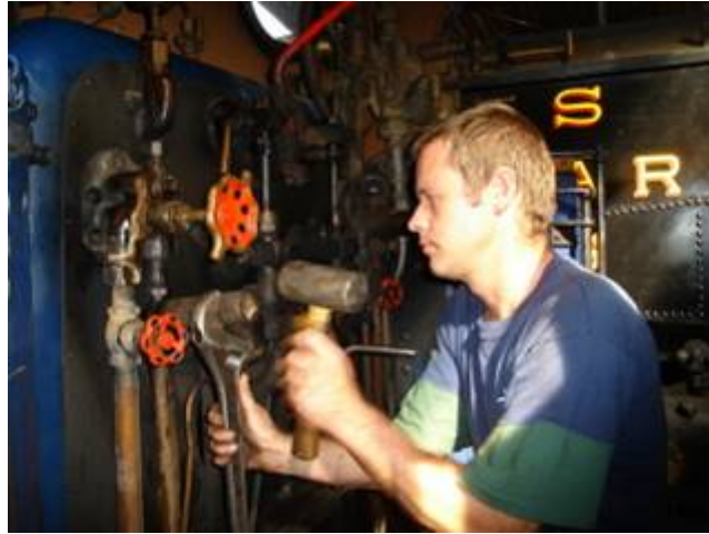
The left side non return valve was also opened and inspected
