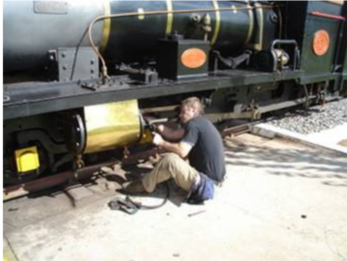
Packing the valve and piston glands on the new lawley number 97.
