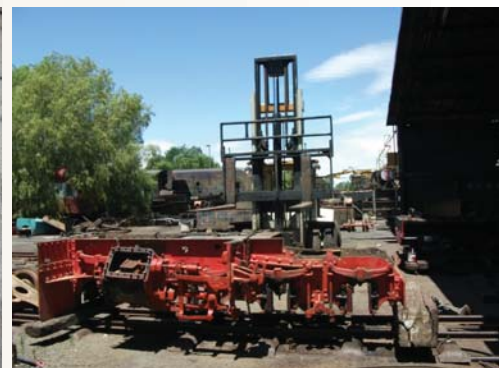
The wheels were removed from the number one end frame. Both wheels and frames are in a bad condition mainly due to rust and some derailment damage caused many years ago. Photograph by Lucas Nel.
