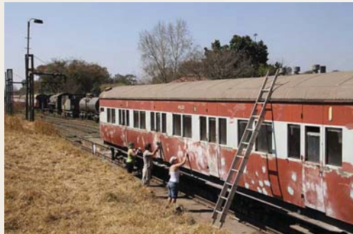
Coach being prepared for painting at CP Photograph courtesy of Chris Janisch
