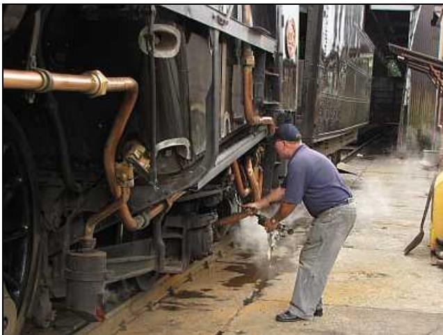
EJ01 – Grease up.
