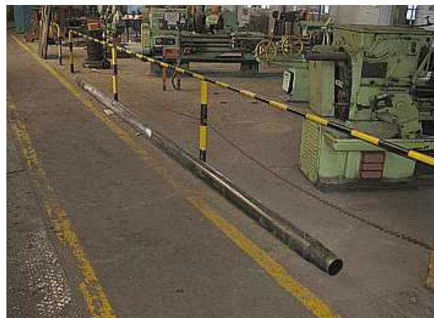
Here is a flue tube 2056 needs 29 of them
