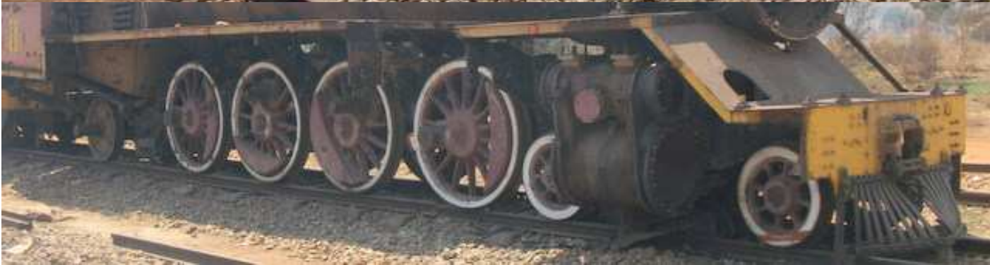
Below: Tender springs were removed, axle boxes destroyed.
