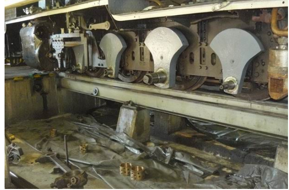
The dismantled driving gear awaiting the brass bushes.
