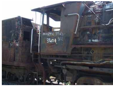
Class 25NC Number 3409 Wheels in a bad condition otherwise not to bad, some boiler mounts available
