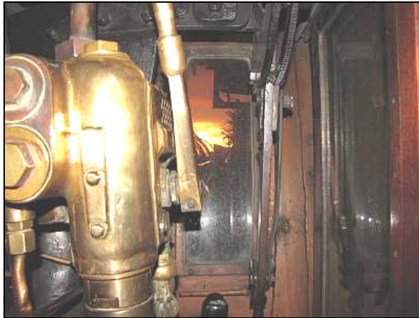
P17 – The ember light as seen through the driver's window. Our 'Lil' Susie' is the only Reefsteamers locomotive driven with the right hand on the regulator, the steam locomotive's equivalent of a 'throttle pedal.' (Hanging down in the corner.) The brass contraption to the left is the vacuum brake ejector.
