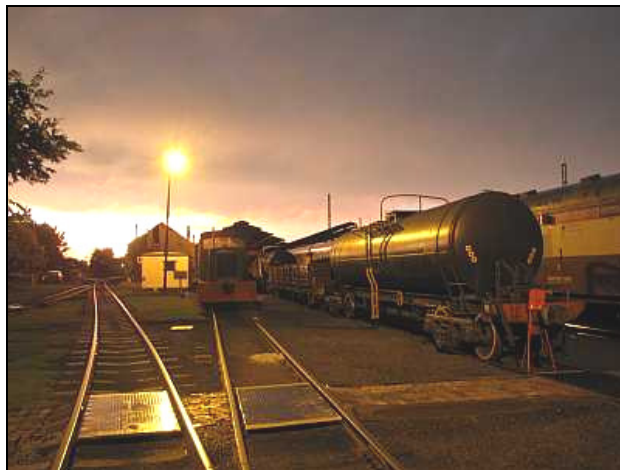
P19 – I'm standing on the crossover points with the 'tea tree' just peeking in from the left. There has been some tight shunting going on. Road number 2 is jam packed with rolling stock and you can see there was barely enough room to put the C&W marker between the tanker and the pedestrian walkway. The signal-red coloured marker indicates that a train is not to be moved, usually because it under repair or inspection. It is analogous to the blue flags and lights used by American railroads.
