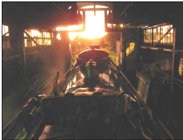
P18 – Rooftop view. The nature of the boiler fittings such as the single, centrally mounted turret manifold, the taller steam dome and the proudly standing safety valves shows this loco was built well within the loading gauge. It looks as if the blower is on, but the smoke is merely streaming via a long exposure.
